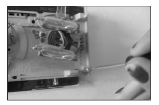
Install the new temperature sensing device in the same location as the old one. Gently pull the labeled wires through the base of the new device. Do not damage the wires or remove the wire labels.
