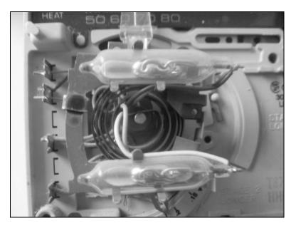
Attach each of the old wires to the corresponding terminals of the new device. As you attach the wires, remove the wire's label. If necessary, strip the wire ends. Replace the cover.
