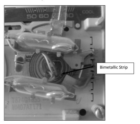
Below are pictures of a temperature sensing coil in a hot water bath device.
