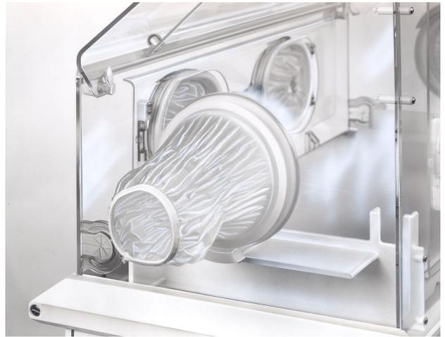
12. Fold the sleeve back, and slip the elastic band over the outer ring of the port housing.
