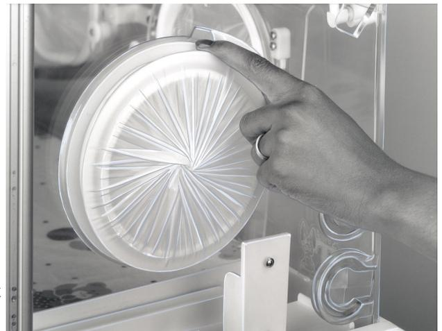
13. Install a tubing access grommet into the front edge of each side of the hood. If a tubing access grommet is distorted or torn, replace it.
