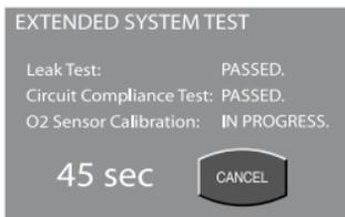
All tests are performed simultaneously. The maximum time for the EST is 90 seconds. To restart the EST at any time, select the Cancel button to return to the Setup screen.
