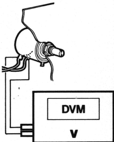
When exchanging any of the potentiometers on the front panel, use the table below for adjustments.
