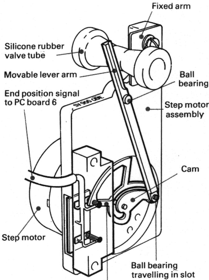
Screen on cam breaks light between lamp and photo detector
