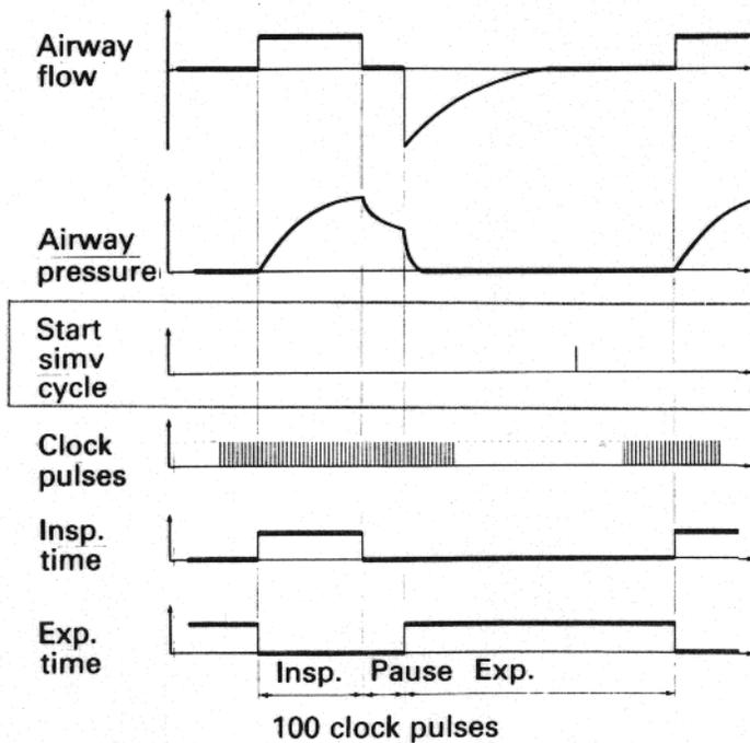
The intervals are controlled by a clock pulse generator.
