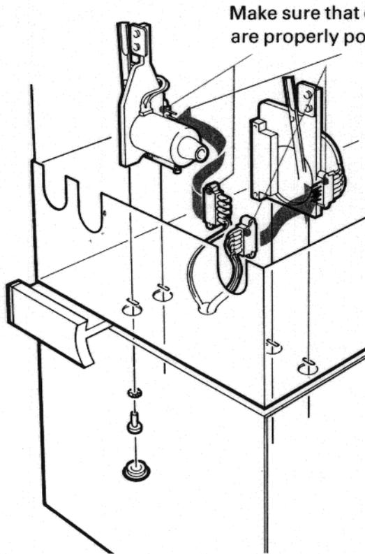
Make sure that connectors are properly positioned
