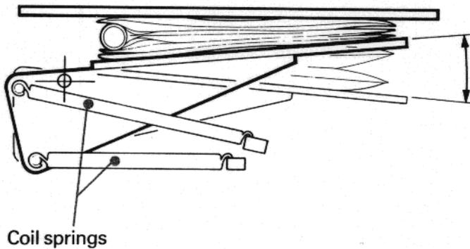
A double coil spring set is arranged to give a constant pressure to the bellows, independent of the plate position. The pressure is set by the adjustment handle **PRESET WORKING PRESSURE**.
