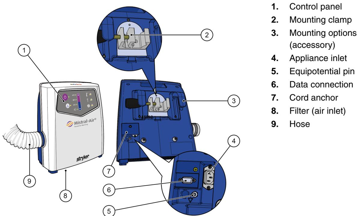
The device can be controlled by using the control panel at the front top of the device. The back of the device is equipped with a universal mounting clamp, a sealed data connector, an appliance inlet and an equipotential pin. It can be expanded with a mounting accessory set as shown in the image above to offer various mounting options, see *Accessories and disposables* on page 20.
