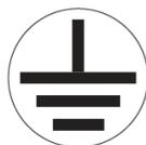
Connect the device to an earthed socket only. Risk of electrical shock exists if the equipment is not connected to a properly grounded receptacle.
