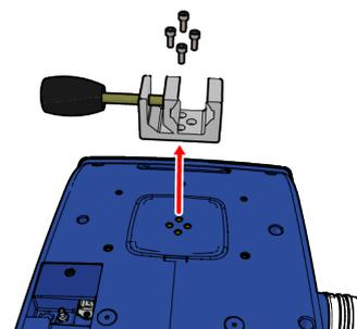
4. Attach the Cover at the 3 indicated locations using the first 3 of the 5 M4x16 3 mm hexagon screws with a maximum torque of  $1.5 \pm 0.2$  Nm or  $13.3 \pm 1.3$  in-lb.
