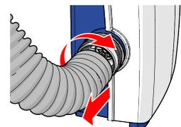
5. Attach a new hose by rotating the hose anti-clockwise.
