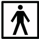
Type BF applied parts (according to IEC 60601-1:2005+A1:2012)
