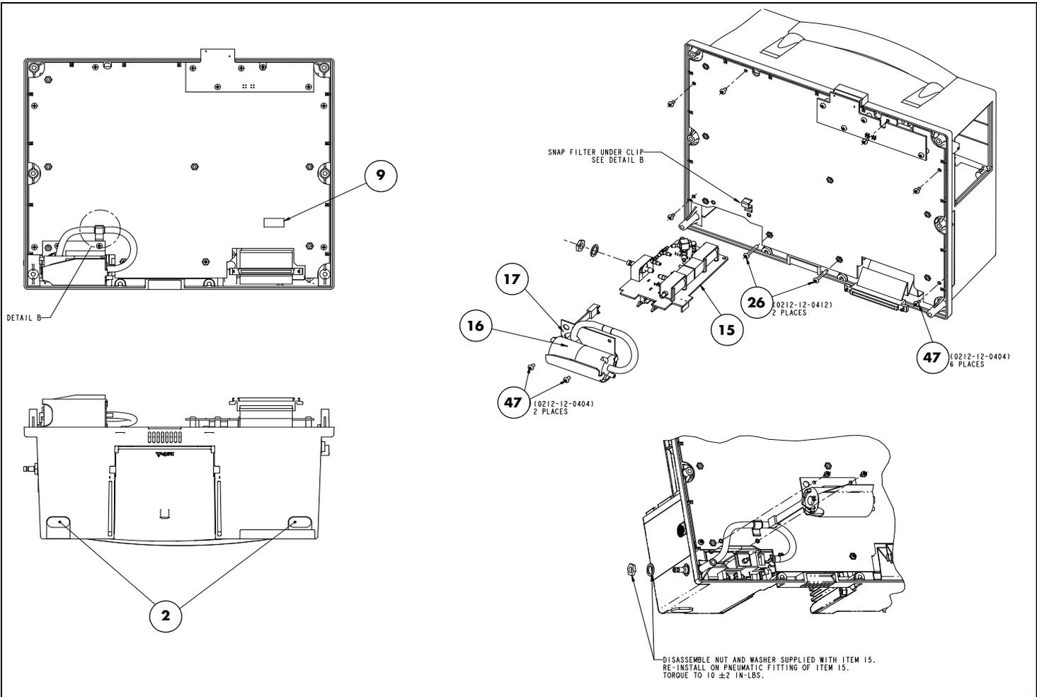
**FIGURE 3-11** Rear Housing Assembly
