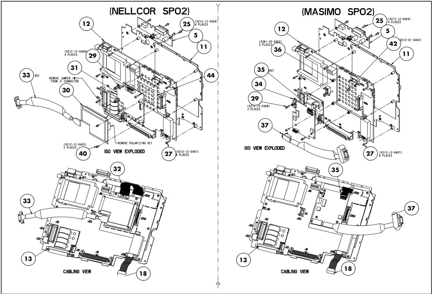
**FIGURE 3-7** Rear Housing Assembly (For use with Spectrum P/N 0998-00-1000-XXXXX only)
