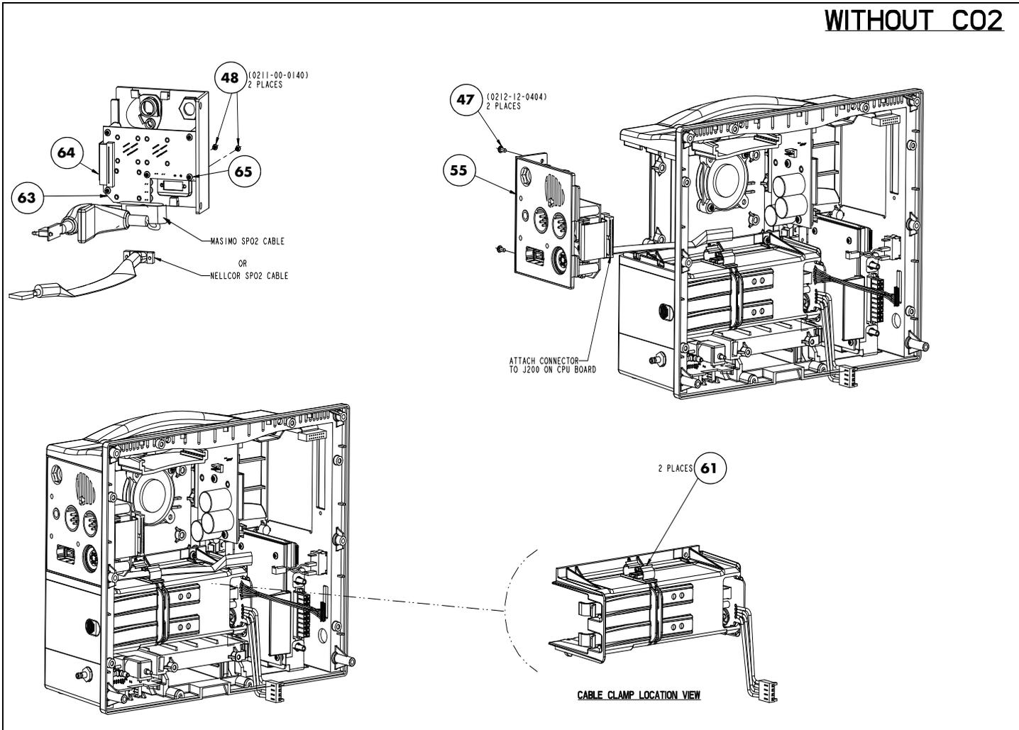
**FIGURE 3-16** Rear Housing Assembly (Sealed Lead Acid battery configuration)
