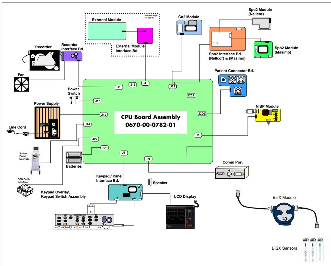
**FIGURE 2-2** Spectrum OR™ Block Diagram
