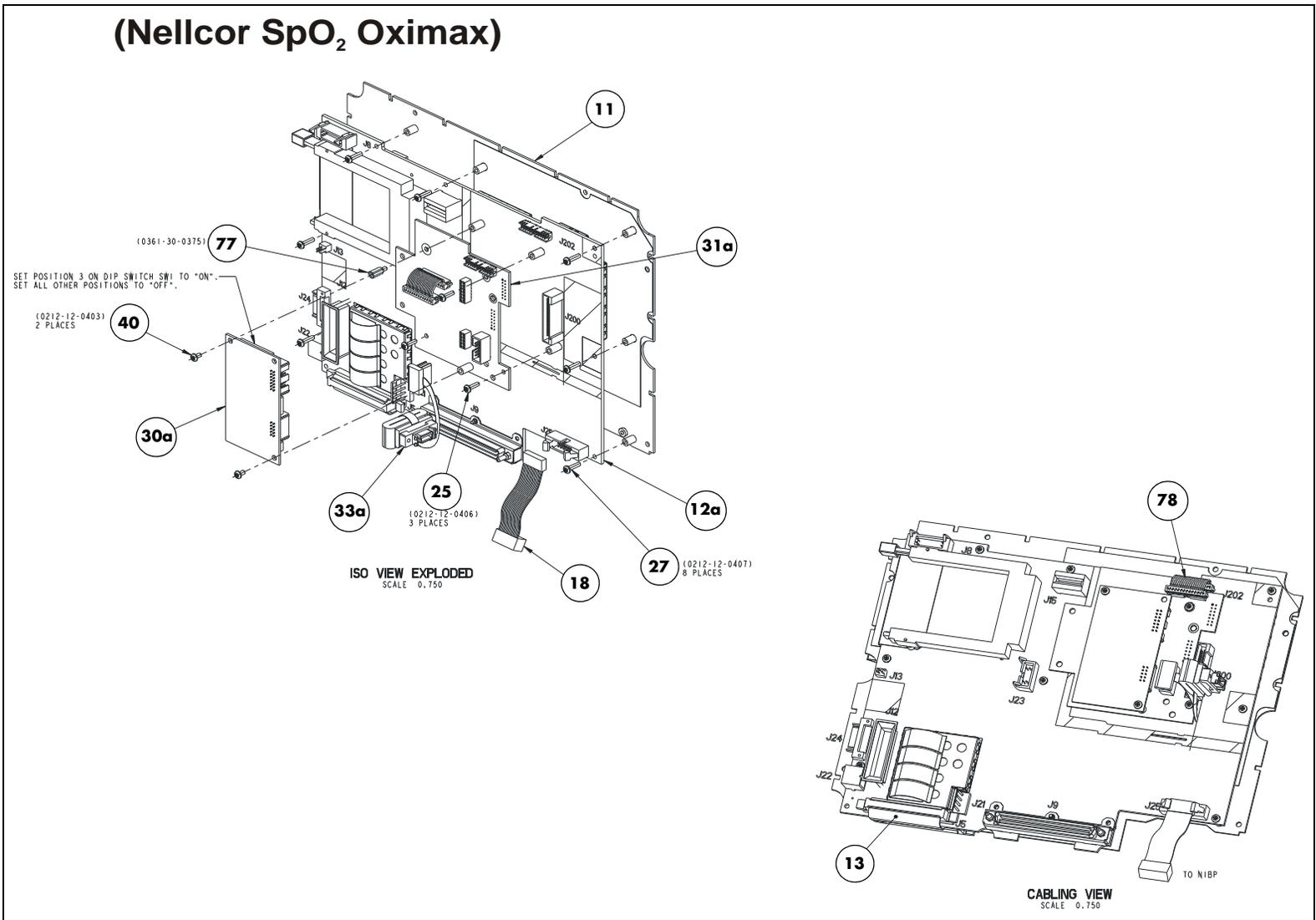
**FIGURE 3-10** Rear Housing Assembly
