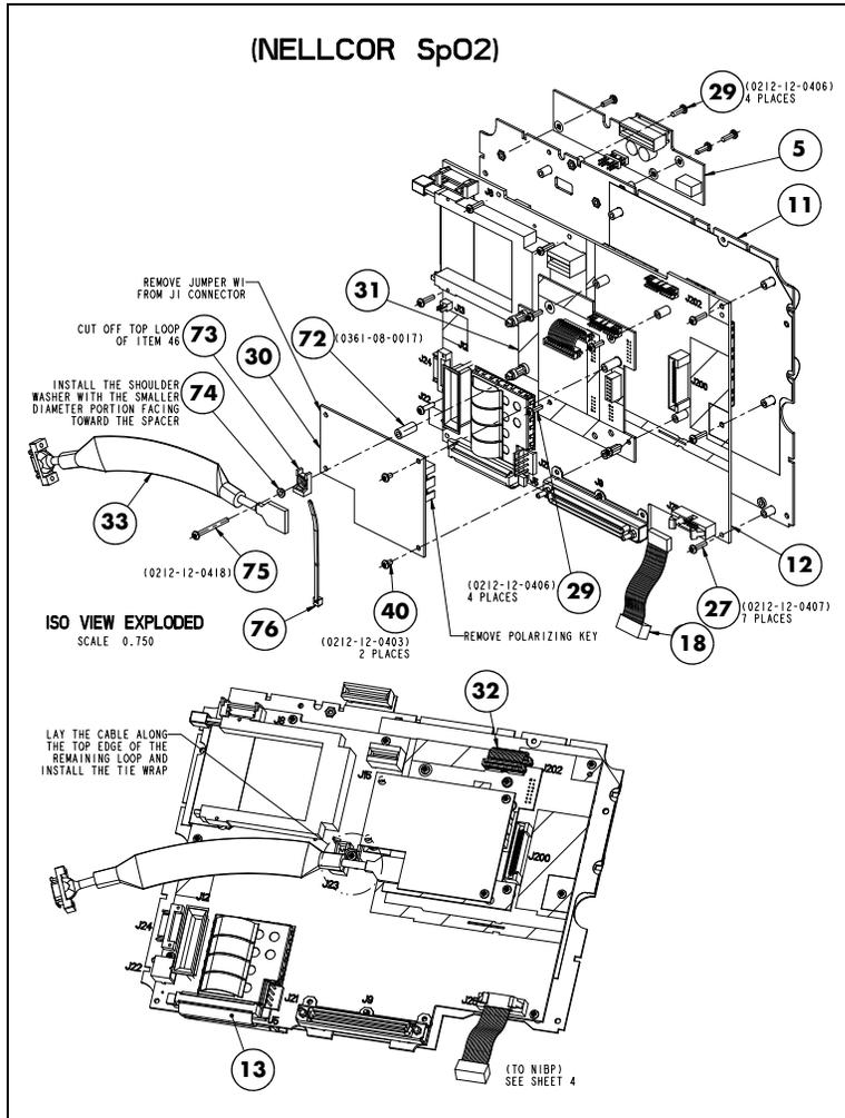
**FIGURE 3-8** Rear Housing Assembly
