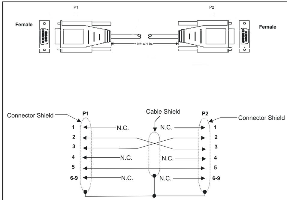
**FIGURE 1-4** Serial Port to Serial Port Cable (P/N 0012-00-1275-01)
