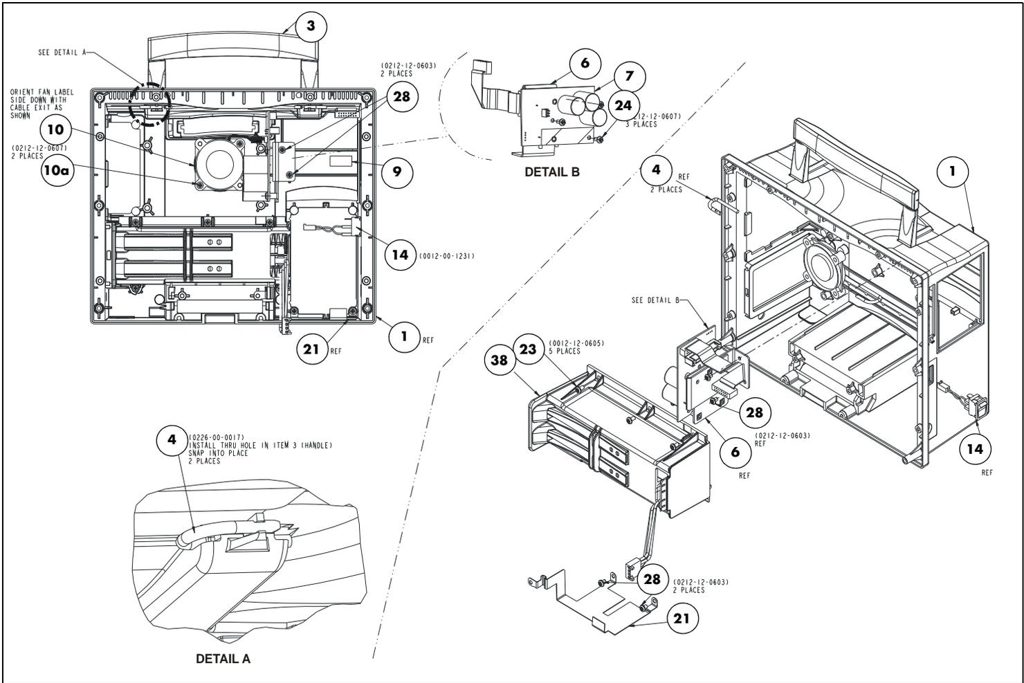
**FIGURE 3-5** Rear Housing Assembly (Sealed Lead Acid battery configuration)
