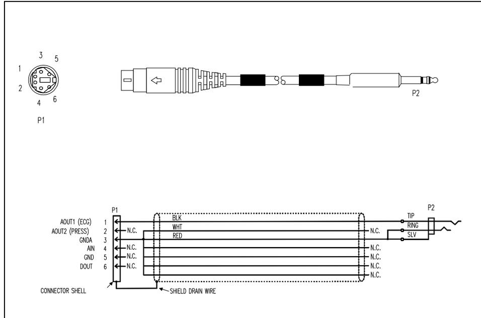
**FIGURE 1-14** IABP Cable (ECG Only) (P/N 0012-00-1459-01)
