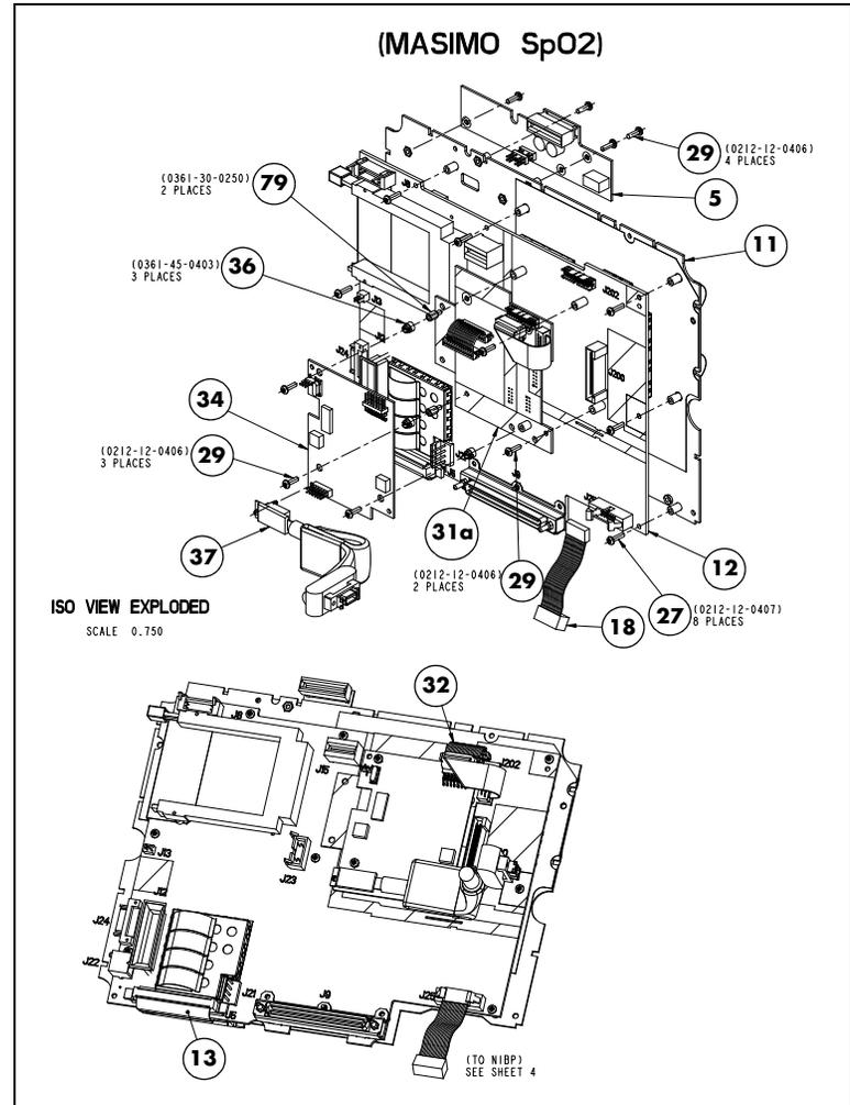
**FIGURE 3-9** Rear Housing Assembly
