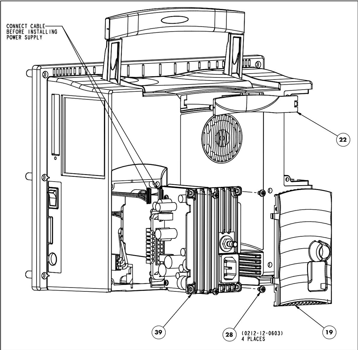
**FIGURE 3-13** Rear Housing Assembly (Lithium-Ion battery configuration)
