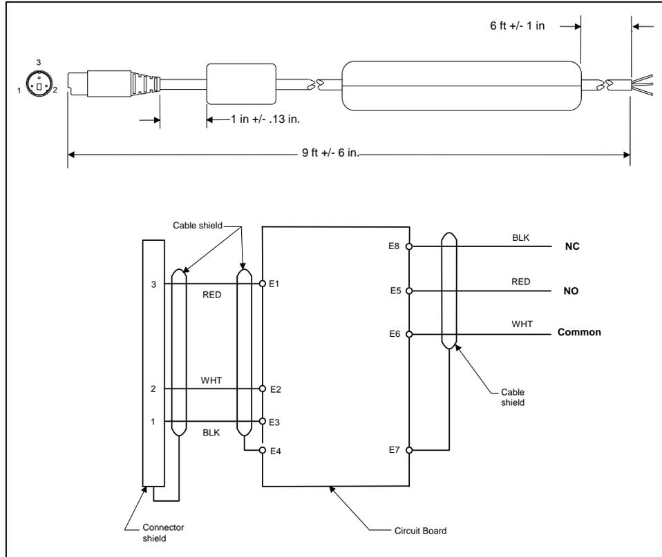
**FIGURE 1-1** Nurse Call Cable (3 Pin Circular to Unterminated)
