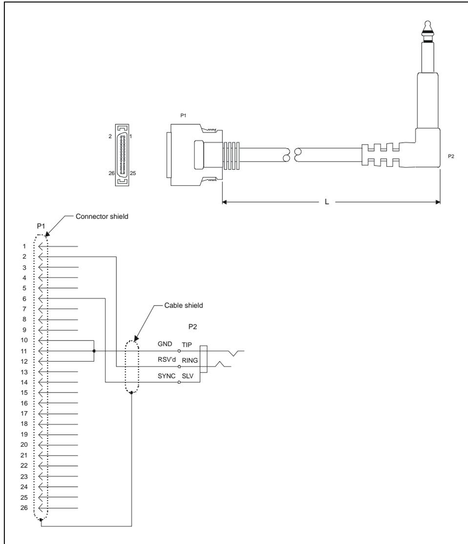
**FIGURE 1-5** 26 pin Molex to Mini Phone Plug (DPD Sync Cable)
