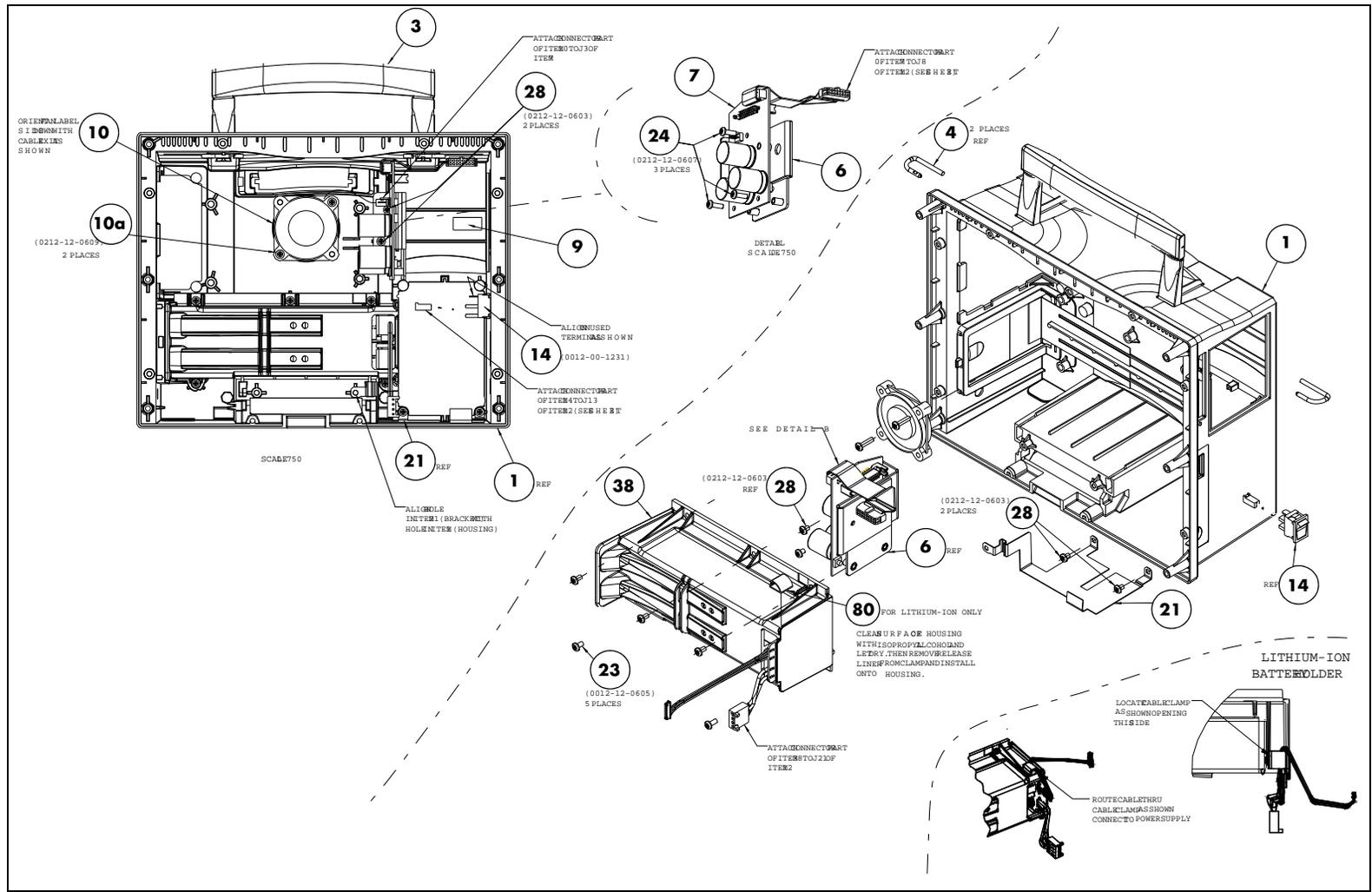
**FIGURE 3-6** Rear Housing Assembly (Lithium-Ion battery configuration)
