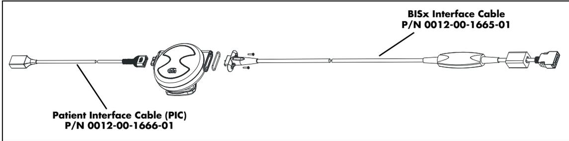
**FIGURE 1-17** BISx Module (Front View)
