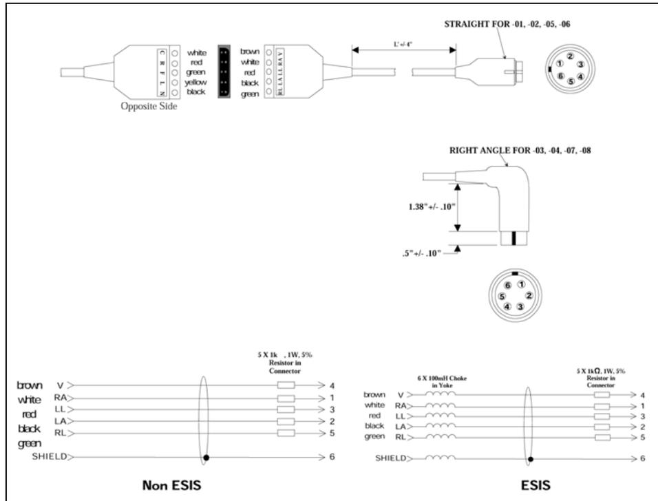
FIGURE 1-9 ECG Cable ESIS and Non ESIS
