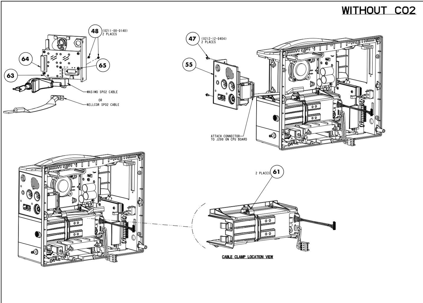
**FIGURE 3-18** Rear Housing Assembly (Lithium-Ion battery configuration)
