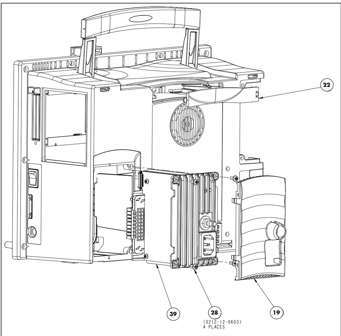
**FIGURE 3-12** Rear Housing Assembly (Sealed Lead Acid battery configuration)
