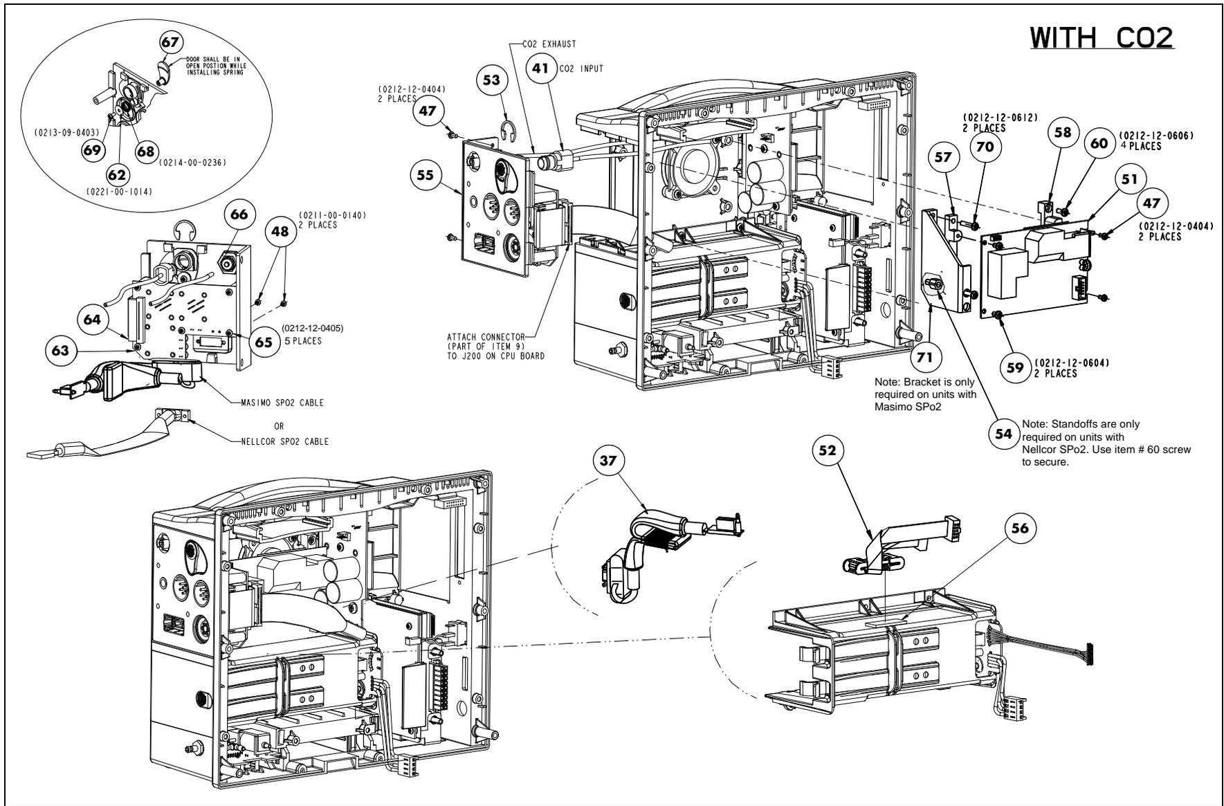
**FIGURE 3-17** Rear Housing Assembly (Lithium-Ion battery configuration)
