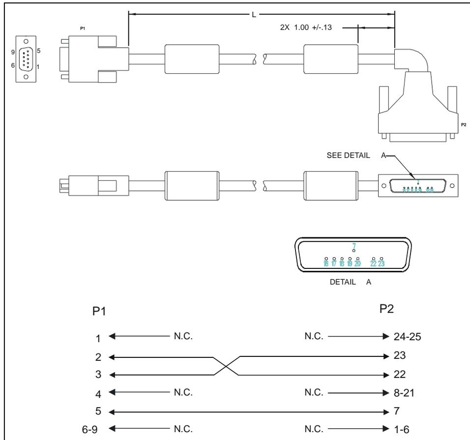
**FIGURE 1-3** Serial Port to Gas Module II/SE/SE with Spirometry Cable (P/N 0012-00-1276-XX)
