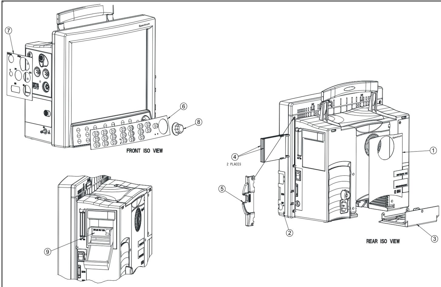
**FIGURE 3-1** Top Level Assembly
