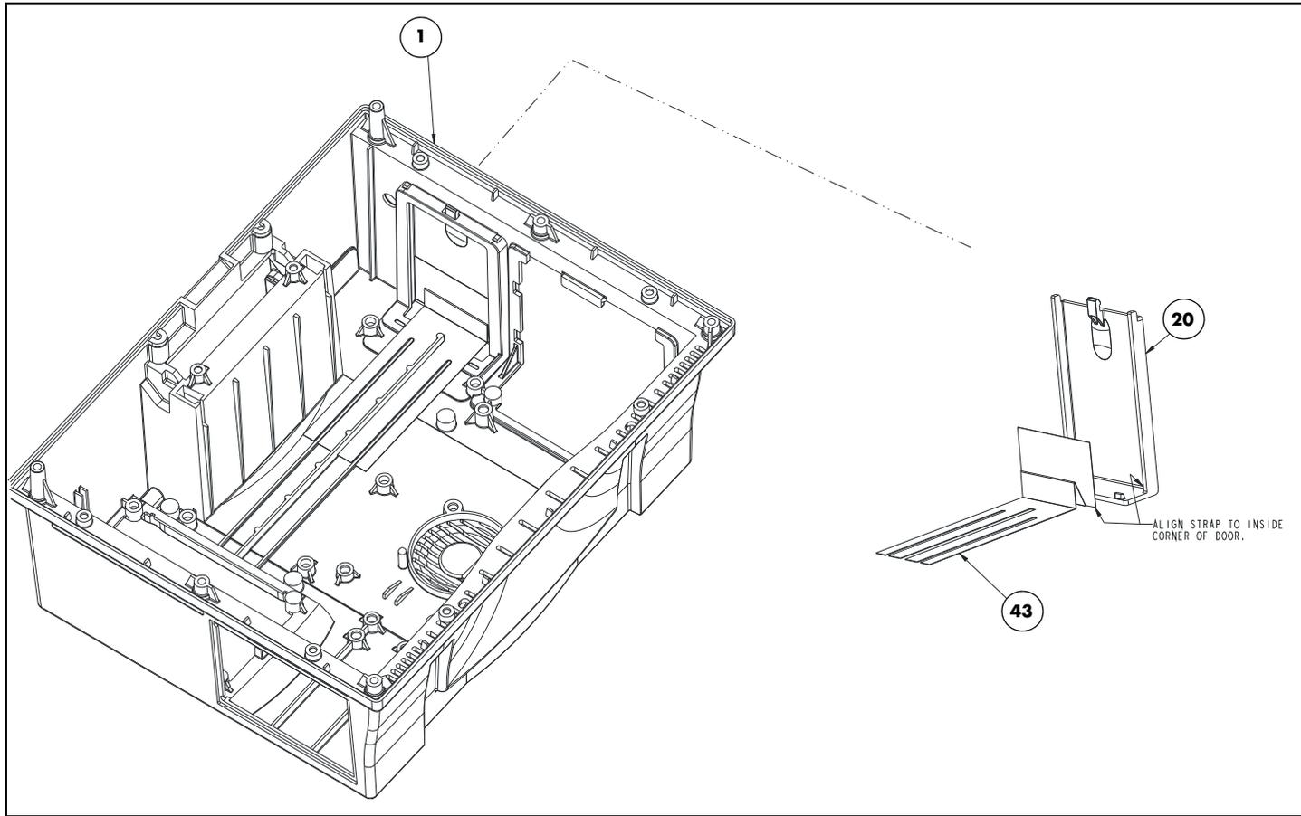
**FIGURE 3-4** Rear Housing Assembly
