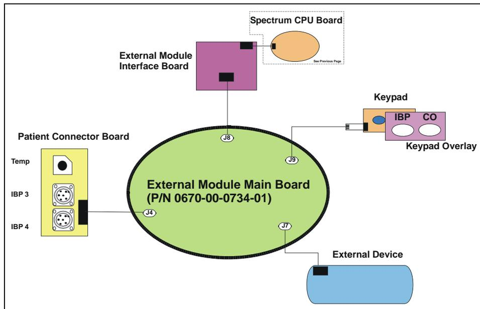
**FIGURE 2-3** Block Diagram (External Parameter Module Main Board)
