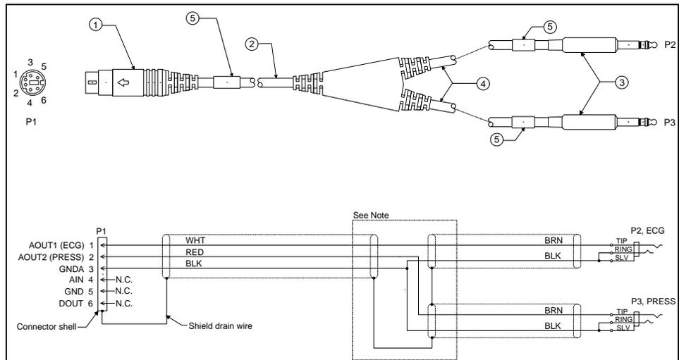
**FIGURE 1-15** IABP Cable (ECG/IBP) (P/N 0012-00-1650-01)
