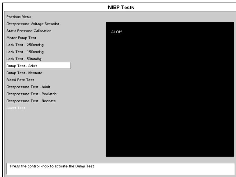
**FIGURE 4-14** Dump Test
