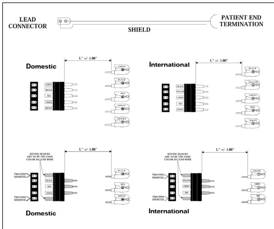
FIGURE 1-6 ECG Shielded Lead Wires
