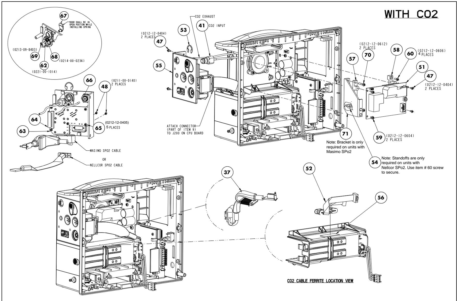
**FIGURE 3-15** Rear Housing Assembly (Sealed Lead Acid battery configuration)
