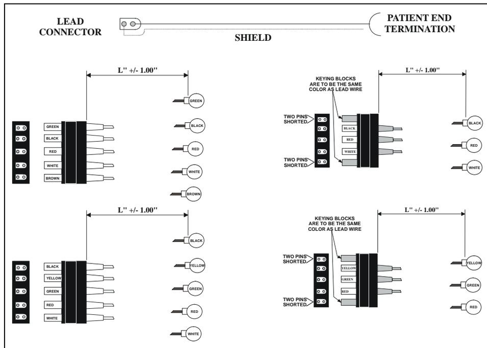
**FIGURE 1-7** ECG Shielded Lead Wires
