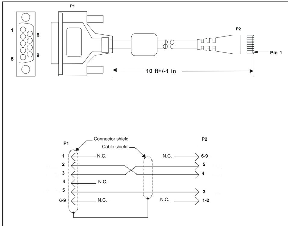
**FIGURE 1-16** Serial Port to RJ 45 Cable (VISA)
