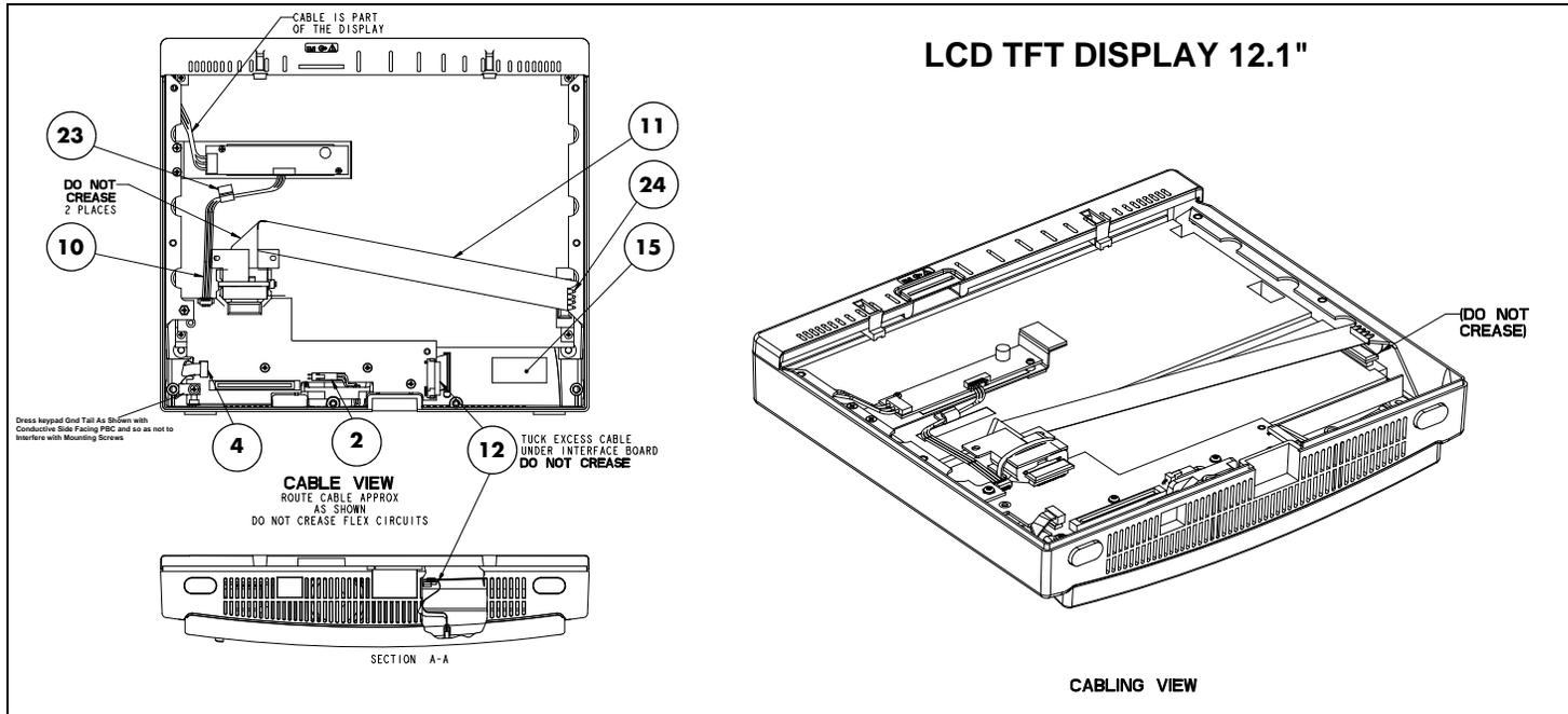
**FIGURE 3-3** Front Housing Assembly
