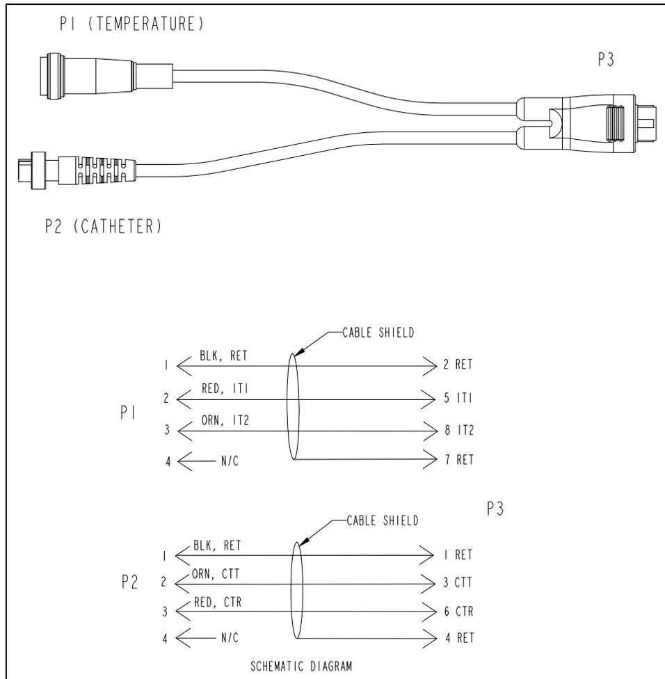
**FIGURE 1-13** Cardiac Output Cable (P/N 0012-00-1447-01)
