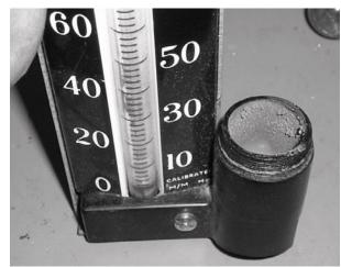
In this photo, the cover for the mercury reservoir has been removed (right). The mercury has oxidized leaving a fine powder that should be removed before refilling the reservoir.
