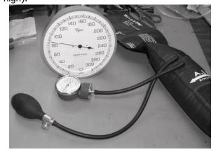
If the pressure is consistently too high or too low, you will need to adjust the zero by removing or adding mercury or twisting the manometer face (if aneroid). Electronic blood pressure devices will have a zero setting which should never need to be adjusted, if the device is properly zeroed before each use. There is a gain setting for electronic devices that occasionally needs to be adjusted.
