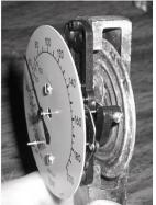
An aneroid manometer uses a calibrated dial. Notice that when the dial is at zero, there is a small rectangle where the needle should rest. This manometer is also calibrated in inches of water.
