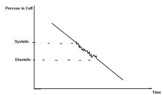
Automatic non-invasive blood pressure (NIBP) machines typically measure the presence of small oscillations in the pressure to determine the systolic and diastolic pressures. Some older machines may use a sensor to detect the Korotkoff sounds.
