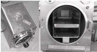
Most hospitals have electric, steam autoclaves, but you will also find an autoclave like the "All American" distributed by UNICEF. It uses an open fire as its source of heat.
