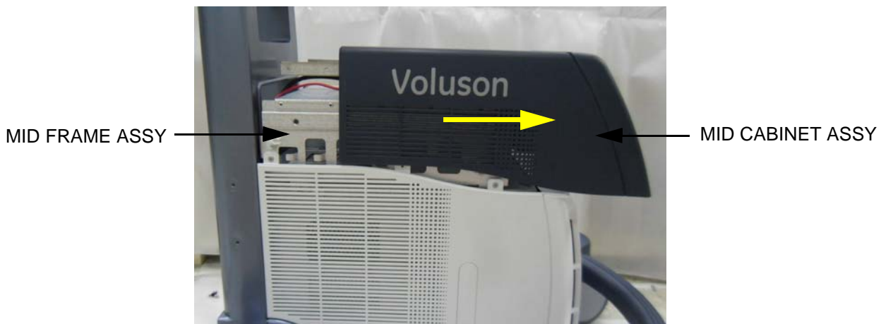
Figure 8-145 Moving forward the MID CABINET ASSY following Slide Rail
