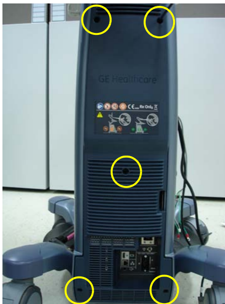
Figure 8-183 Unscrewing 5 screws and removing the REAR COVER POLARIS ASSY
