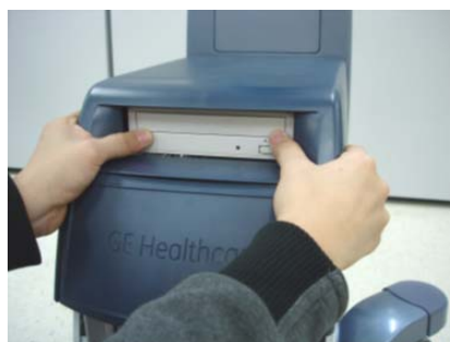
Figure 8-235 Pulling out the MID/HIGH CABINET ASSY BT16
