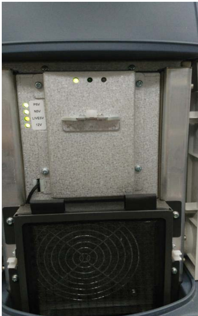
Figure 7-6 Checking green LED inside DPS
