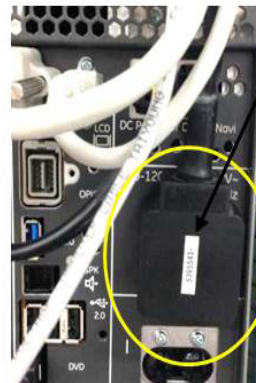
Figure 8-152 Connecting the BW PRINTER CABLE
