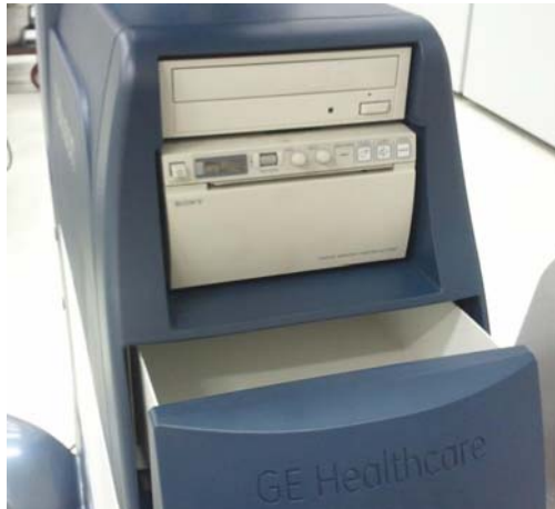
Figure 8-209 The DRAWER Assembly for the HIGH CABINET Option
