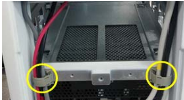
Figure 8-50 Untying the 2 cable clamps
