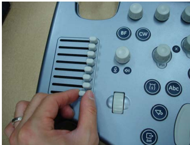
Figure 8-82 Removing 8 TGC KNOBS
