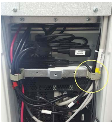
Figure 8-229 Untying cable clamp to unroute WIRELESS LAN cable
