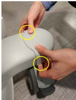
Figure 8-90 Removing the CASTER CAP
