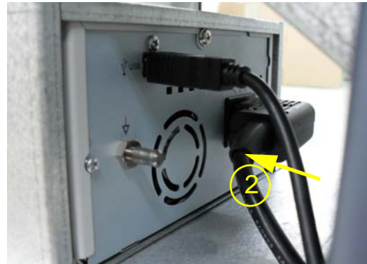
Figure 8-151 Connecting BM PRINTER CABLE
