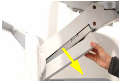
Figure 8-264 Pulling out the ELEVATION ARM LOWER COVER LCF from the ELEVATION ARM ASSY
