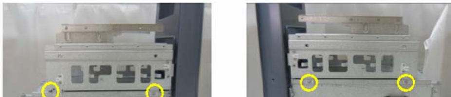
Figure 8-251 Unscrewing 4 screws to remove the MID FRAME POLARIS
