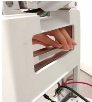
Figure 8-258 Removing the HIGH FRAME GROUND BRKT
