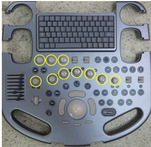
Figure 8-77 Pulling 10 encoder key caps out
