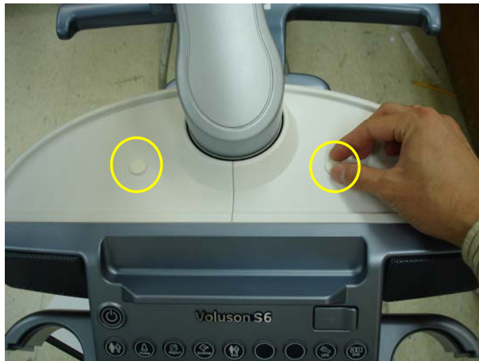
Figure 8-33 Removing the RUBBER CAPS
