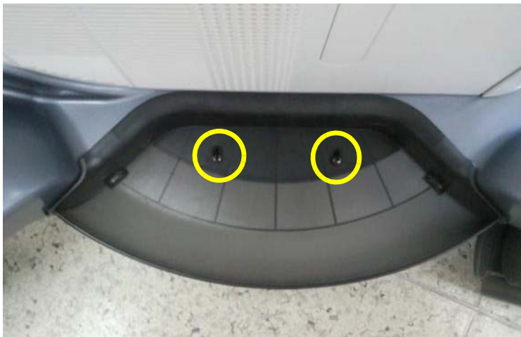
Figure 8-97 Unscrewing 2 screws and remove the SIDE TRAY ASSY
