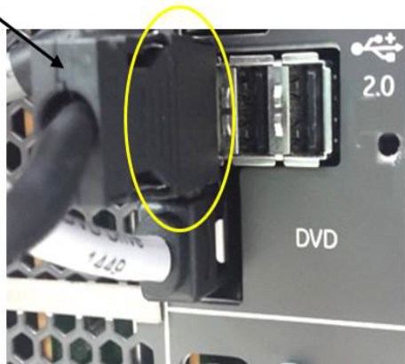
Figure 8-152 Connecting the BW PRINTER CABLE
