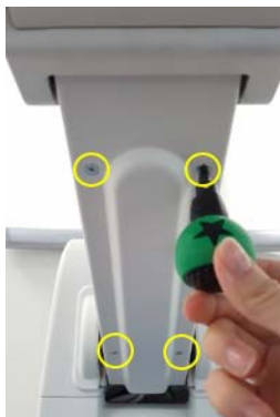
Figure 8-263 Unscrewing 4 screws to disassemble the ELEVATION ARM LOWER COVER LCF
