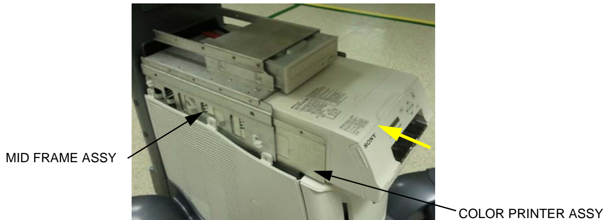
Figure 8-163 Inserting COLOR PRINTER ASSY to MID FRAME ASSY
