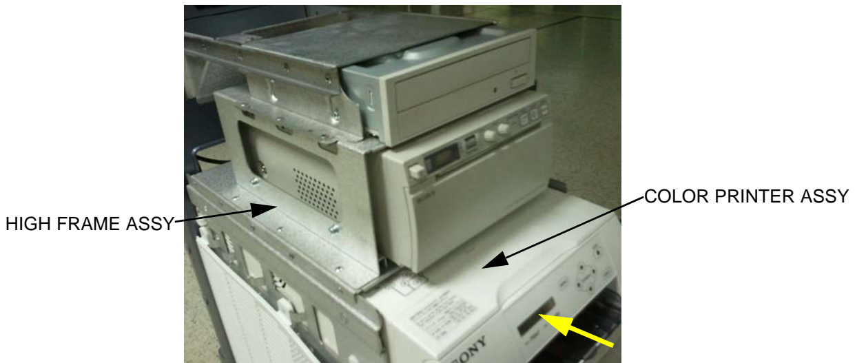
Figure 8-169 Inserting COLOR PRINTER ASSY to HIGH FRAME ASSY
