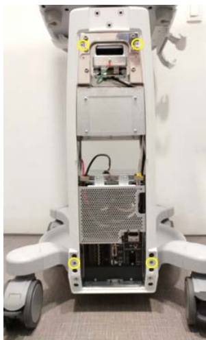
Figure 8-246 Unscrewing 4 screws to remove the BACKBONE REAR COVER LCF
