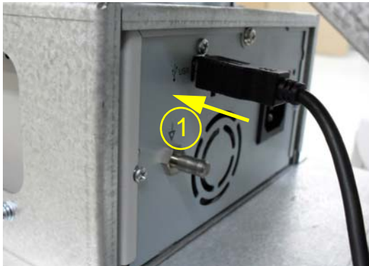
Figure 8-151 Connecting BM PRINTER CABLE
