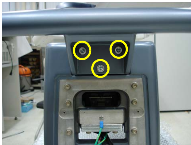
Figure 8-100 Unscrewing 3 screws and remove the REAR HANDLE
