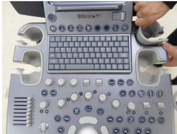
Figure 8-63 Removing the PROBE HOLDER
