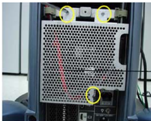
Figure 8-49 Disconnecting CABLE COVER BRACKET
