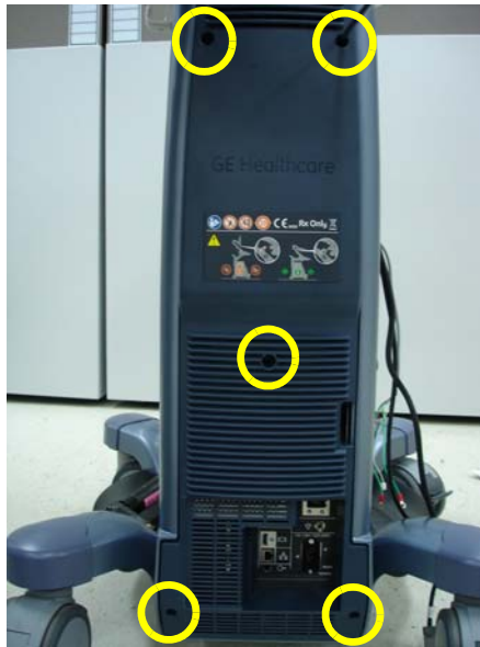
Figure 8-99 Unscrewing 5 screws and remove the REAR COVER ASSY
