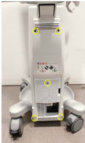
Figure 8-244 Unscrewing 5 screws to remove the REAR COVER BT16
