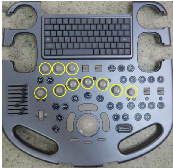
Figure 8-73 Pulling 10 encoder key caps out
