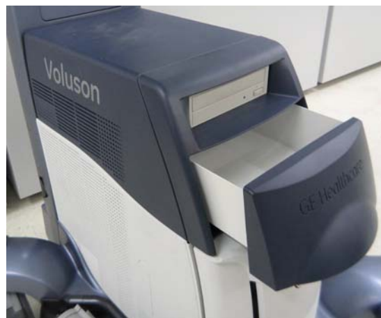
Figure 8-208 The DRAWER Assembly for the MID CABINET Option
