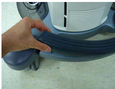
Figure 8-96 Removing FOOTREST COVER
