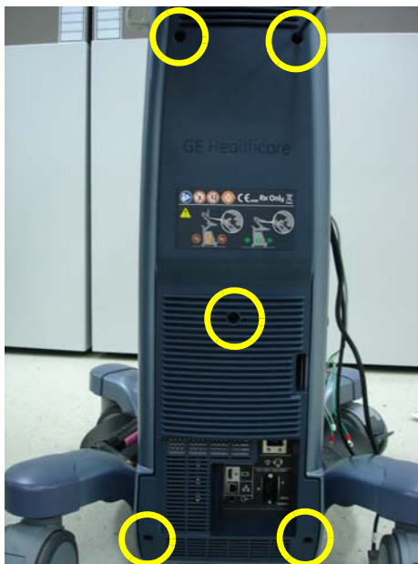
Figure 8-149 Unscrewing 5 screws and remove the REAR COVER ASSY
