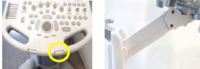
Figure 8-200 Lifting the ELEVATION ARM ASSY to the highest position
