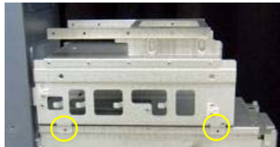
Figure 8-182 Unscrewing 4 screws and removing the MID FRAME ASSY
