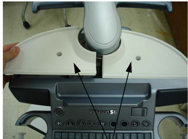
Figure 8-35 Removing the OPIO COVER L,R
