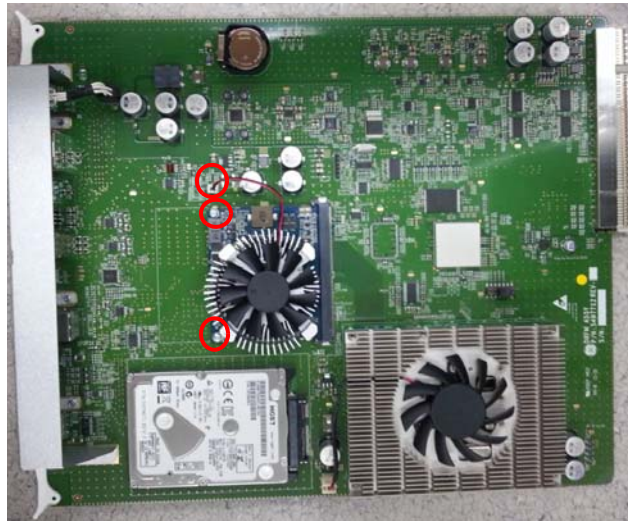
Figure 8-225 Screw point and FAN Connector
