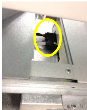
Figure 8-250 Disconnecting 2 cables from DVD
