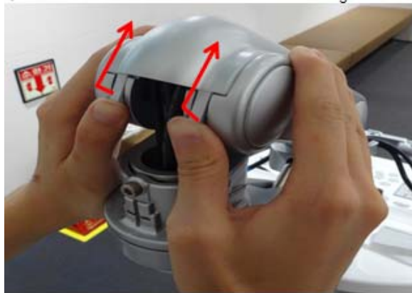
Figure 8-27 Removing 2ND ARM COVER
