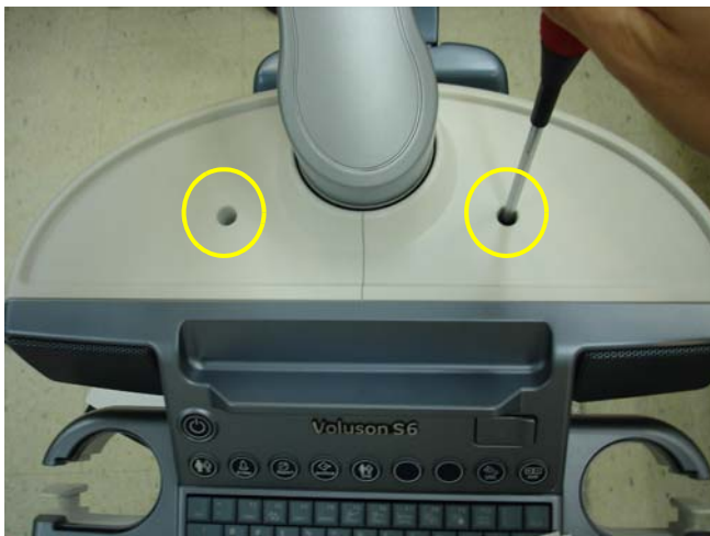
Figure 8-35 Removing the OPIO COVER L,R
