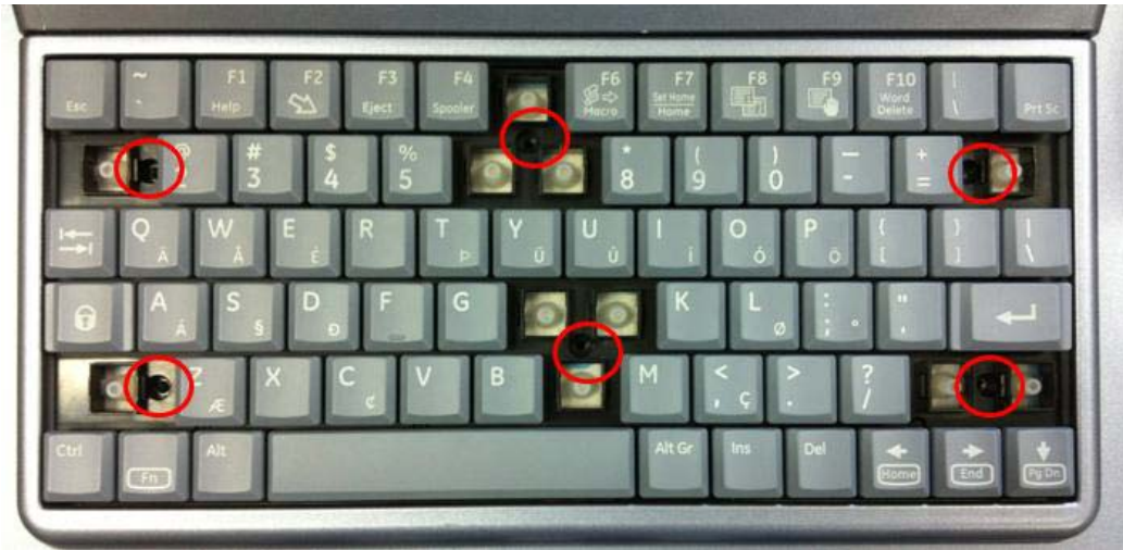
Figure 8-142 Screwing the 6 screws
