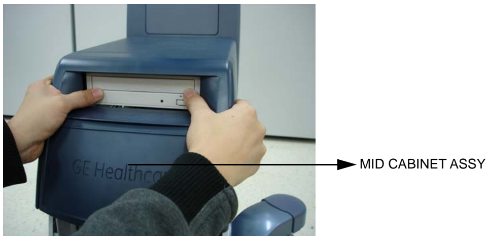
Figure 8-64 Removing the MID CABINET ASSY
