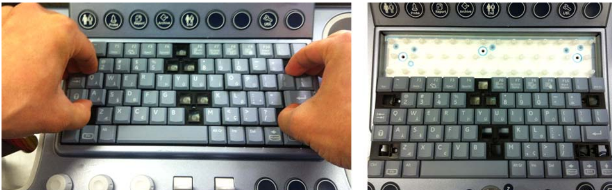
Figure 8-141 Pulling out AN Key Top Assy
