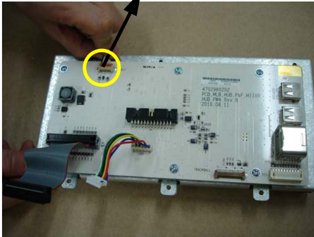
Figure 8-87 Unscrewing 6 screws and pull out the remove the OPIO HUB PWA ASSY
