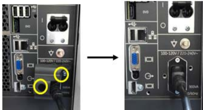
Figure 8-98 Unscrewing 2 screws to remove the POWER CORD FIX BRACKET and disconnect the Cable
