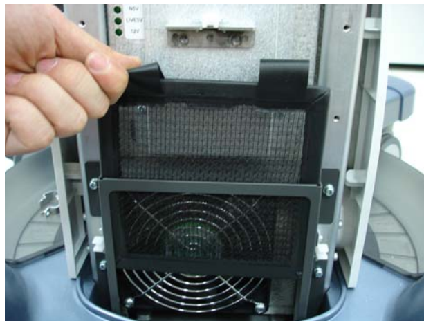
Figure 8-62 Removing the AIR FILTER
