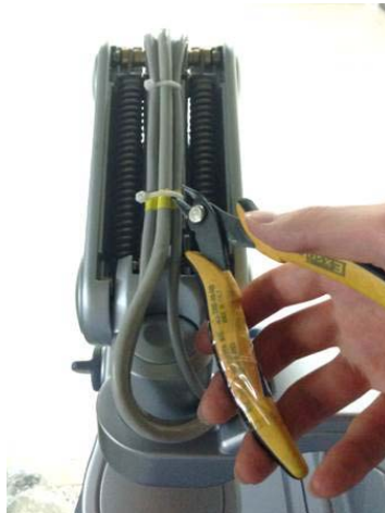
Figure 8-28 Removing the Cable Tie
