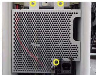
Figure 8-227 Unscrewing 3 screws to remove CABLE COVER BRKT
