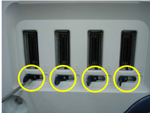
Figure 8-69 Removing the 4 RS KNOBS
