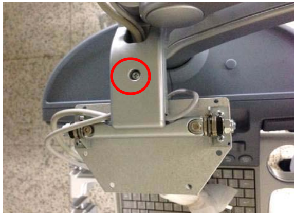
Figure 8-25 Removing the 3RD ARM COVER
