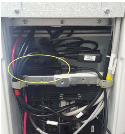
Figure 8-230 Pulling out WIRELESS LAN dongle from loop sheet
