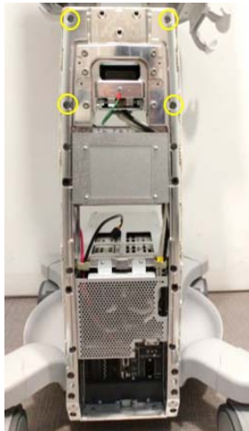
Figure 8-248 Unscrewing 4 screws to remove the BACKBONE FRONT TOP LCF
