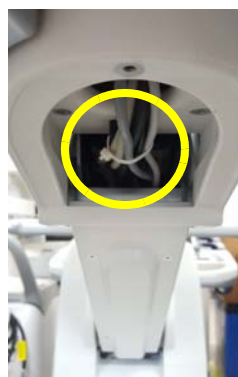
Figure 8-54 Removing the cable tie
