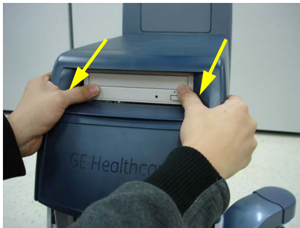
Figure 8-130 Removing the MID CABINET ASSY
