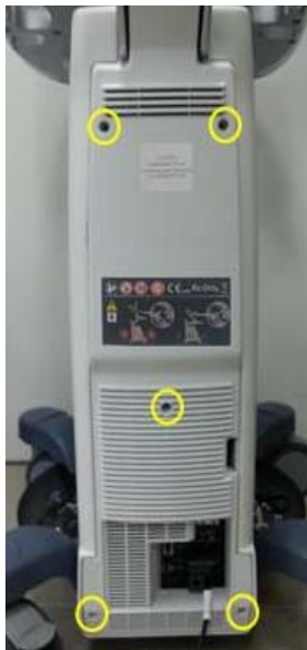
Figure 8-216 Unscrewing 5 screws and removing REAR COVER POLARIS.
