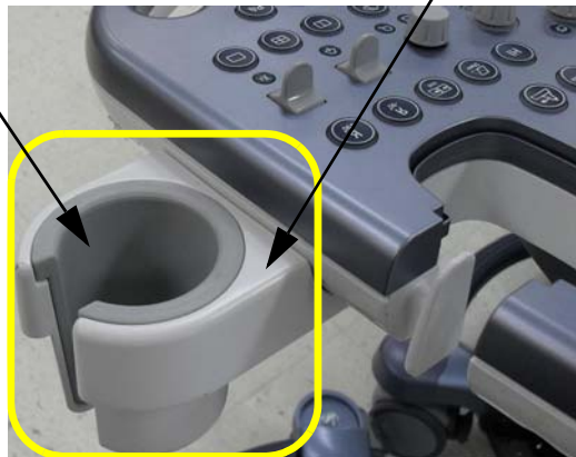
Figure 8-213 Inserting the TV PROBE HOLDER RUBBER to the PROBE HOLDER BASE
