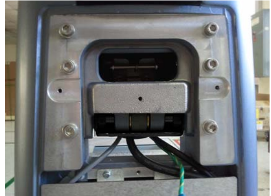
Figure 8-197 The ELEVATION ARM DOWN STOPPER HIGH POLARIS with 2 Hexagonal screws (5405682, HSH M6x30)
