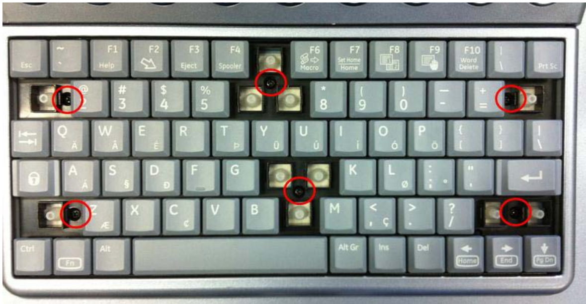
Figure 8-140 Loosening the 6 screws
