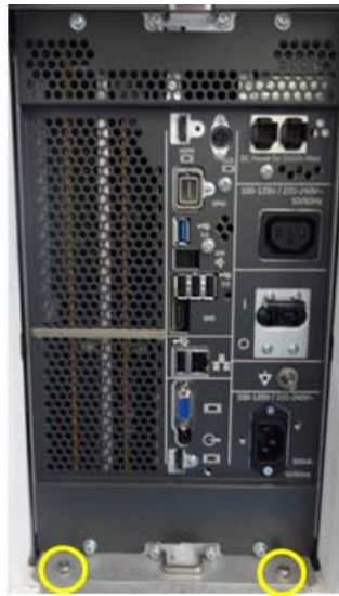
Figure 8-59 Unscrewing 2 hexagonal socket screws
