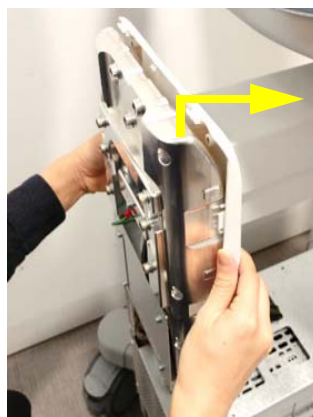
Figure 8-249 Disassembling the BACKBONE FRONT TOP LCF
