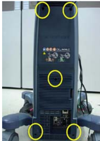
Figure 8-47 Unscrewing 5 screw and remove the REAR COVER
