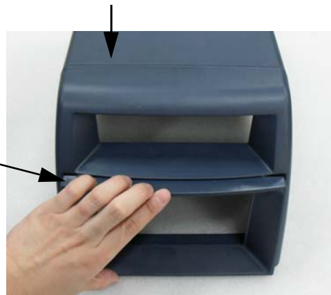
Figure 8-155 Assembling the DUMMY CASE MID BW POLARIS with the MID CABINET ASSY
