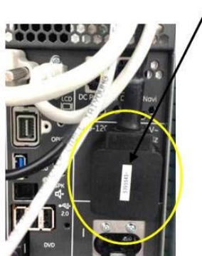
Figure 8-166 Connecting the COLOR PRINTER CABLE into the NEST
