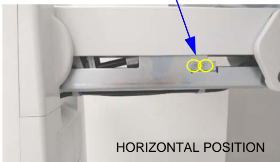
Figure 8-202 Unscrewing 2 screws to remove the ELEVATION ARM STOPPER 12 DEG
