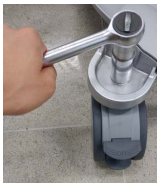
Figure 8-91 Unfastening the NUT
