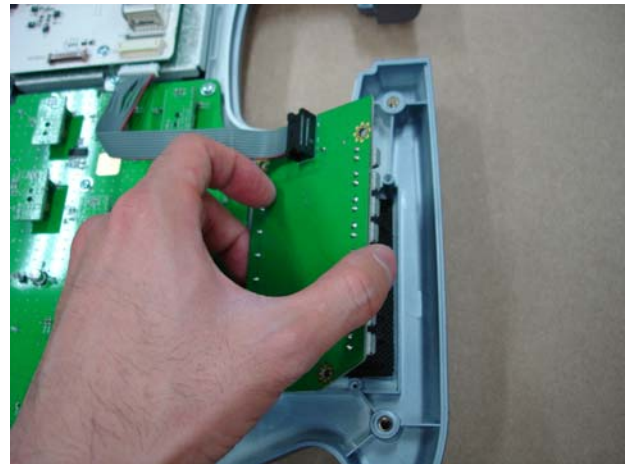
Figure 8-84 Unscrewing 4 screws and pulling out the TGC BOARD
