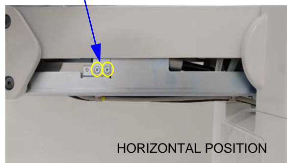
Figure 8-202 Unscrewing 2 screws to remove the ELEVATION ARM STOPPER 12 DEG
