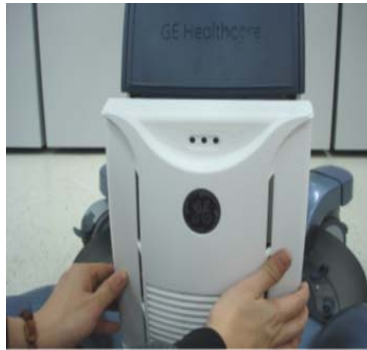
Figure 8-236 Pulling out the FRONT COVER ASSY BT16
