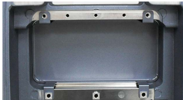
Figure 8-189 Placing the SPEAKER DUMMY BRKT on the HIGH FRAME GROUND BRKT
