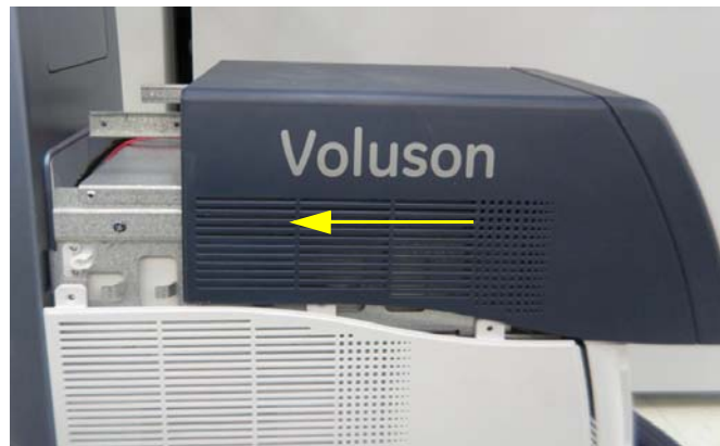
Figure 8-207 Placing the MID CABINET on the MID FRAME and Moving toward the BACKBONE
