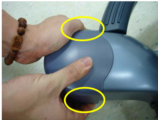
Figure 8-89 Removing the CASTER CAP
