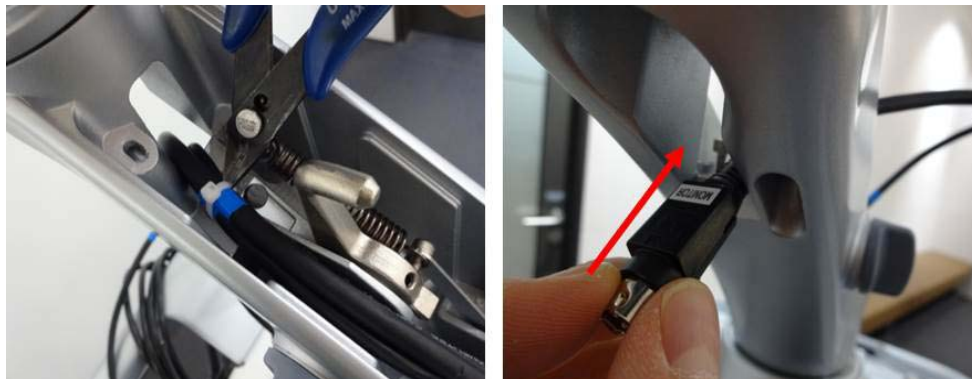
Figure 8-30 Removing Cable Tie and Monitor Cables
