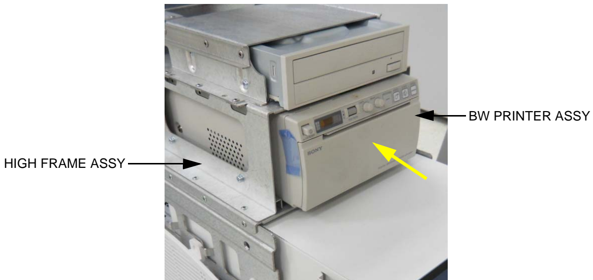
Figure 8-159 Inserting the BW PRINTER ASSY to the HIGH FRAME ASSY
