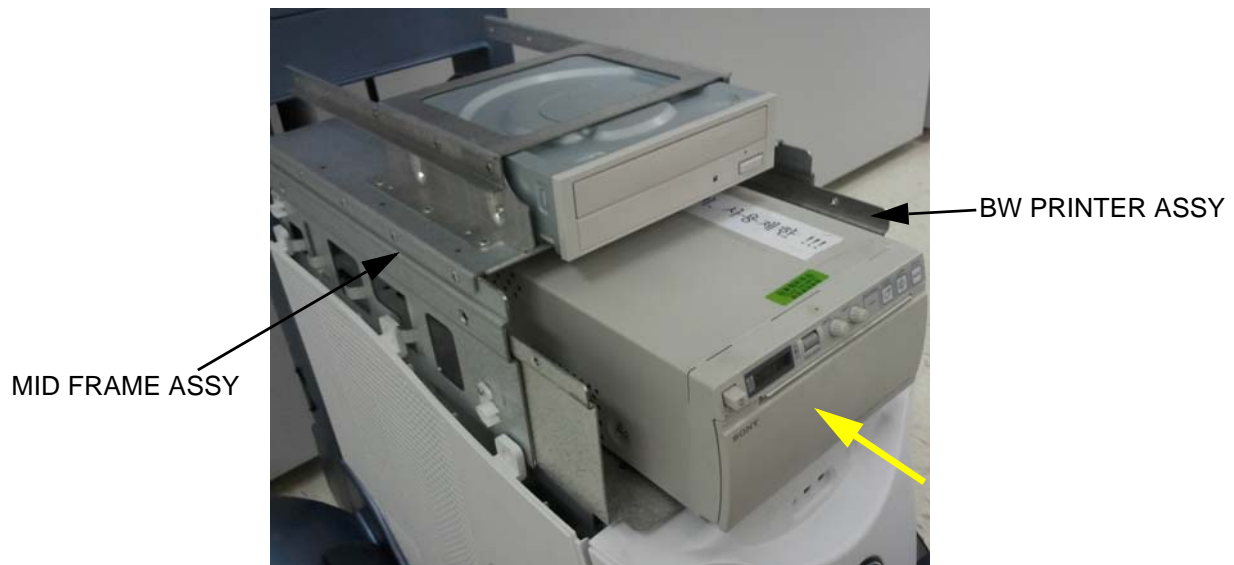
Figure 8-147 Inserting the BW PRINTER ASSY to the MID FRAME ASSY
