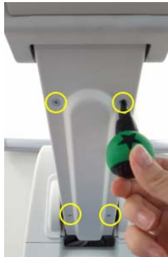
Figure 8-52 Unscrewing 4 screws to remove the ELEVATION ARM LOWER COVER LCF
