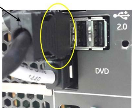
Figure 8-166 Connecting the COLOR PRINTER CABLE into the NEST
