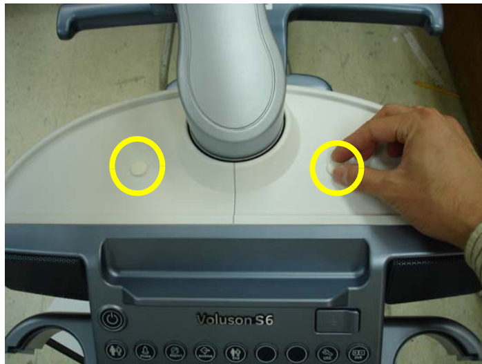
Figure 8-101 Removing the RUBBER CAP
