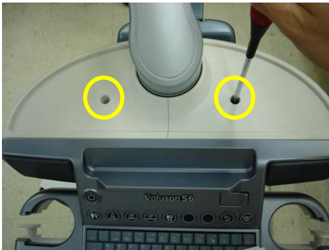
Figure 8-102 Removing the OPIO COVER L, R
