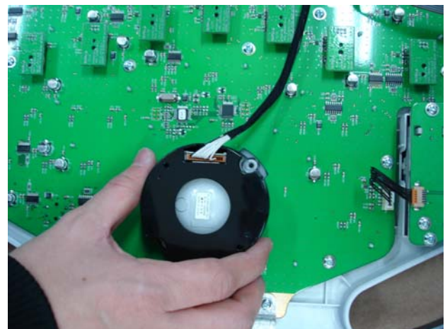
Figure 8-72 Unscrewing 2 screws and pulling out the TRACKBALL
