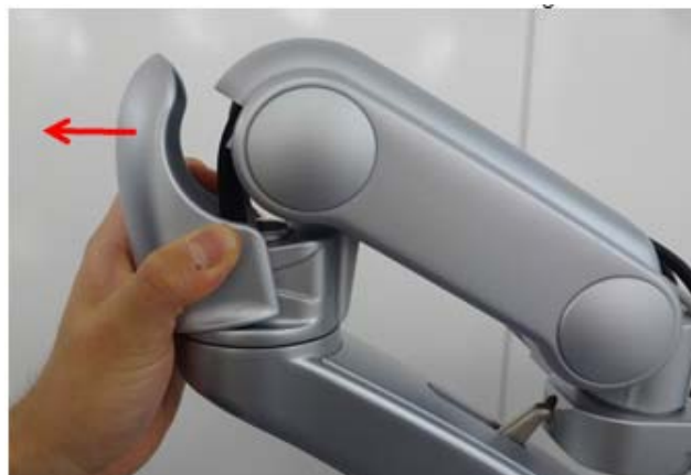
Figure 8-26 Removing the 2ND AXIS COVER
