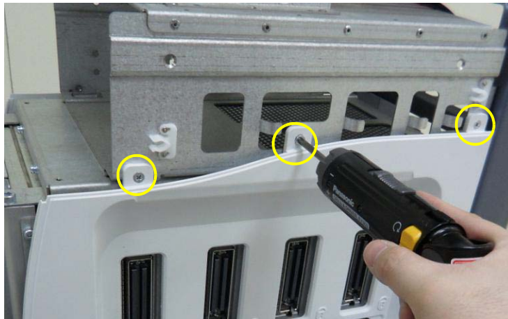
Figure 8-175 Unscrewing 3 screws to remove the SIDE COVER R ASSY
