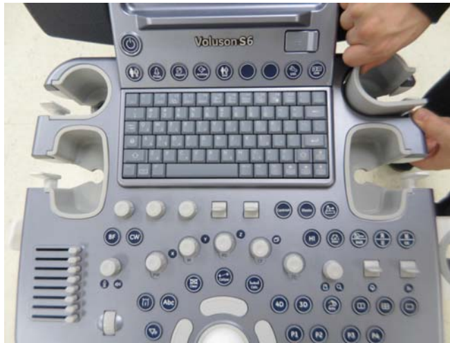
Figure 8-34 Removing the 4 PROBE HOLDERS
