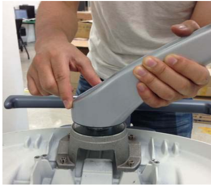
Figure 8-32 Removing the LCD ARM
