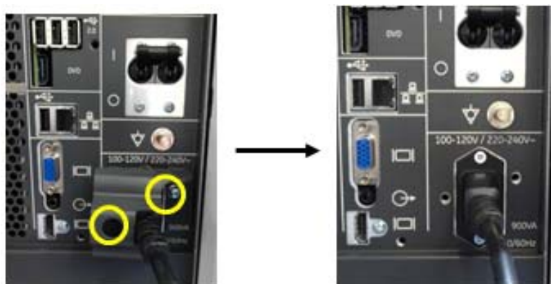
Figure 8-46 Unscrewing 2 screws to remove the POWER CORD FIX BRACKET and disconnect the Cable
