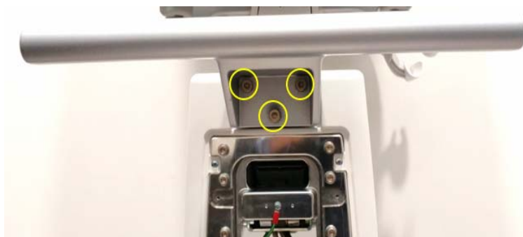
Figure 8-245 Unscrewing 3 screws to remove the HANDLE BT16
