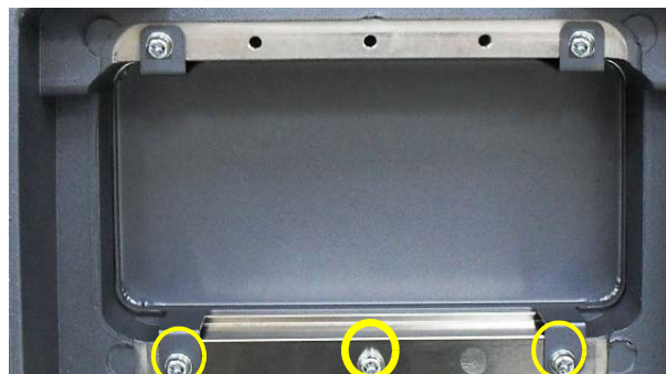
Figure 8-190 Assembling the HIGH FRAME GROUND BRKT with 5 screws (2159625, W/SP PH M4X8)
