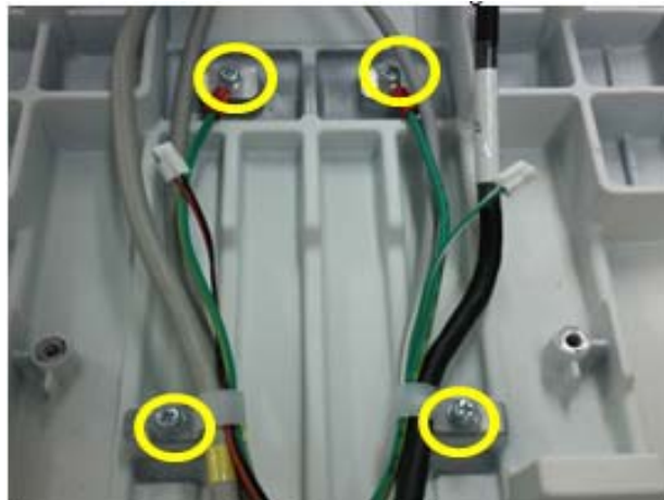
Figure 8-41 Unscrewing 4 screw to detach the cables
