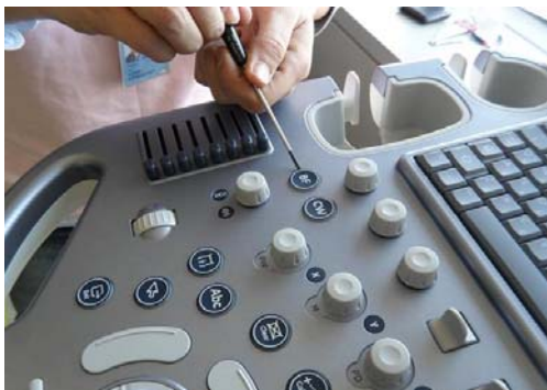
Figure 8-144 Pushing against the circle cap and lift it
