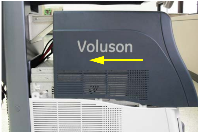
Figure 8-161 Assembling the HIGH CABINET ASSY
