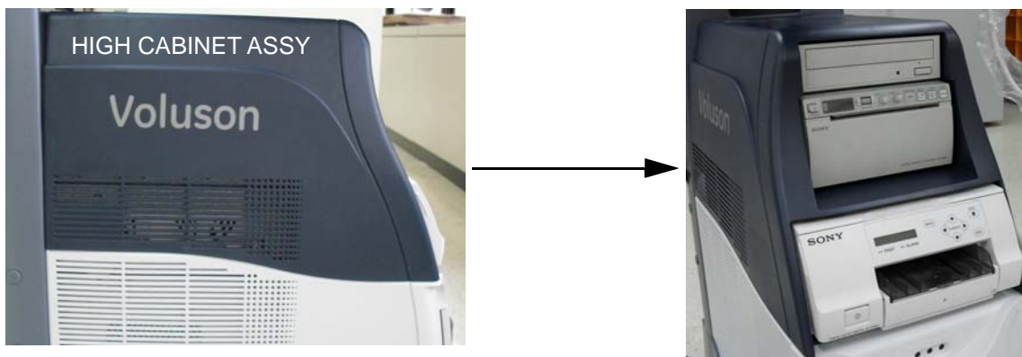
Figure 8-199 Assembling the HIGH CABINET ASSY
