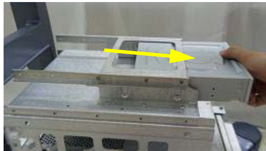
Figure 8-181 Removing DVD from the MID FRAME ASSY
