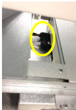
Figure 8-253 Disconnecting 2 cables from DVD
