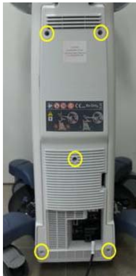
Figure 8-226 Unscrewing 5 screws to remove REAR COVER
