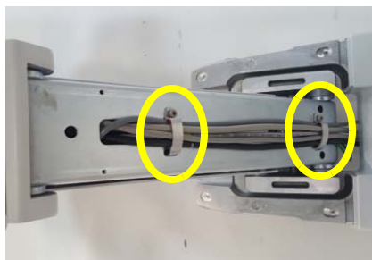
Figure 8-53 Unscrewing 2 screws to remove the ELEVATION CABLE CLAMP2
