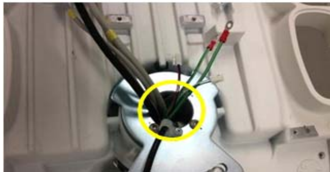
Figure 8-45 Pulling out the cables
