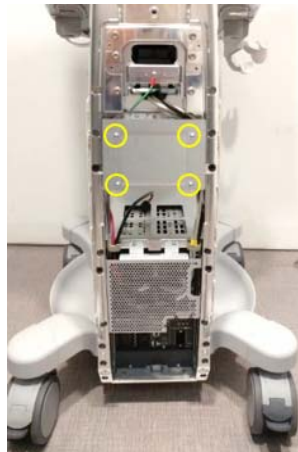
Figure 8-255 Unscrewing 4 screws to remove the SPEAKER FIX BRKT
