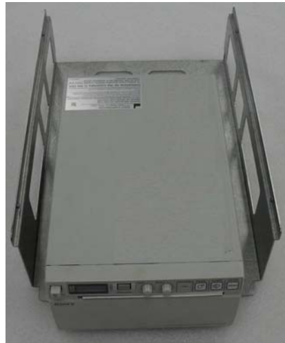
Figure 8-146 Fixing the BW PRINTER to the COLOR PRINTER BRKT POLARIS
