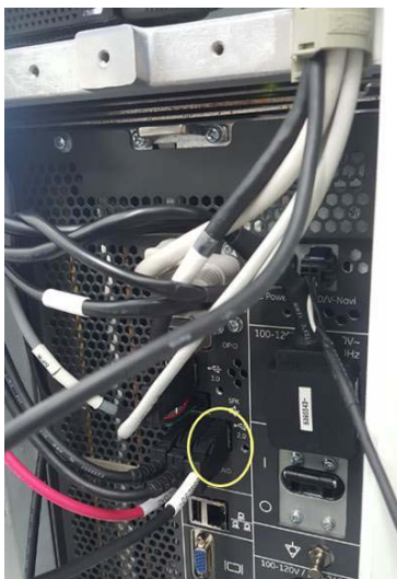
Figure 8-228 Disconnecting WIRELESS LAN cable from NEST BOX
