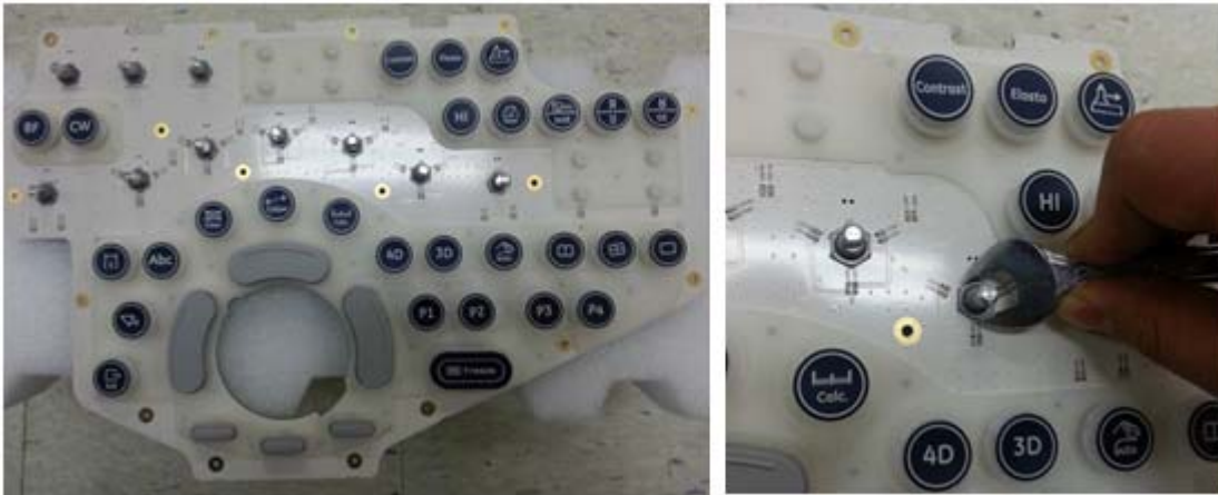
Figure 8-75 Unscrewing the nut of encoder and replace the encoder
