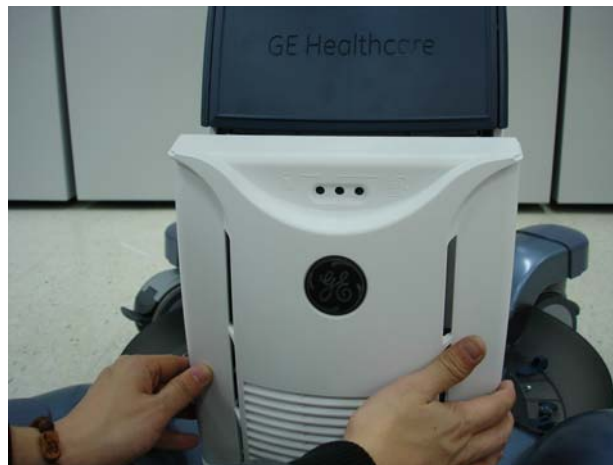
Figure 8-61 Removing the FRONT COVER ASSY
