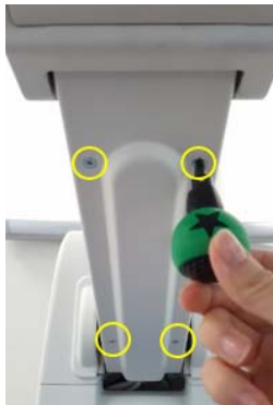
Figure 8-201 Unscrewing 4 screws to disassemble the ELEVATION ARM LOWER COVER LCF
