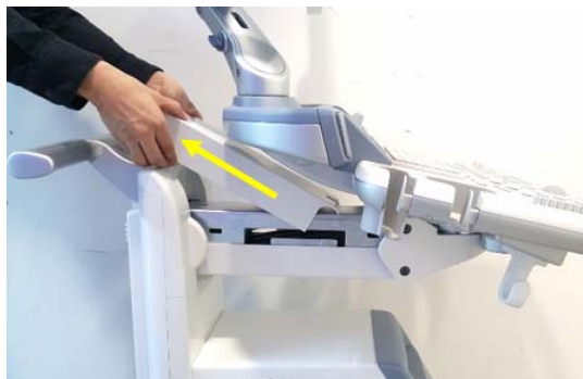
Figure 8-261 Removing the ELEVATION ARM UPPER COVER LCF
