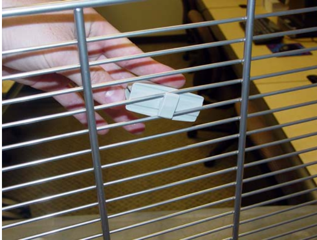
Figure 3-8. Rotate the Shelf Clip and Lock it Into Place
