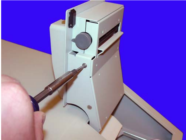
Figure 1-19. Remove the screws securing the printer assembly
