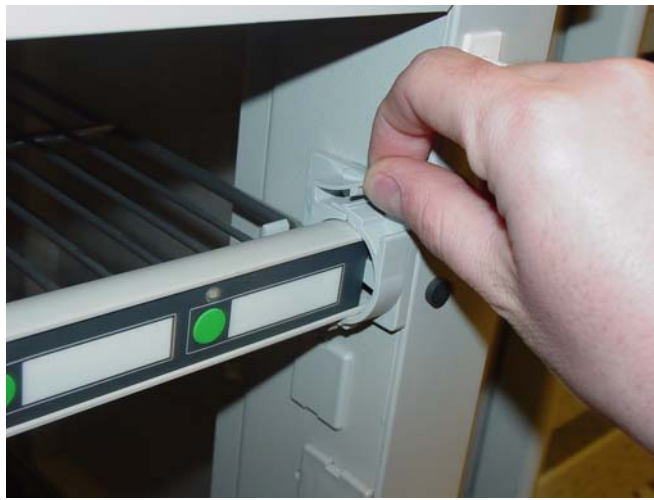
Figure 3-1. Lift the shelf clips
