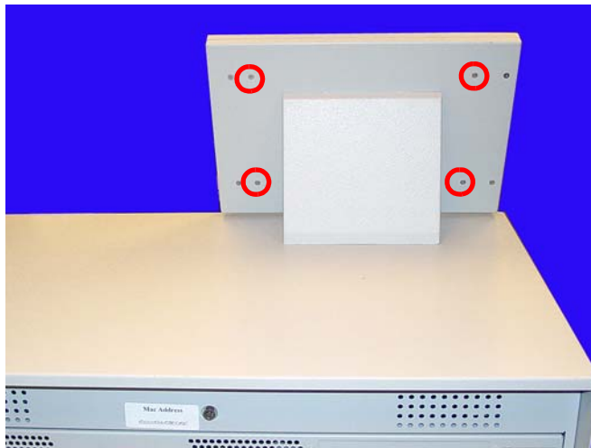
Figure 1-6. Remove the four inner screws
