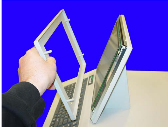
Figure 1-5. Remove the front bezel
