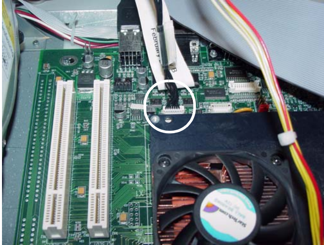
Figure 1-1. Disconnect the video image cable.
