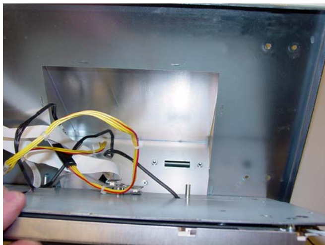
Figure 1-7. Remove the cables from the opening in the lid
