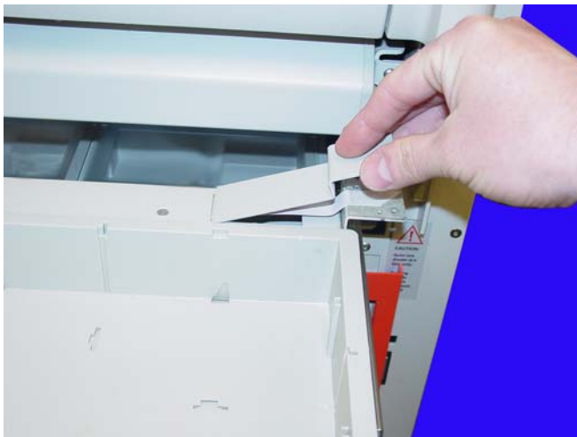
Figure 6-8. Remove the controller cable cover
