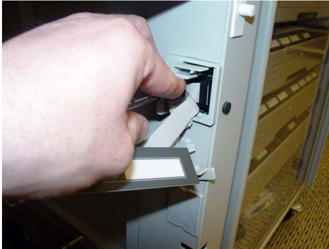
Figure 3-2. Disconnect the switchpanel from the SPC board
