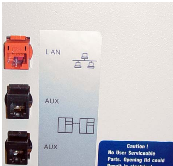
Figure 1-24. Location and labels for LAN and AUX cable connections on CT PC Tray
