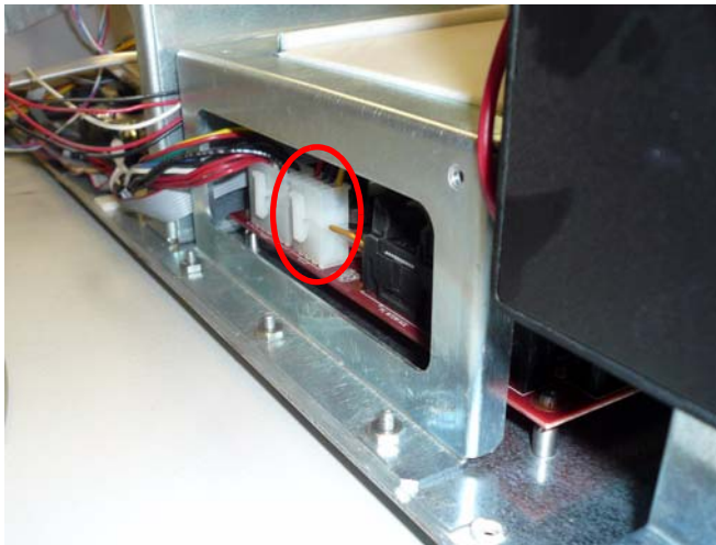
Figure 1-14. Disconnect the battery cable
