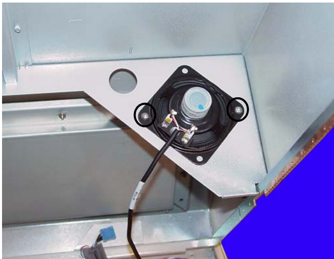
Figure 1-9. Remove the two screws that secure the speaker
