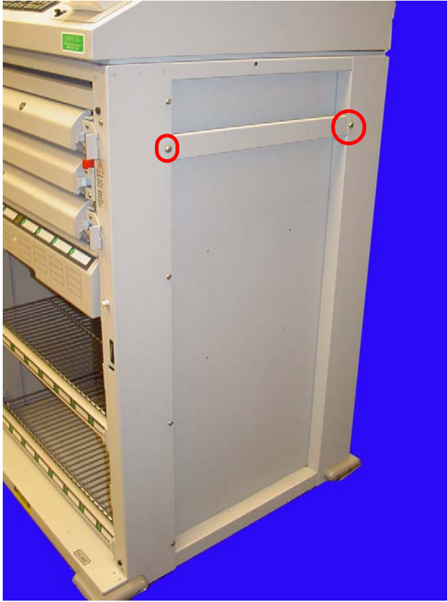
Figure 2-3. Remove the two screws securing the transport handle
