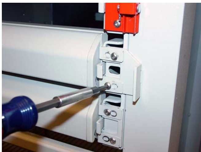
Figure 6-4. Remove the screws securing the false drawer front
