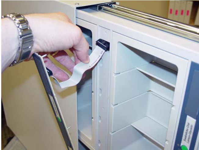
Figure 4-5. Remove the Switchpanel from the Drawer
