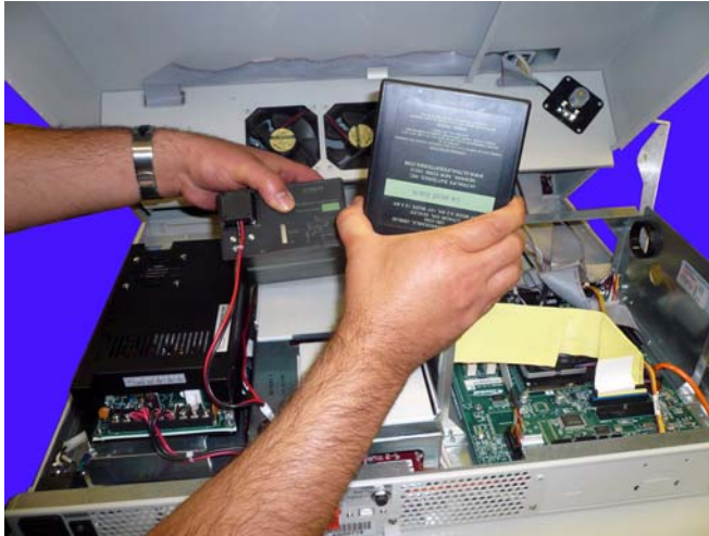
Figure 1-13. Lift the batteries off the stand
