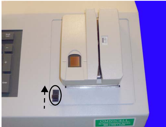
Figure 1-17. Open the printer cover
