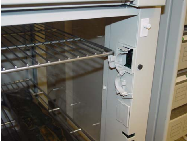
Figure 3-4. Push the shelf up and remove
