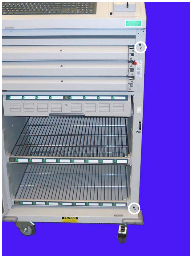
Figure 2-2. Remove the two screws on the front of the half cell
