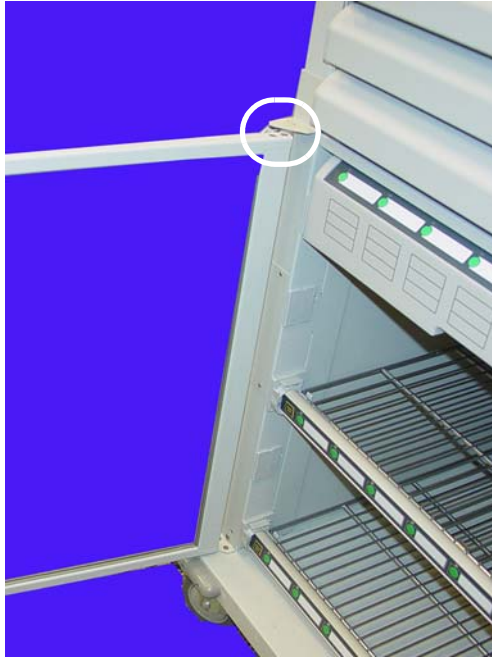
Figure 5-1. Remove the screws securing the top bracket
