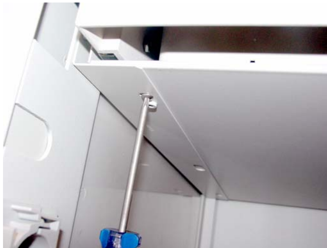
Figure 4-4. Remove the screws securing the drawer to the mounting bracket
