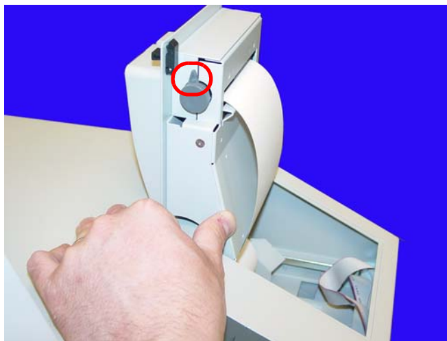
Figure 1-18. Push the platen lever to the left and remove the paper
