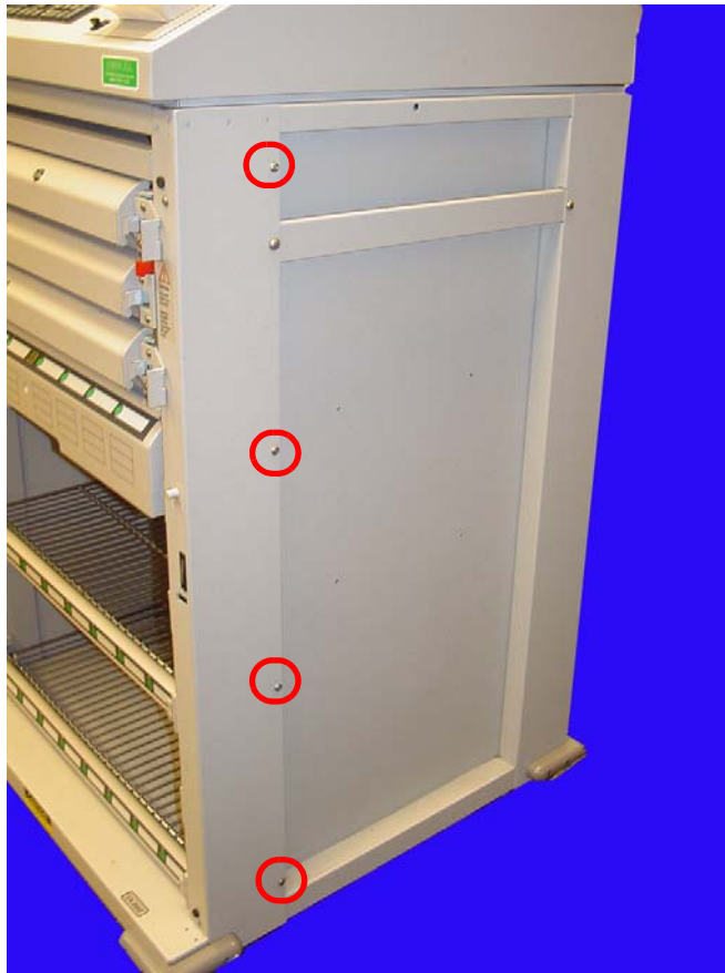
Figure 2-1. Remove the four screws on the side of the half cell
