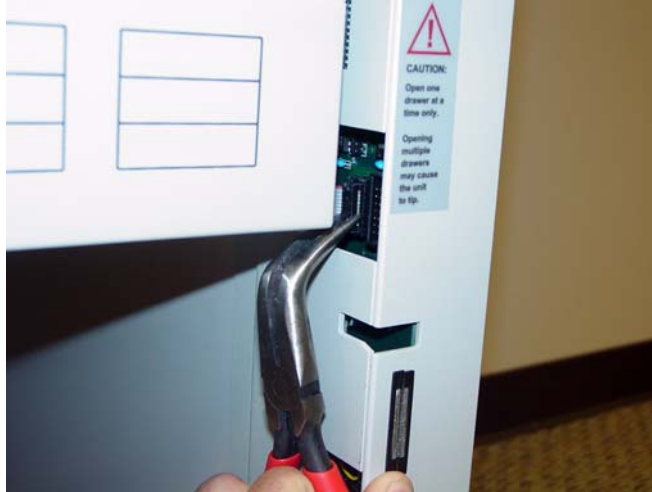
Figure 4-3. Disconnect the Switchpanel from the SPC Board in the Wireway
