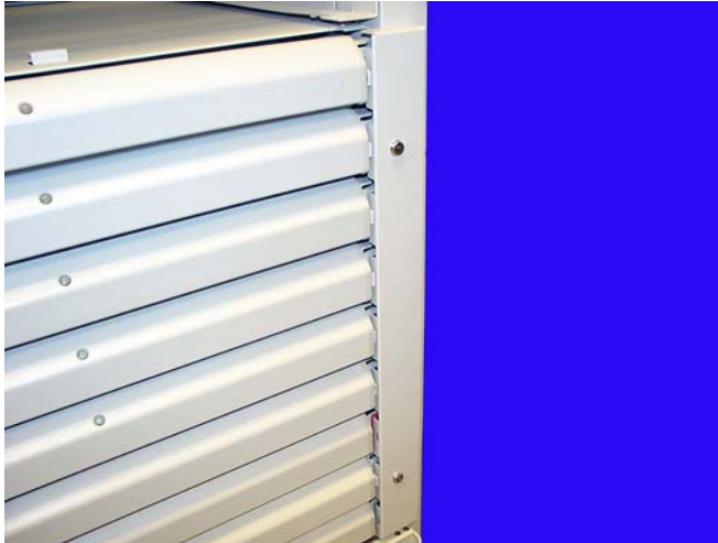
Figure 6-7. Remove the manual override cover
