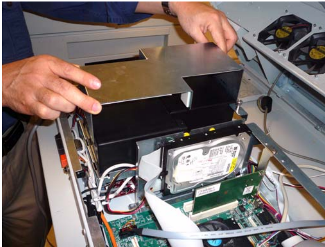
Figure 1-11. Slide the battery cover
