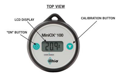
**LCD Display:** A 3-digit display provides a direct readout of oxygen concentration in the range of 0 - 100%. The display is blank when the MiniOX 100 enters its Sleep (power off) mode. The MiniOX 100 will automatically enter the Sleep mode after approximately 1.3 minutes from the last time the ON button was pressed.
