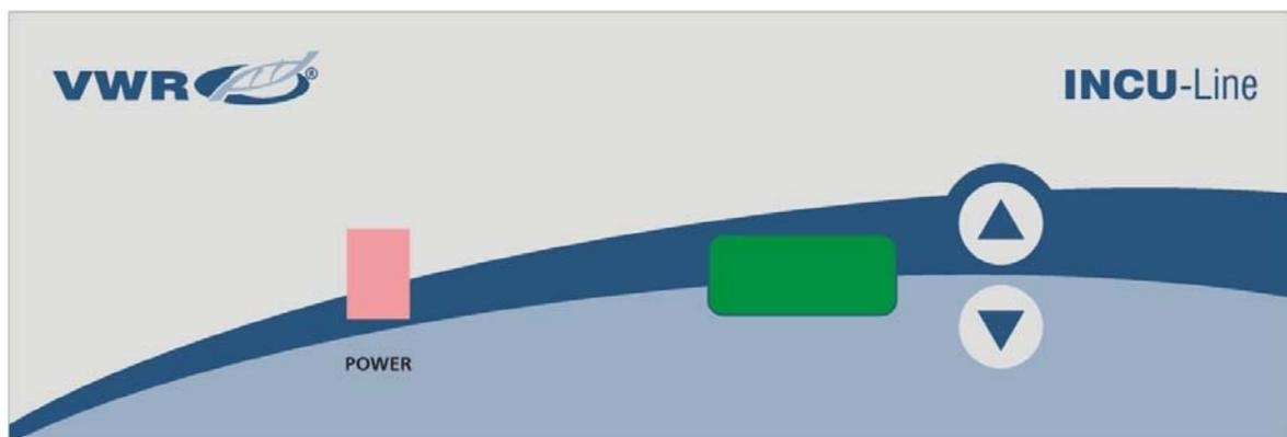
POWER - power switch: For turning the incubator ON and OFF. It lights when incubator is switched ON.
