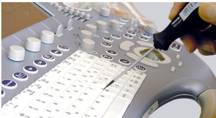
Figure 8-23 Key Cap Replacement
