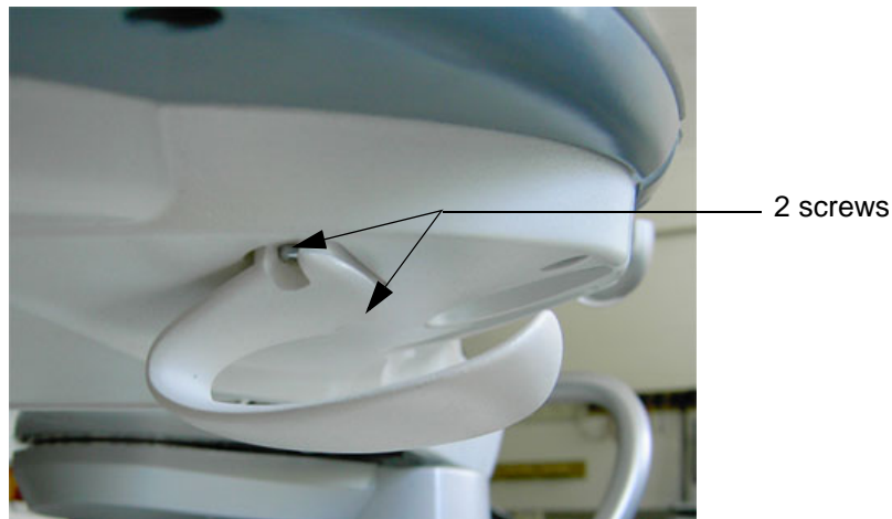
Figure 8-19 loosen 2 screws and remove cable holder
