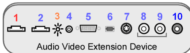
Figure 54: AVED: Audio Video Extension Device I/O Panel Diagram
