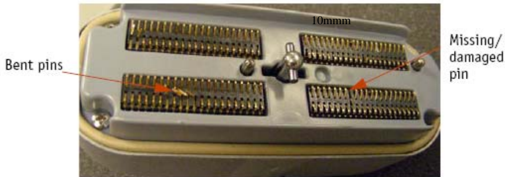
Figure 62: Transducer Connector Pin Damage - (Example)
