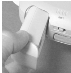
Figure 36: Battery Pack Installation
