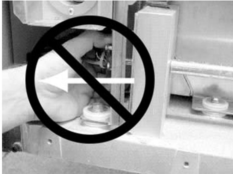
2. Use a long, thin needle nose pliers and place on the elevation shaft, behind the coupling tube.
