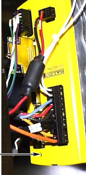
Arrow points to the Drive Controller fault status LED
