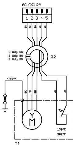
E2753 (250Ω) = 2,1 ohms between 2 motorwires
