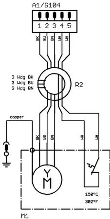
E2753  $R_{BKBU} = 2,1 \text{ ohms}$  between 2 motorlines
