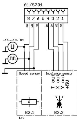
During centrifugation the speedometer pulses of the speed sensor (B2.1) at the bottom of the motor are interrupted.
