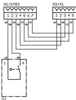
Position switch "Mc" of the motor-driven lid lock opens during the centrifugation run.
