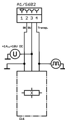
After start-up no speedometer pulses will be received from the speed sensor (B4) on top of the motor.
