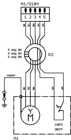
E2753 (Z500) = 2,1 ohms between 2 motorwires
