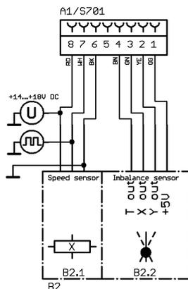
The frequency converter recognises excess speed. It evaluates the signals from the speed sensor (B2.1) at the bottom of the motor.
