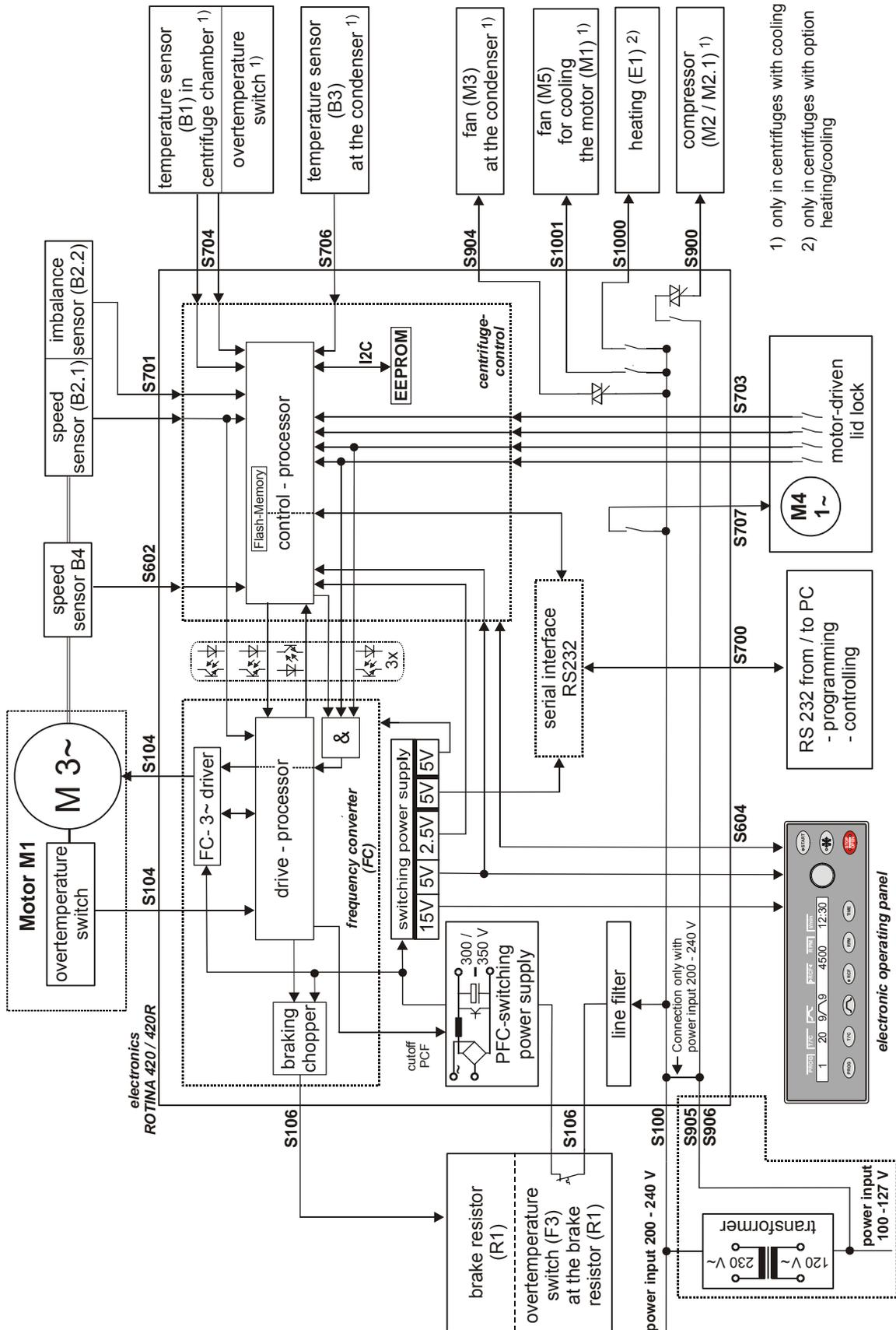
These microprocessor controlled centrifuges mainly consist of the following electrical components:
