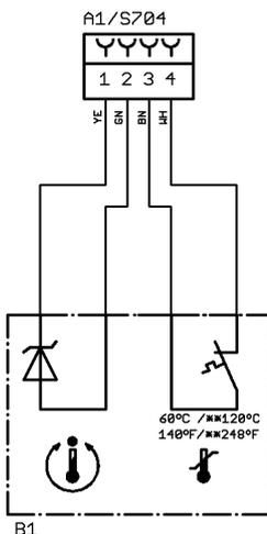
The temperature in the centrifuge chamber measured by the temperature sensor (B1) is out of the valid range.
