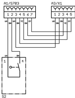
Position switch "Mo" of the motor-driven lid lock closes during the centrifugation run.
