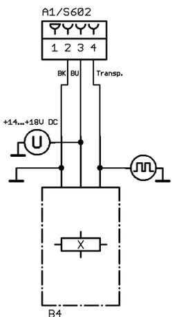
Excess speed. The speed measured by the speed sensors B4 or B2.1 is 250 RPM higher than the maximum speed of the rotor.
