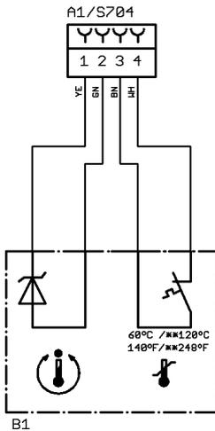
Overtemperature in centrifuge chamber
