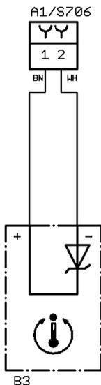
The temperature on the condenser measured by the temperature sensor (B3) is out of the valid range.
