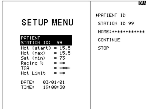
From this point, follow the instructions in the previous section for entering the PATIENT and STATION ID and NAME. To get back to the PROFILE screen, scroll to CONTINUE in the SETUP MENU and press SELECT. This will return you to the START UP screen, which will then automatically revert to the PROFILE screen after 10 seconds.
