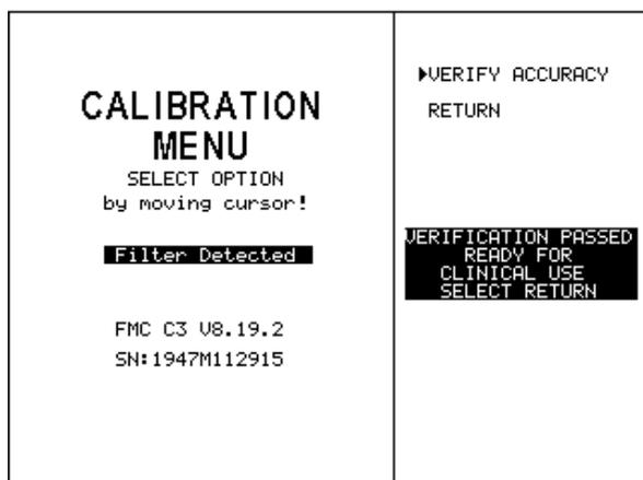
If the CLM III is unable to verify accuracy, it will prompt you to retry the VERIFY ACCURACY routine again after ensuring that the sensor clip is properly attached to the verification filter and the verification filter is clean.
