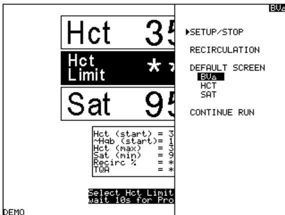
The STARTUP/SPLIT screen menu appears after pressing the MENU key while viewing the STARTUP screen. Its icon is the same as the STARTUP screen without the menu displayed.
