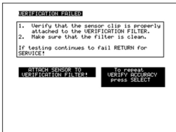
If the VERIFY ACCURACY routine fails the second time, the monitor will return to the original CALIBRATION MENU. Check to make sure that the sensor clip is properly attached to the verification filter.
