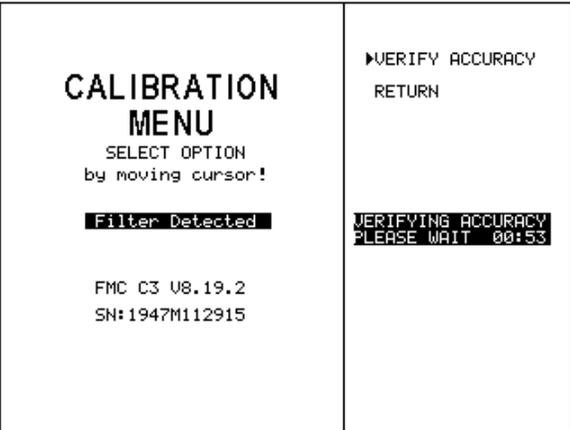
In sixty seconds, one of two possible messages will be displayed. Verification Passed or Verification Failed.
