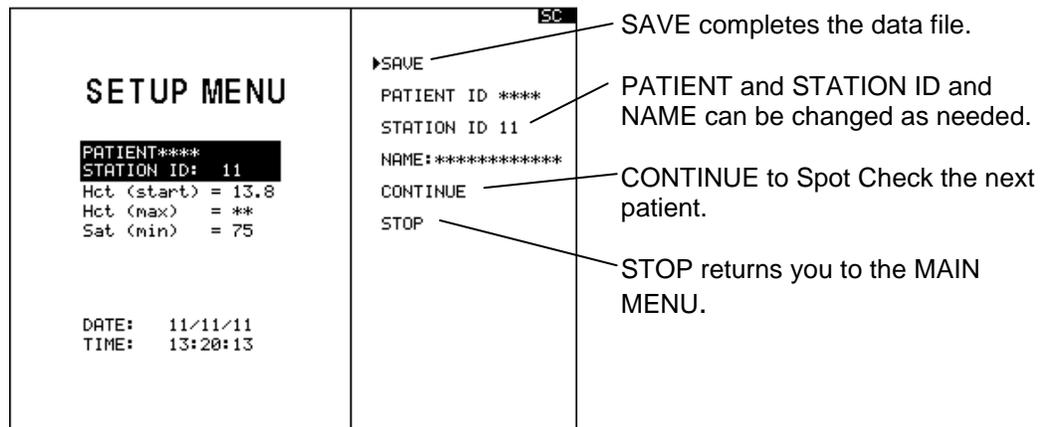
Whenever SAVE is selected, the current PATIENT ID and STATION ID are recorded into memory along with their corresponding Hct and O<sub>2</sub> Sat readings.
