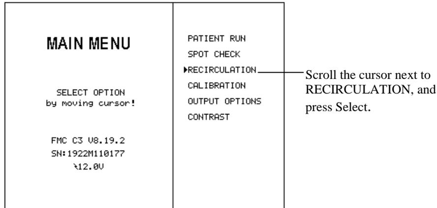
This feature is also available during a patient run. To momentarily leave profile monitoring and conduct a recirculation test, press MENU or SELECT to move to the START-UP screen. Then press MENU to bring up the START-UP menu.
