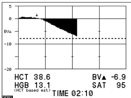
The PROFILE screen displays a plotted graph of the change in the measured parameters versus time to allow you to see the trend in those measurements.
