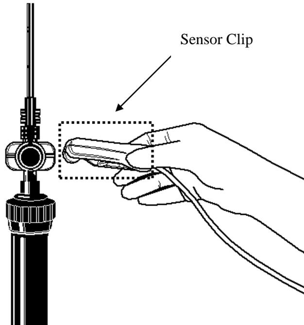
Whenever the CLM III is not being used, the sensor clip should be placed on the verification filter on the side of the monitor. This provides protection from damage and keeps the sensor elements clean. (See section 8 for cleaning instructions). **Never remove the clip from the verification filter by pulling on the sensor cable.**
