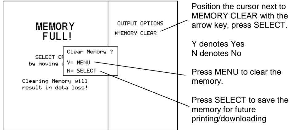
**NOTE:** Once the memory has been cleared, data cannot be retrieved. If you do not want to clear the data (i.e. you want to print or download data prior to erasing) the output options feature must be selected (see Section 4 – Output Options).
