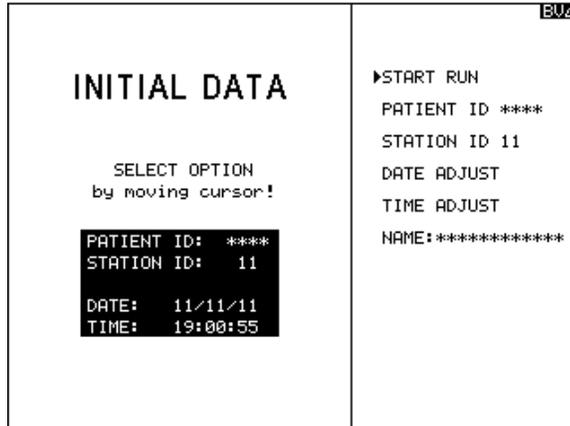
The INITIAL DATA screen allows the input of various parameters. It appears after selection of PATIENT RUN, SPOT CHECK, and RECIRCULATION on the MAIN MENU.
