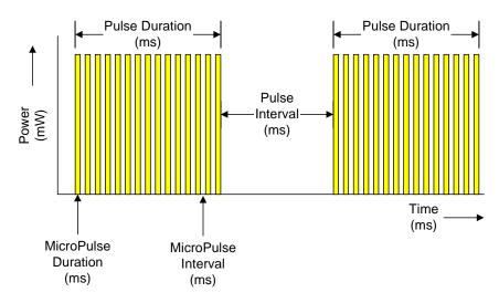
The percentage of time the treatment laser is activated during each pulse is referred to as the duty factor. The duty factor is calculated according to the following formula:
