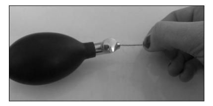
Sometimes dirt accumulates in the tube, too. The dirt impedes air flow through the tube. To remove the dirt, insert a long wire into the open tube end. Gently push the wire into the tube until the wire reaches the cuff. Pull out the wire.
