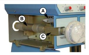
Refitting the silencer and exhalation block is the reversal of removal. **Do not force the** exhalation block into place.
