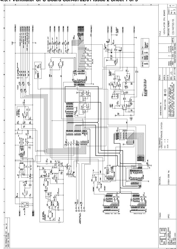
14.3.1 Ventilator CPU Board CD/A0702/01 Issue 2 Sheet 1 of 3
