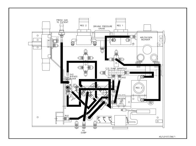
Gas from the AIR/OXYGEN Blender is supplied to the preset regulator REG3 via the supply manifold. The output of REG3 is set to 10PSI and is fed to two flow valves.
