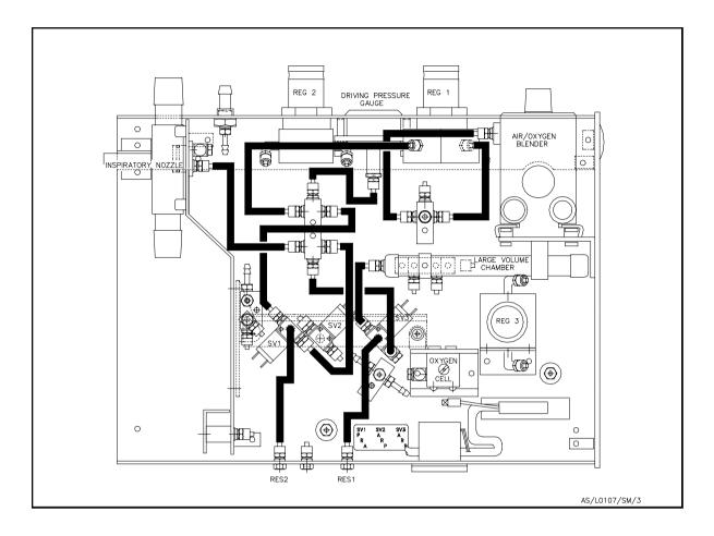
Gas from the AIR/OXYGEN Blender is supplied to the user adjustable PIP regulator REG1 through the supply manifold. The output pressure of REG1 is supplied to the inspiratory nozzle via the solenoid valve SV1 which controls the breathing rate. If the pressure wave switch is in the taper position then SV3 is energised and the inspiratory flow enters the large volume chamber before reaching the inspiratory nozzle, thus lengthening the pressure rise time.
