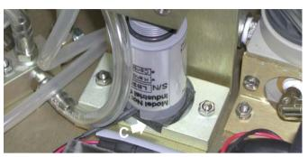
6. Ensure that the foam rubber pad is fitted between the cell and the mounting base and that the gas seal "O" ring is fitted to the manifold. After refitting, recalibrate the cell.
