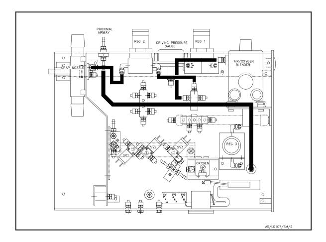
Gas from AIR/OXYGEN Blender is supplied to the CPAP pressure regulator REG2 via the supply manifold. The output pressure of REG2 is fed to the CPAP nozzle in the expiratory manifold, and into the expiratory limb of the patient circuit to create the circuit CPAP pressure.
