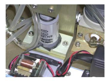
2. Remove the two screws (B) retaining the manifold and lift it clear.
