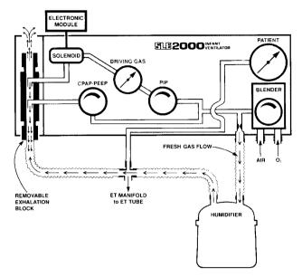
The PIP regulator and gauge on the front panel set the pressure that is supplied to a solenoid valve which is connected to the rear nozzle. The Electronic Module controls the rate and duration of the flow of Driving Gas into the Exhalation block in opposition to the Fresh Gas flow. This opposing flow acts as a pneumatic piston and creates a pressure wave at the ET manifold. The lung inflation pressure and hence the tidal volume are controlled by the PIP regulator.
