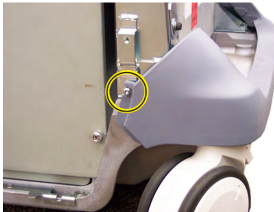
Figure 8-27 Left screw placement for Rear Bumper
