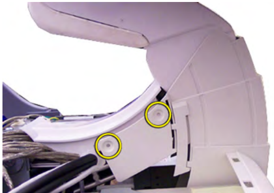
Figure 8-31 With console raised, left side screw placement
