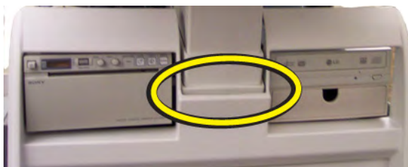
Figure 8-32 Position the column cover inside the front cover
