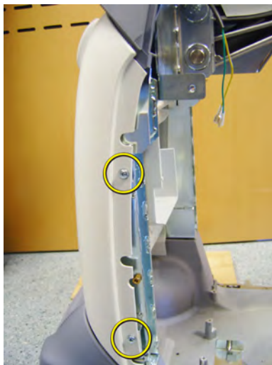
Figure 8-21 Rear Cover fixing screws
