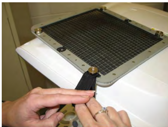
Figure 8-57 Placement of Fingers in Looped Strap
