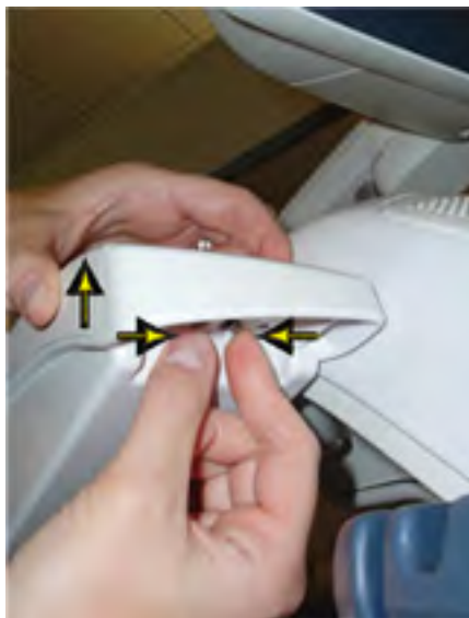
Figure 8-52 Squeeze the two prongs
