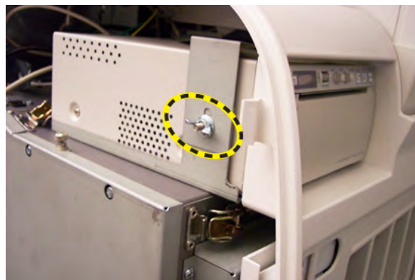
Figure 8-69 Black and White Digital Graphic Printer - wing nut
