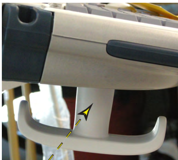
Figure 8-55 Screw placement, Probe Cable Hook
