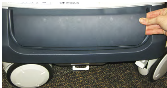
Figure 8-20 Remove the Filter Cover
