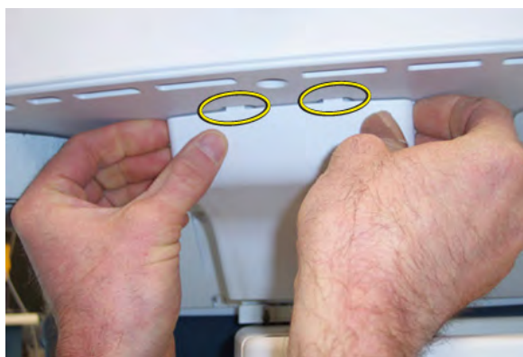
Figure 8-40 Upper lock tabs (placement on Bulkhead Cover)
