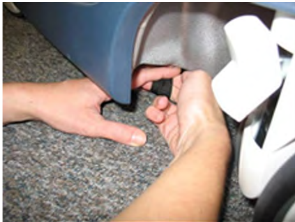
Figure 8-56 Bottom Filter Looped Strap (located in wheel well)
