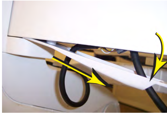
Figure 8-37 Pull down and slide XY / Frogleg cover out
