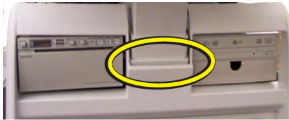
Figure 8-34 Position the column cover tab inside the front cover
