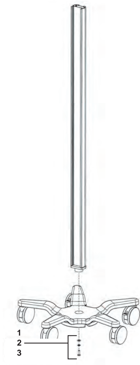
Figure 8-72 Post into Base - (1) 5/16 fLAT Washer, (2) 5/16 Lock Washer, (3) 5/16-18 x 1 inch Screw - Roll Stand only
