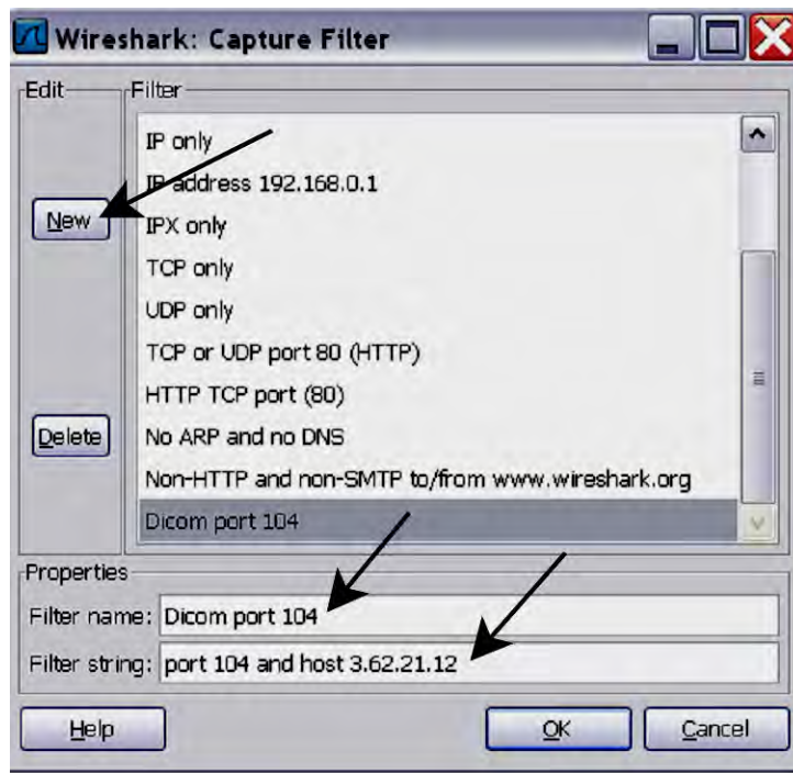
Figure 7-15 Sniffer Capture Filter IP and Port
