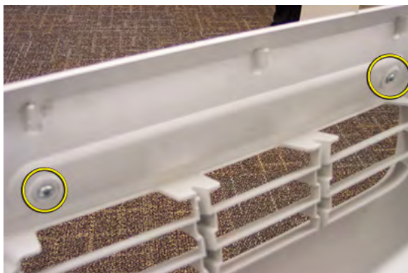
Figure 8-26 Cable Hook screw placement
