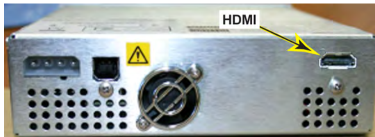
Figure 5-21 V Nav Inside Option HDMI Auxiliary Sensor Input from GRLY
