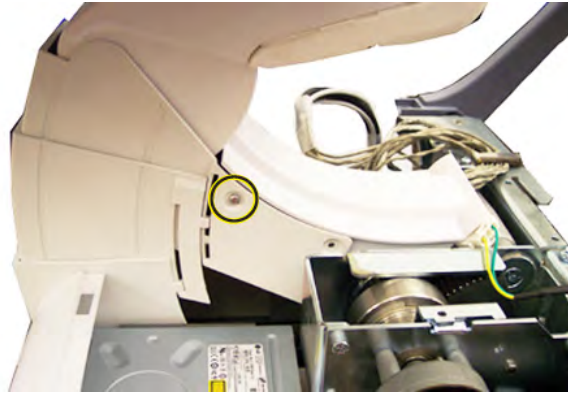
Figure 8-30 With console raised, upper right side screw placement
