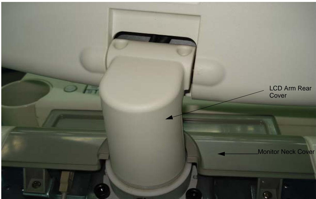
Figure 8-4 LCD Arm Rear Cover and Monitor Neck Cover
