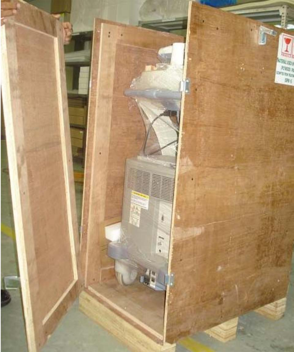
Figure 3-3 Removing the front plywood
