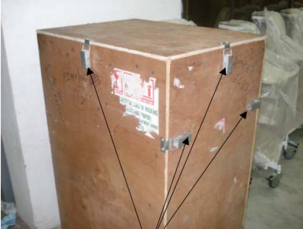
Figure 3-1 The metal bands to be removed
