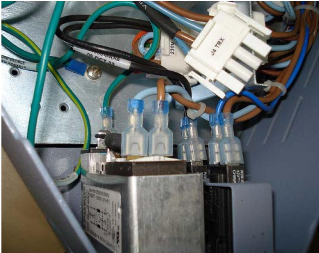
Figure 8-54 Power Entry Module
