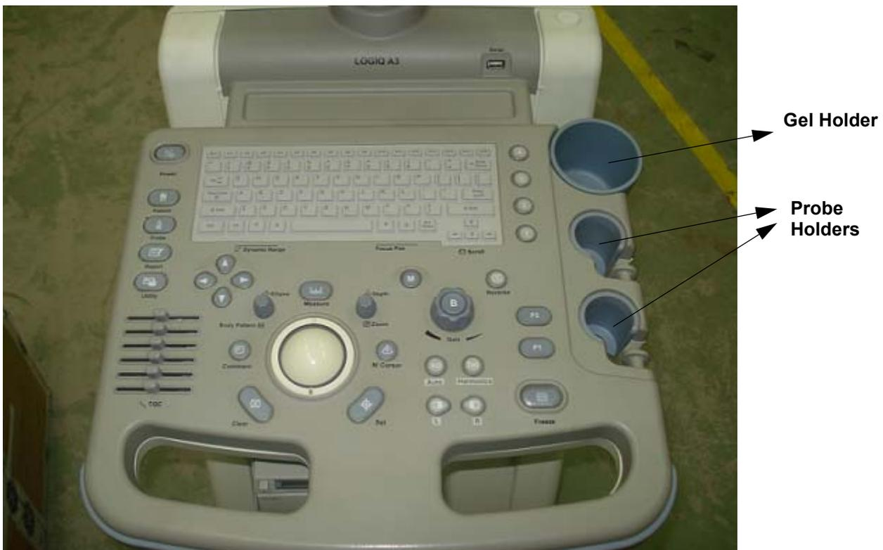
Figure 8-7 Key Board Top View
