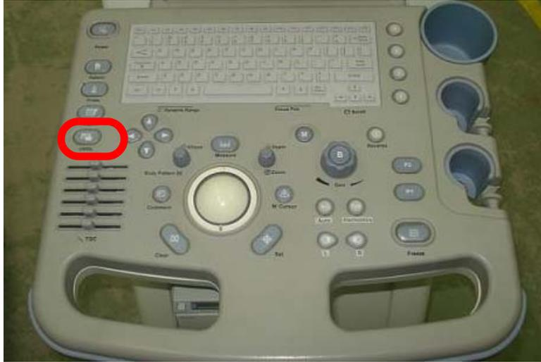
Figure 7-6 Utility button on keyboard
