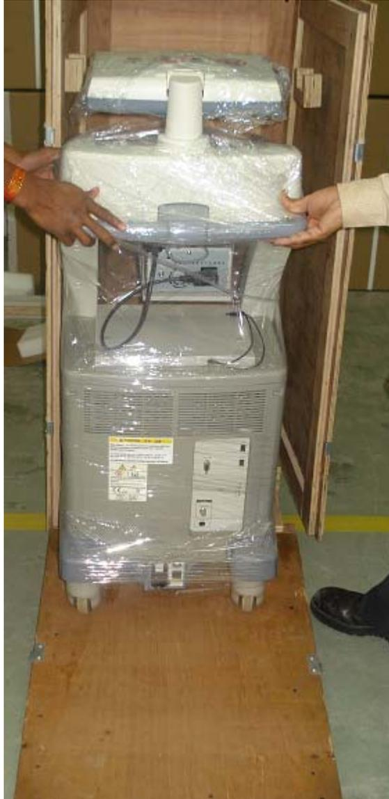
Figure 3-5 Moving the LOGIQ A3 from the crate
