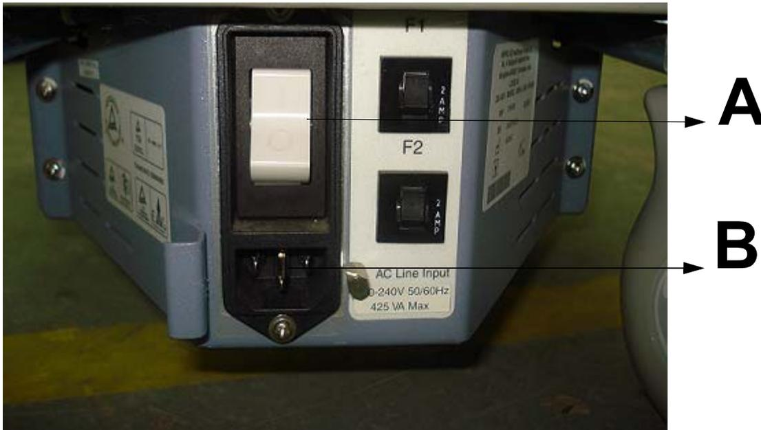
**Figure 3-8 Circuit Breaker and Power Cable on Back of Scanner**
