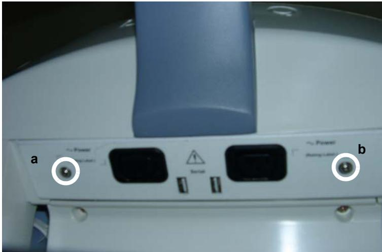
**Figure 8-38 Removing Front Panel Assembly**
