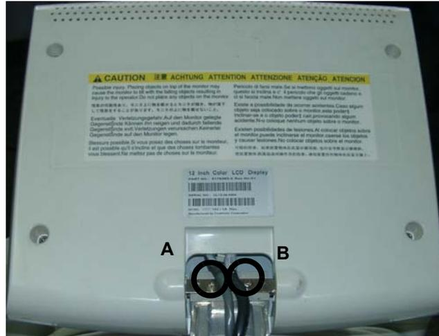
**Figure 8-3 Remove LCD Assembly**
