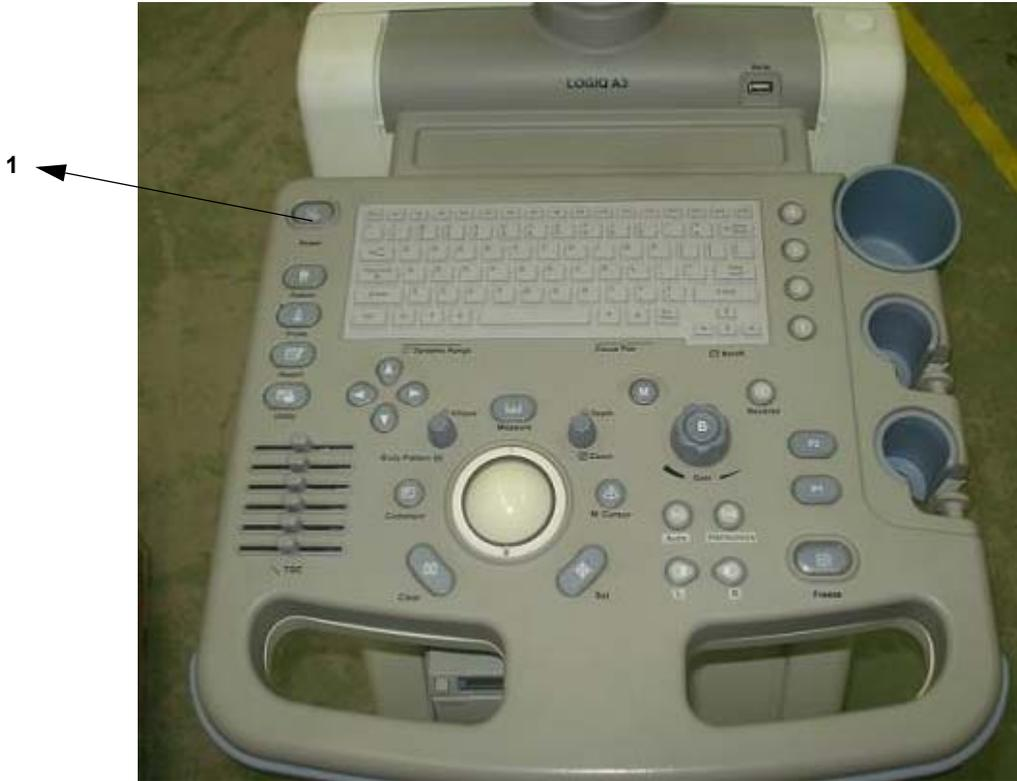
**Figure 3-9 Power On/Off Switch for Back-end Processor Boot Up**
