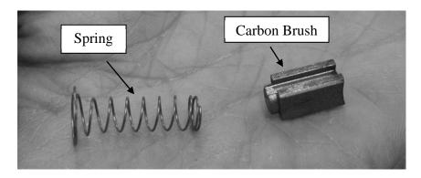
Examine the springs. Determine whether or not any of the springs need to be replaced. Purchase a replacement spring if any of the springs are burnt, rusty, melted, or rigid. Purchase a replacement spring if any of the springs are deformed or broken. Try to purchase a spring with similar dimensions and similar elasticity to the original spring. Attach the new spring to the carbon brush. The diameter of the spring should ideally be slightly smaller than the attachment point on the brush.
