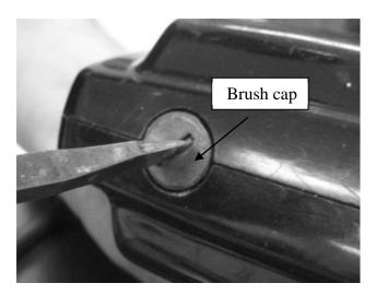
Carbon brushes are attached to coil springs. Check the springs if the motor is turning slowly or not at all. Springs that prevent the carbon brushes from making full contact with the commutator must be replaced. Springs that are burnt, rusty, melted, or rigid must be replaced. Springs that are deformed or broken must be replaced.
