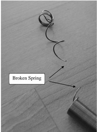
Springs that are detached from the carbon brush must be reattached.
