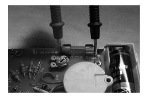
If the fuse is intact, the resistance will be 0 ohms, the buzzer will sound, or the screen will read 'short.' A nonfunctional fuse will have a very high resistance or the reading 'open.'
