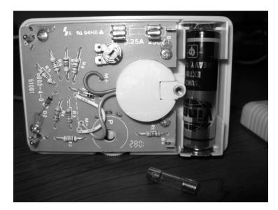
Replace the old fuse with an identical, functional fuse. The new fuse must match the amperage, voltage, and type of the previous fuse.
