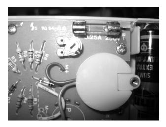
Use your continuity tester or multimeter to test the fuse. To use the continuity tester, place one lead on either end of the fuse. The LED will illuminate if the fuse is still functional.
