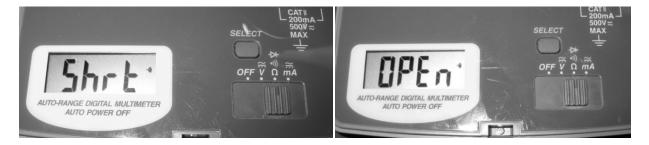
Immediately replace a nonfunctional fuse. Most devices will not function with a nonfunctional fuse. Remove the old fuse, and check the amperage rating, voltage rating, and type.
