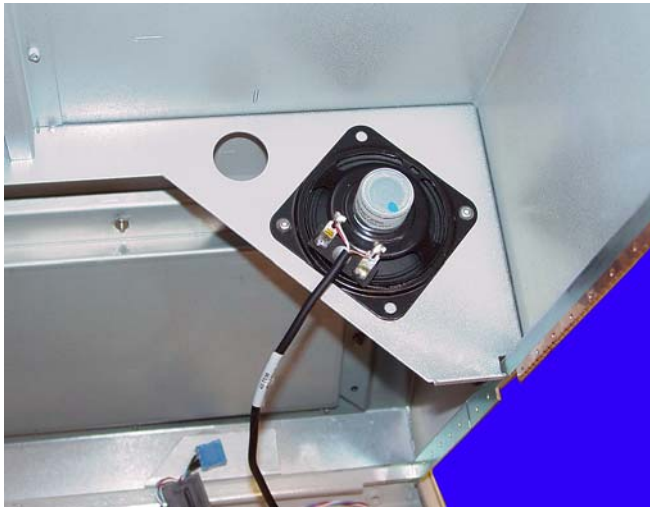
Figure 1-4. Remove the two screws that secure the speaker
