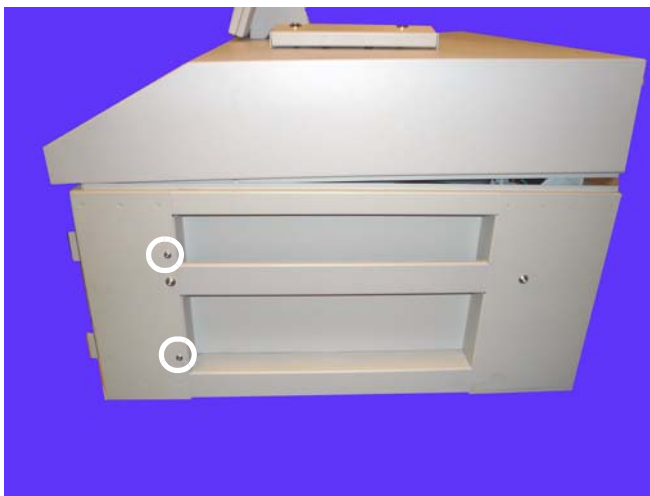
Figure 2-1. Remove the two screws securing the wireway
