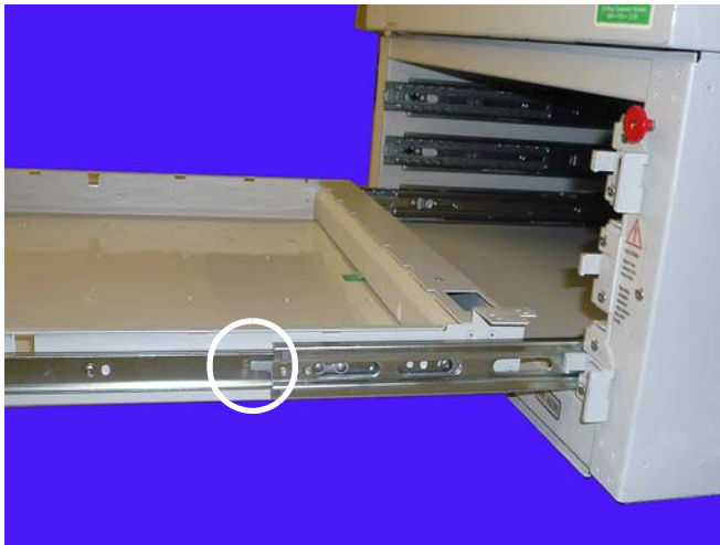
Figure 3-11. Push the release levers to release the drawer
