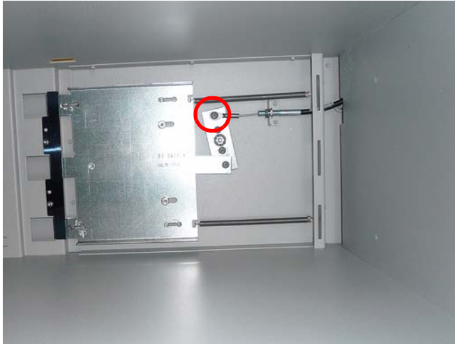
Figure 2-9. Remove the screw that secures the cable to the manual override assembly.
