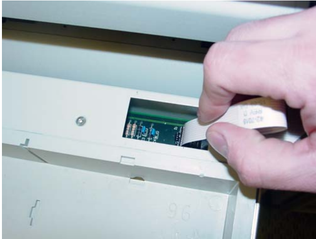
Figure 3-10. Remove the controller cable
