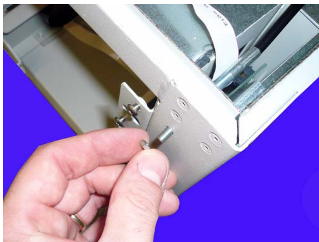
Figure 2-8. Remove the nut that secures the manual override cable to the frame.
