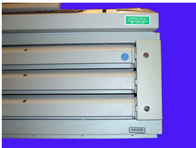
Figure 3-7. Remove the manual override cover
