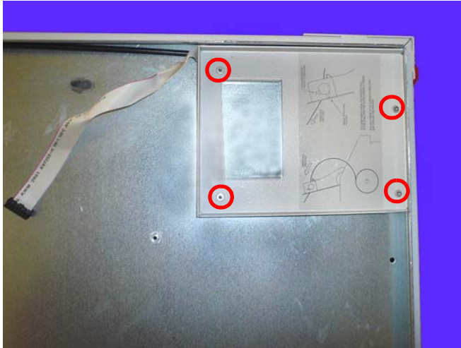
Figure 2-5. Remove the four screws that secure the printer support bracket to the frame
