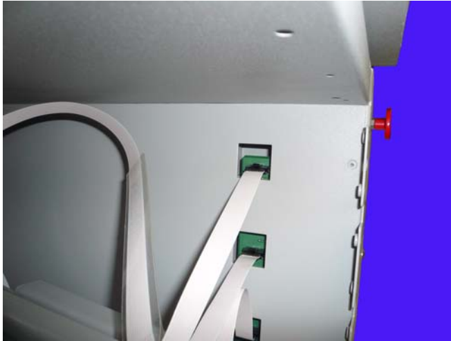
Figure 3-4. Connect the drawer cable to the drawer connect board
