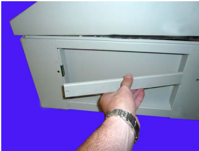
Figure 2-3. Pull the transport handle toward the rear of the cabinet then remove it
