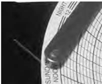
Chart recorder stylus and time line groove
