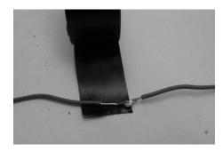
The picture above shows initial placement of the electrical tape. Notice that the tape overlaps the insulation on the wire.
