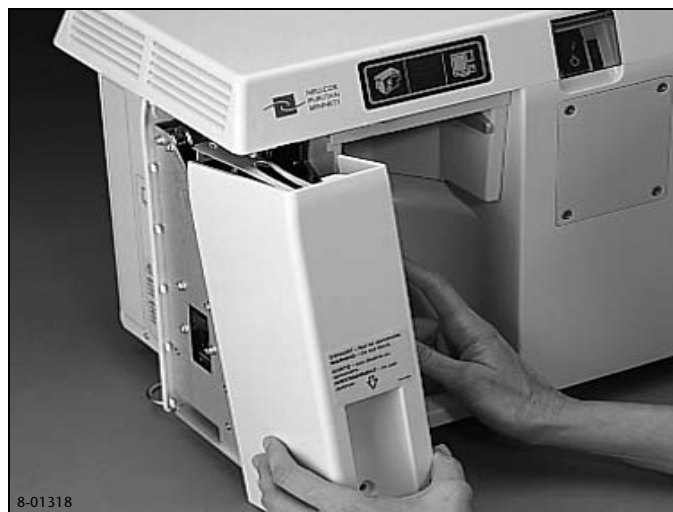
Figure 8-63. Removing exhalation module cover
