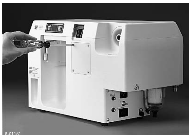
Figure 8-42. Replacing humidifier receptacle
