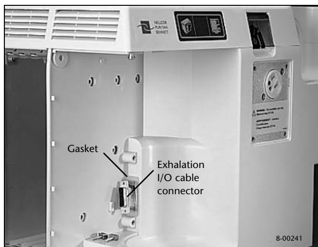
Figure 8-71. Removing BDU housing
