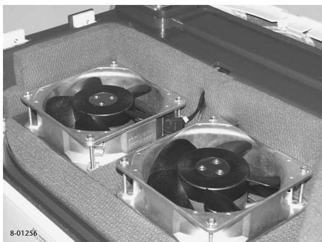
Figure 8-81. Fans installed in compressor
