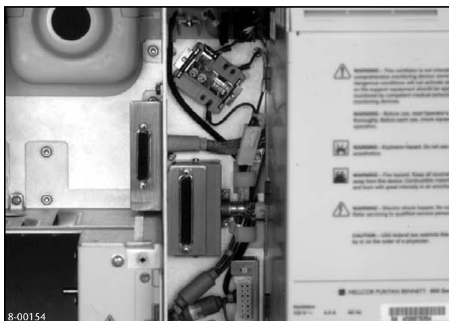
Figure 8-42. Replacing humidifier receptacle
