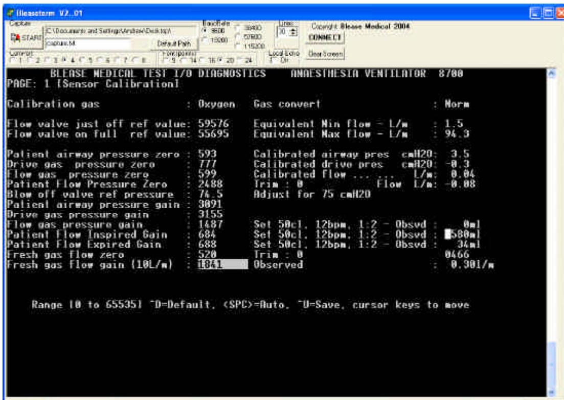
**Figure 48 Fresh Gas Flow Sensor Gain**
