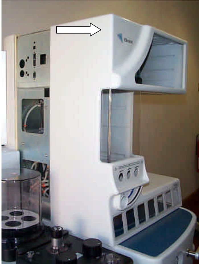
**Figure 6 Removal of Front Moulding**
