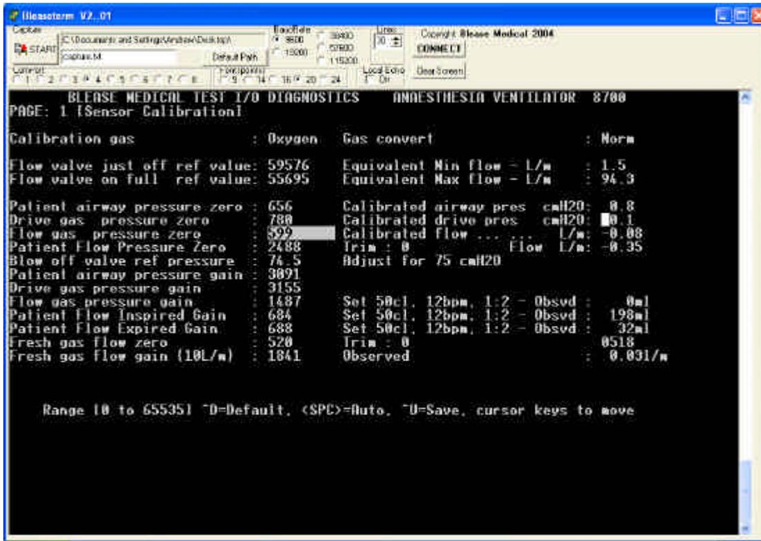
Adjust the pre-set potentiometer VR3 until 600 +/- 10 is shown. Note: the number in the cursor box will only update when the space bar is pressed. Therefore, it is necessary to make a small adjustment then press the space bar to update the number then if necessary make another small adjustment, press the space bar to update again repeating until the correct value is shown.
