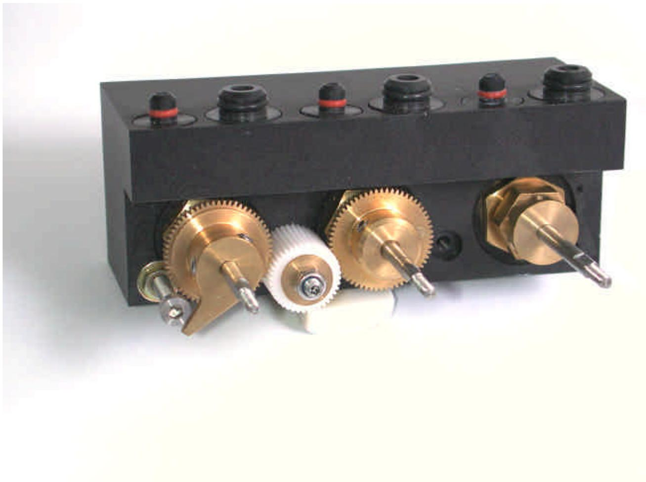
**Figure 13 Assembled Hypoxic Guard Unit**
