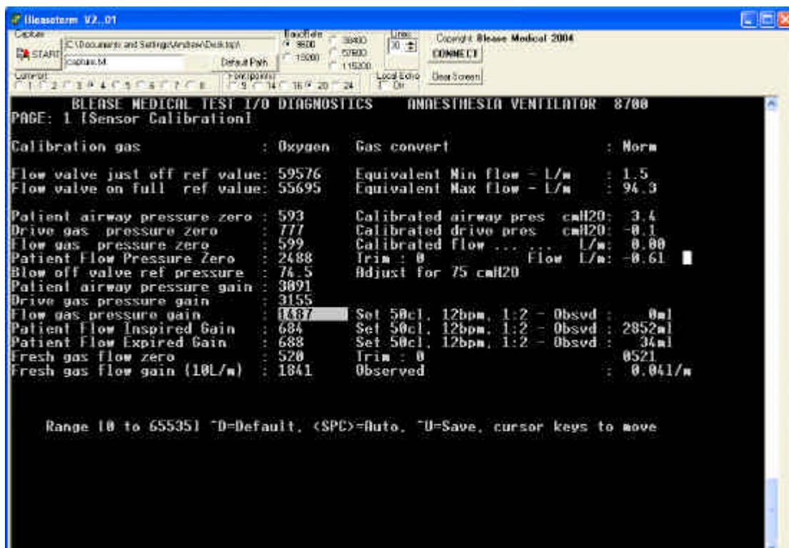
**Figure 47 Delivered Volume Calibration**
