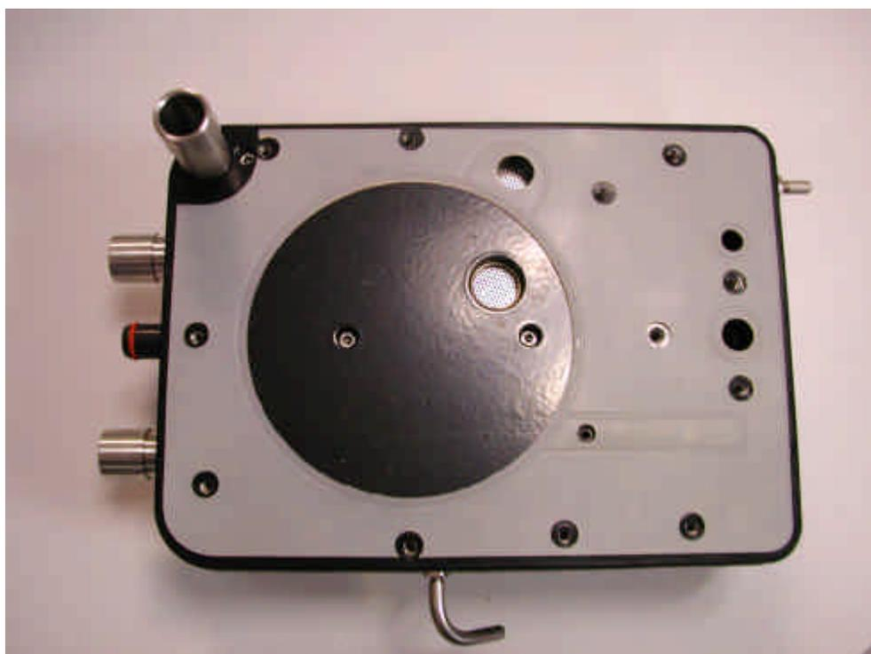
Remove gasket to expose the 15 M4 screws which hold the top moulding to the centre plate.
