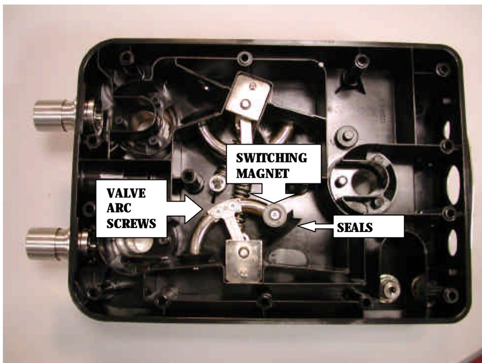
To replace seals remove the two M3 screws from the valve arc.
