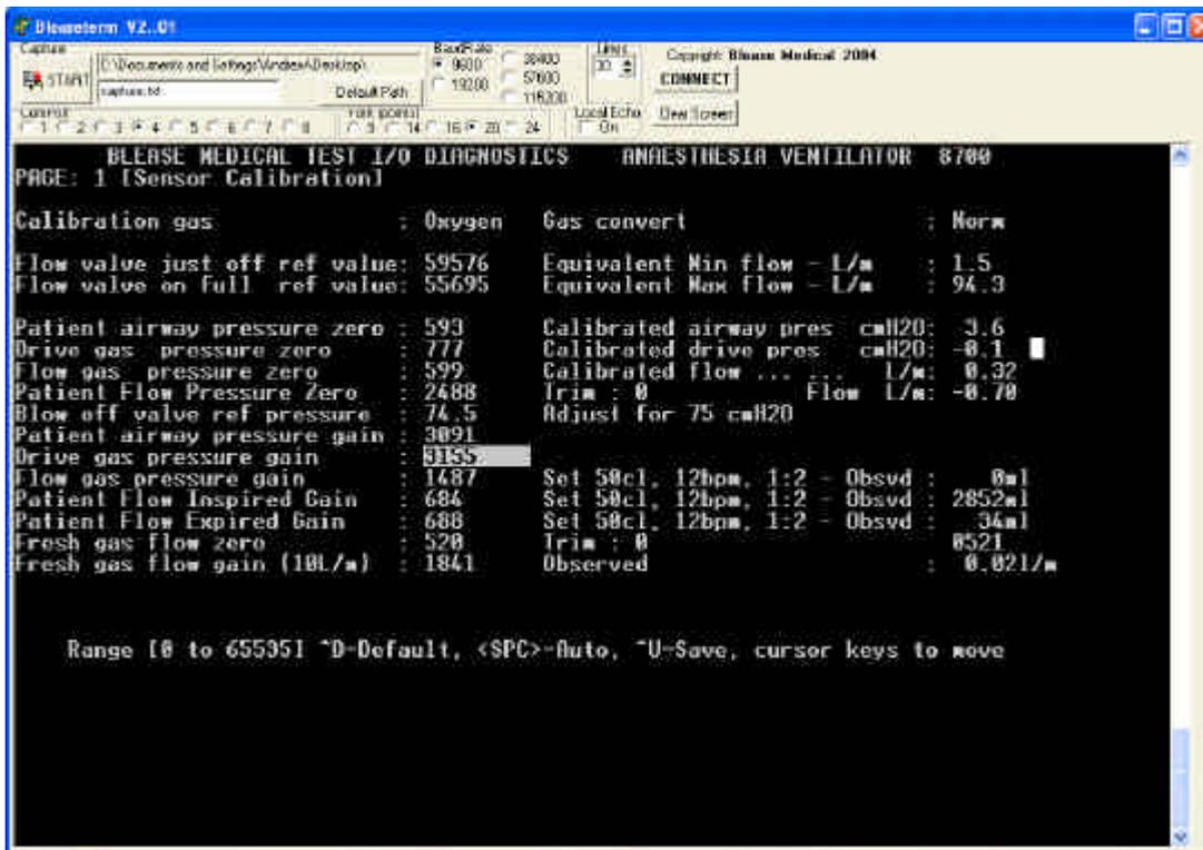
Check the pressure is still 75 +/- 3cmH2O and press the space bar to record the value.
