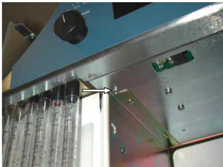
From the rear of the unit remove the drive gas hose, the exhaust (do not unscrew or move the locating ring) and patient sensor tubing making a note of which tube comes from which connector then, remove the four screws for the “D” connectors and the top drive gas fitting.
