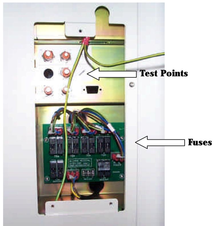
**Figure 11 Part rear Panel Removed**
