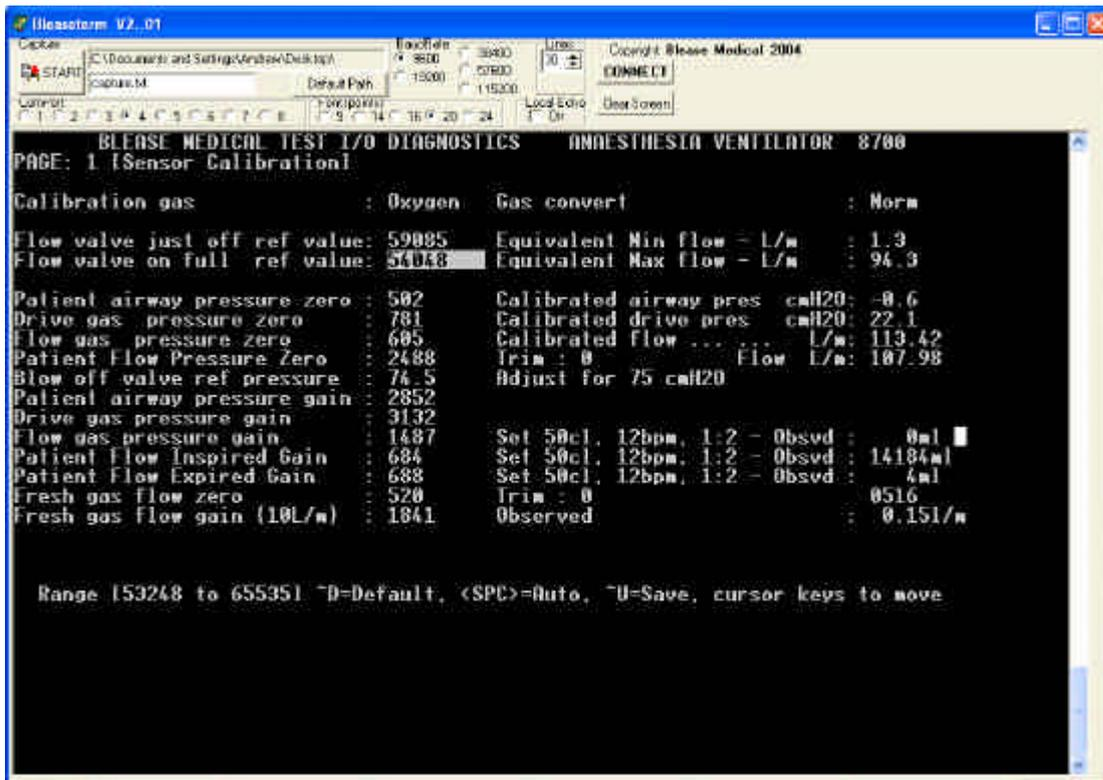
Move cursor to Equivalent Max flow L/M and type in the value recorded on the flow measuring device.
