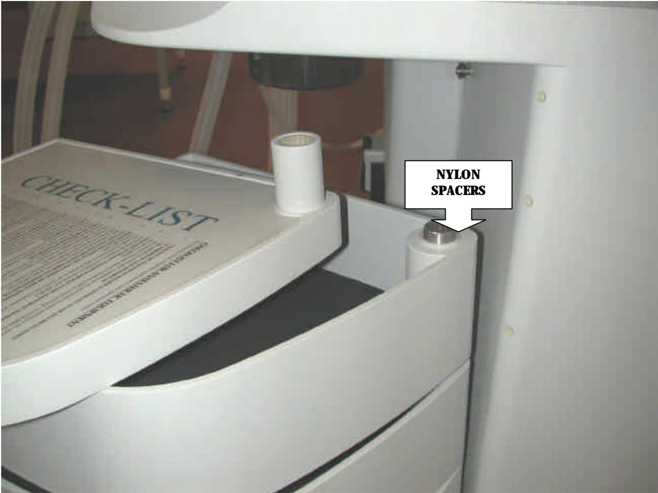
The drawer pole and two collars can then be lifted out of the machine base.
