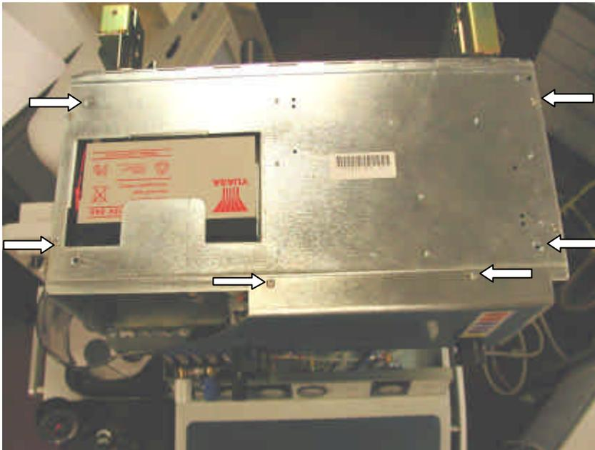
The front of the ventilator will now hinge forward a little to allow the top to open up.
