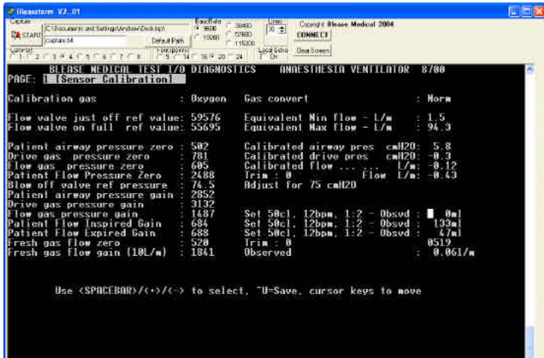
Figure 41 BleaseTerm Sensor Calibration
