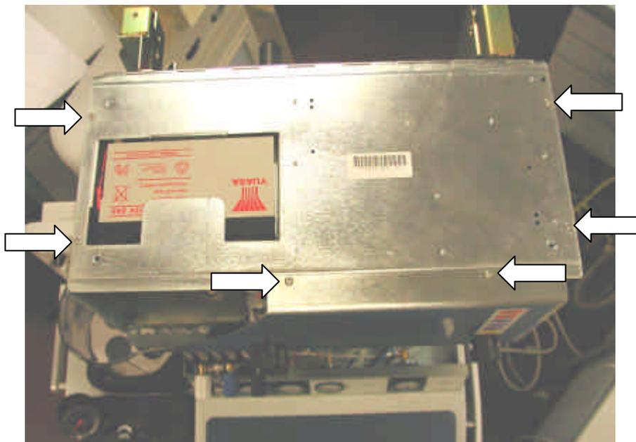
**Figure 38 Ventilator Case Top**
