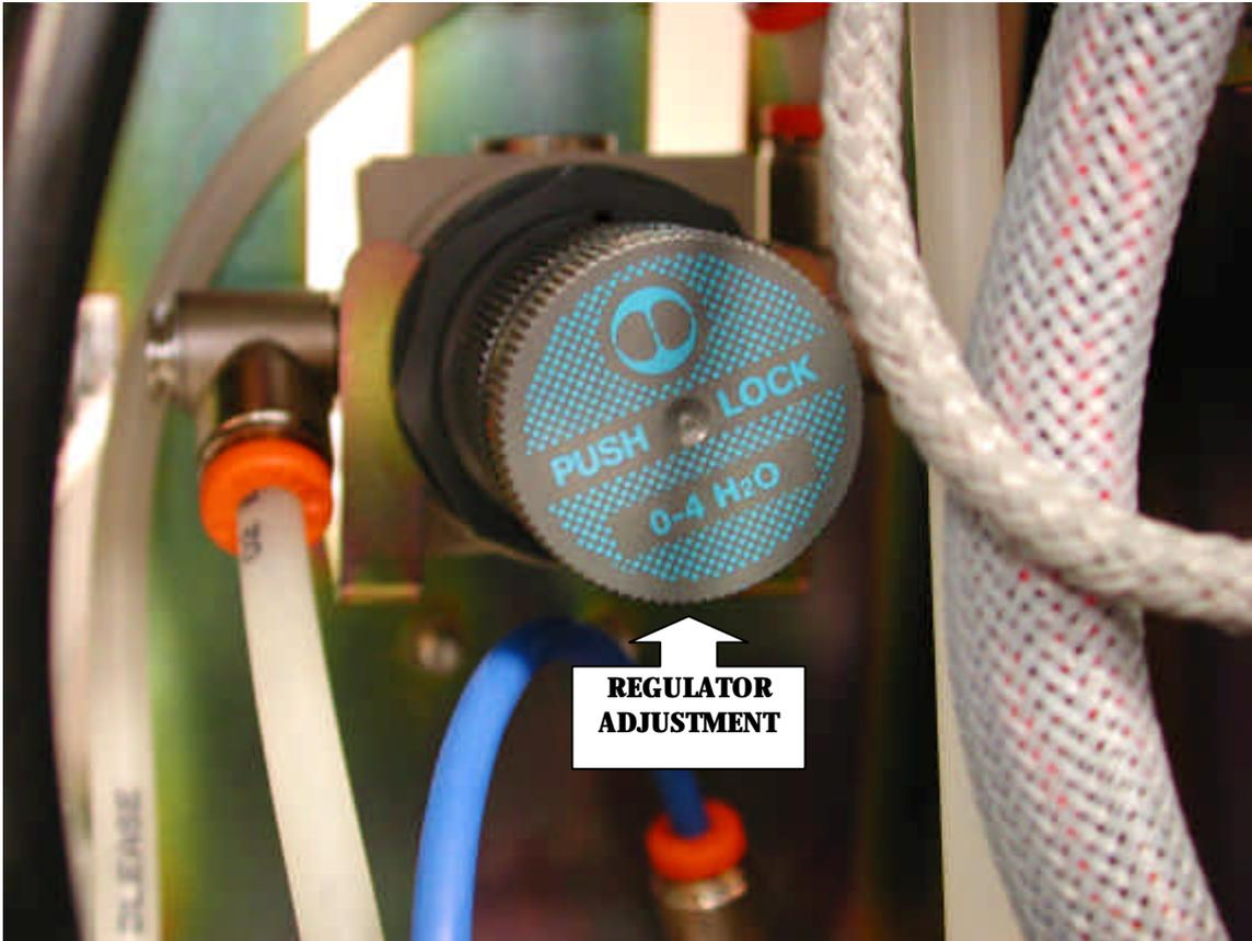
**Figure 19 Regulator Adjustment**
