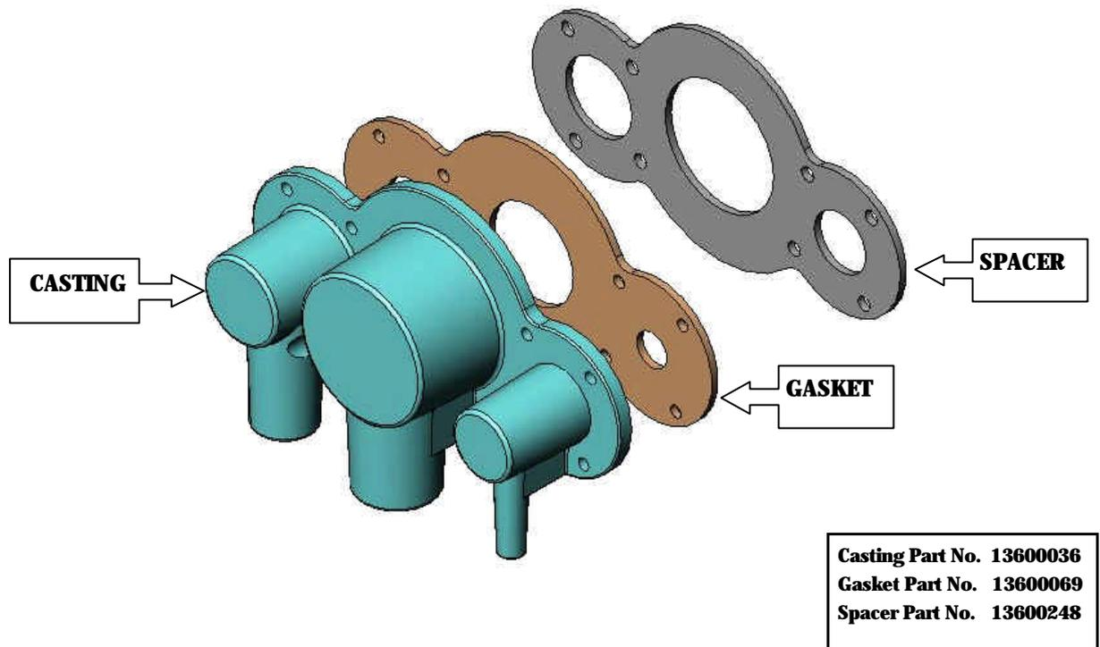
**Figure 30 Absorber Interface Manifold Assembly**
