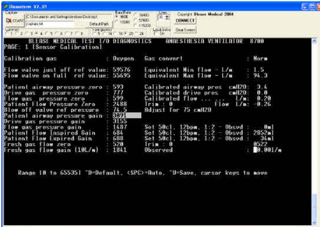
With the blow off pressure at 75 +/- 3 cmH2O press the space bar to record the value. Move the cursor to Drive gas pressure gain.
