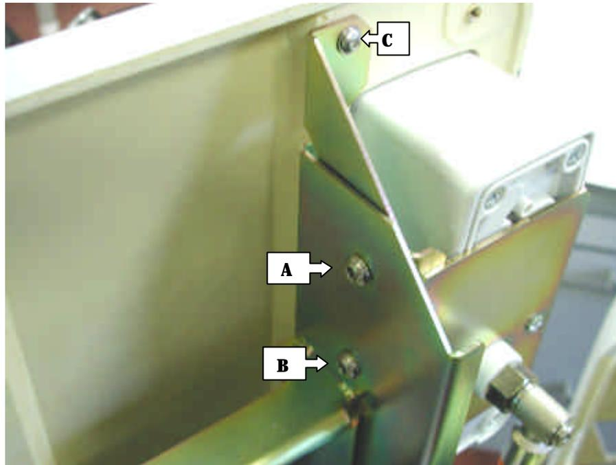
**Figure 36 Suction Controller Removal/ Replacement**
