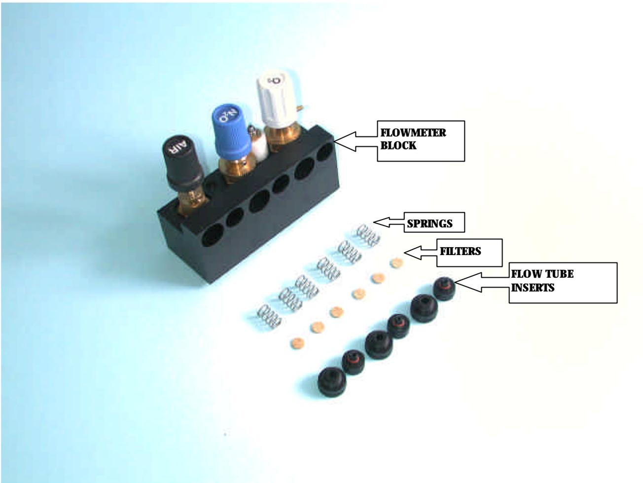
**Figure 15 Flow Block Showing Flow Tube Filters and Tube Lower inserts**
