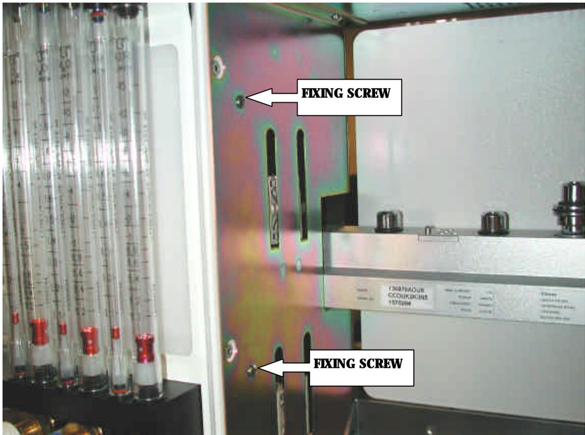
**Figure 28 Flow Meter Removal**
