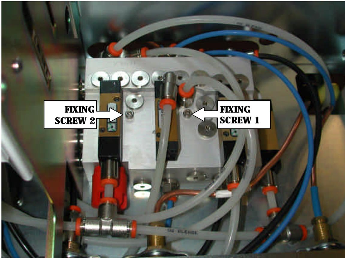
**Figure 25 Alarm Block Removal**
