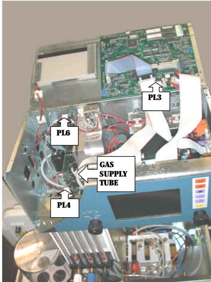
**Figure 39 Inside Ventilator**
