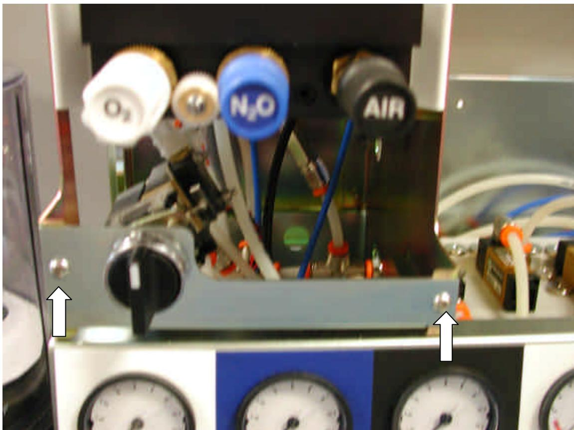
**Figure 29 On/Off Switch Removal**
