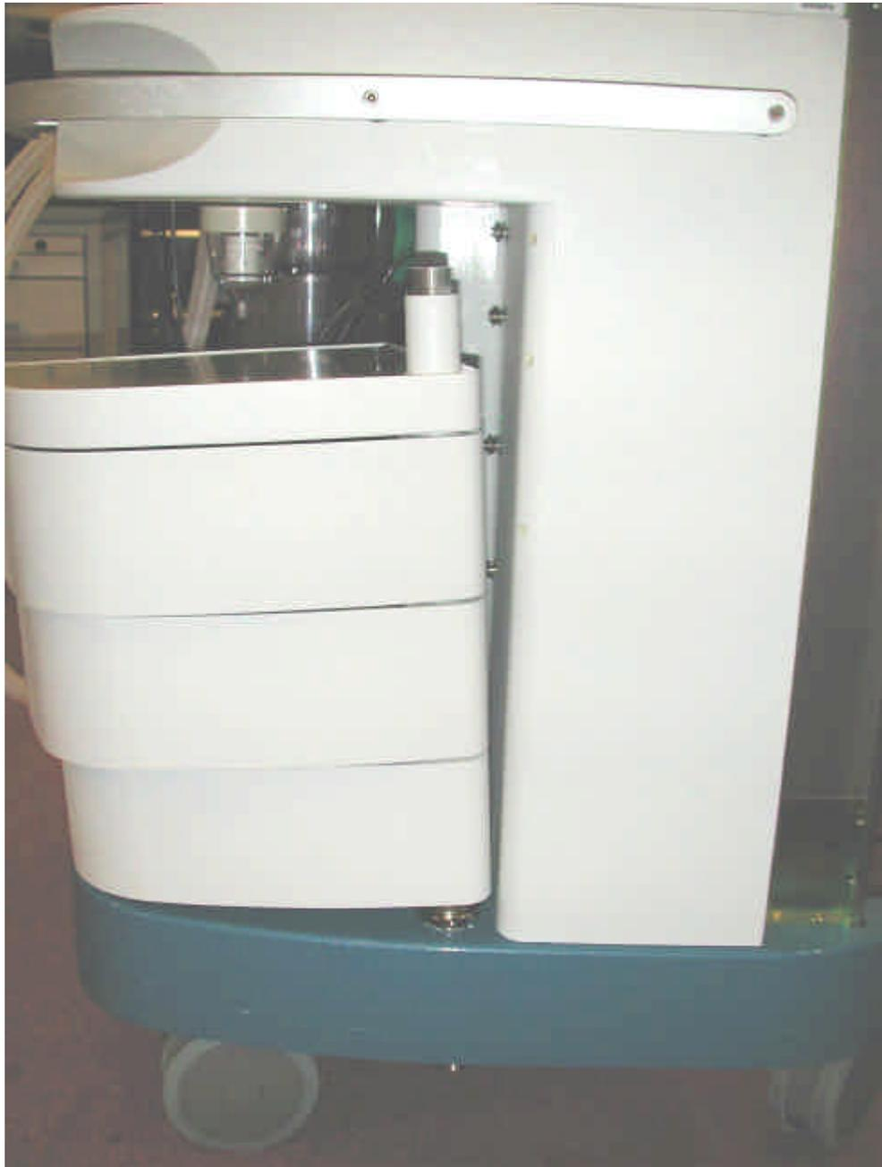
The writing surface and drawers can then be lifted off the pole in turn, taking care not to lose the nylon spacers between each.
