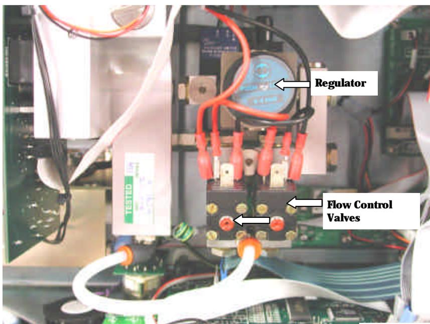
**Gas Inlet Assembly Part No. 13700003**
