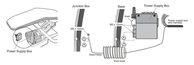
(4) Attach the connectors onto the LED light control PCB of the power supply box.
