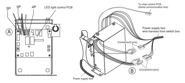
(5) Connect the power supply wire from power supply box to the connector on the metallic box inside the junction box.
