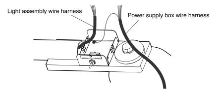
(2) As illustrated below, place the wire harness inside the guide. The part with the cable tie should be inside the box. Lead all the wires underneath the switch, and connect the connectors (3 pins) from the power supply box wire harness and the mode selection switch. See [4] Wiring diagrams.
