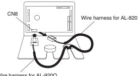
Wire harness for AL-920Q from LED light power supply box (Serial communication line)
