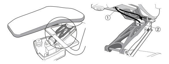
(3) Attach the power supply box by the motor pump of the chair with two M5 x 12mm screws.
