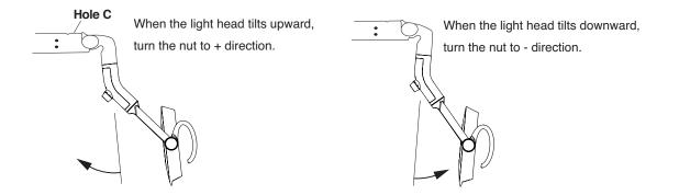
3) After adjustment is done, re-tighten the socket screw.
