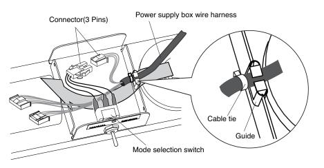
(3) As illustrated below, place the Light Assembly Wire Harness inside the cable guide. The part with the cable tie should be inside the box. Make sure that the Light Assembly Wire Harness should be above that from the power supply box.
