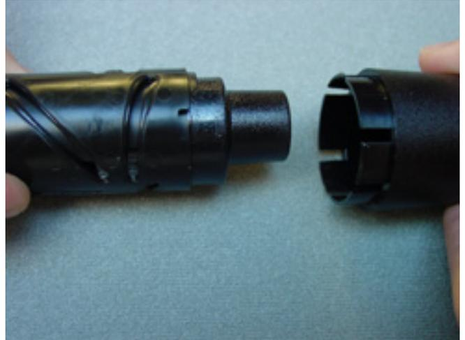
F. Slide the front body over the assembly. You may have to rotate the front body. The front body will snap in place.
