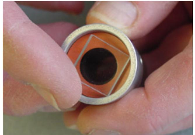
C. Remove the heat filter gasket.
