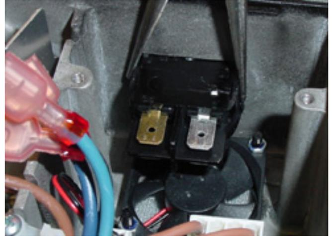
*NOTE: Notice the orientation of the switch when properly installed.*
