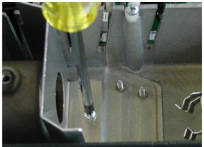
7. Light Pipe Connector Assembly Removal
