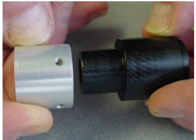
F. Remove the brake from the inside of the insulator.
