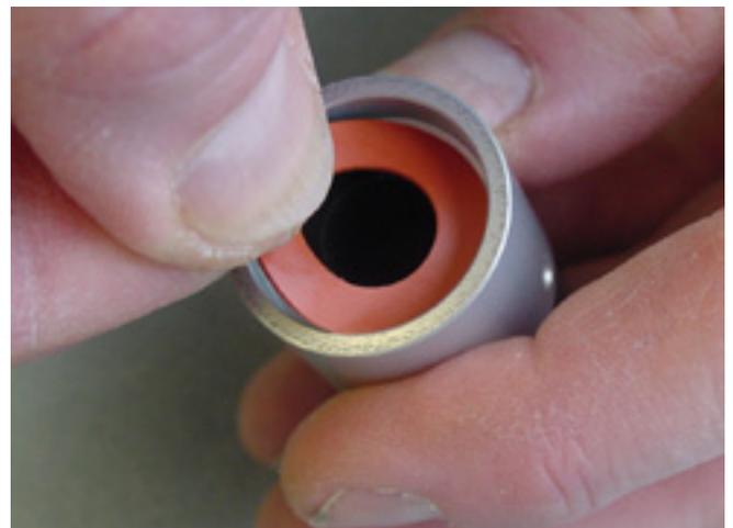
D. Remove the two hex set screws that secure the insulator to the retaining collar.
