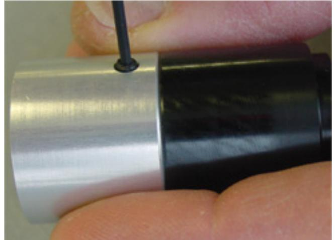
E. Pull the retaining collar from the insulator.
