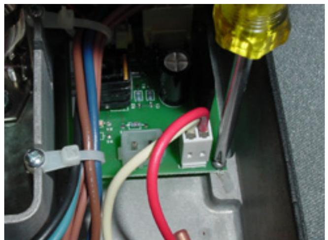
**12. Light Pipe Connector Assembly Disassembly.**
