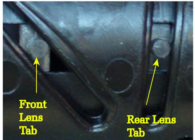
*Note: Observe that each cam sleeve has a slot at the rear of the cam sleeve. The slot must face toward the rear of the assembly.*
