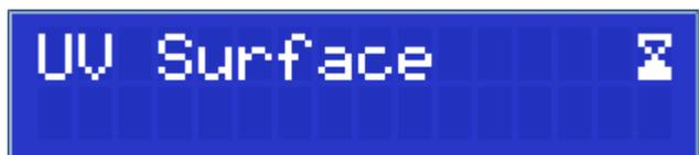
**After replacing UV light tubes it is necessary to reset the hours of duty in the software manually!**
