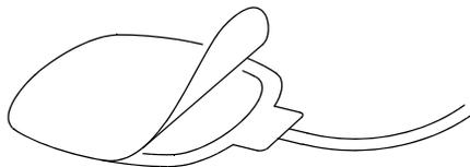
**Figure 5-2** Peeling the Liner from the Electrode
