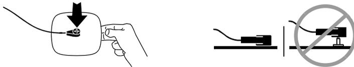
Figure 5-4 Connecting FAST-PATCH Electrodes to Defibrillation Cable
