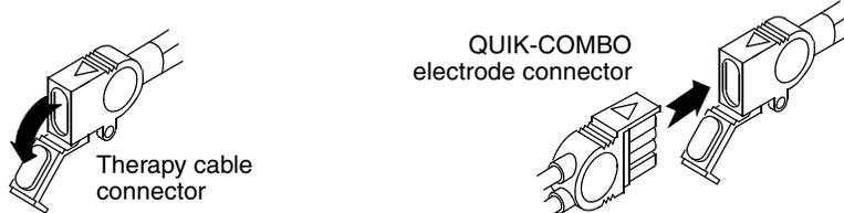
Figure 5-3 Connecting QUIK-COMBO Electrodes to Therapy Cable
