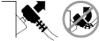
Figure 5-7 Disconnecting Defibrillation Cable from Test Post
