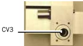
CV3 prevents the patient from exhaling through the inspiratory limb during a safety valve open condition, which prevents the patient from rebreathing exhaled gas.
