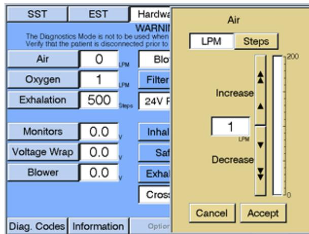
Figure 8-15: Diagnostic Mode - Setting Air Flow
