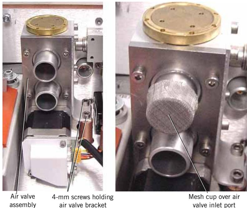
Figure 9-80: Air Valve and Mesh Cup
