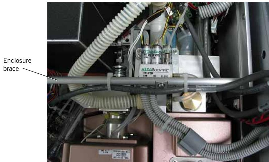
Figure 9-64: Enclosure Brace
