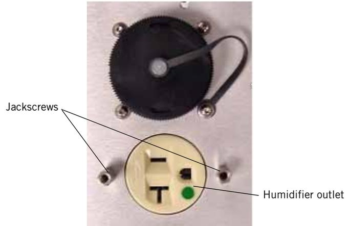
Figure 9-51: Removing AC Receptacle Jackscrews
