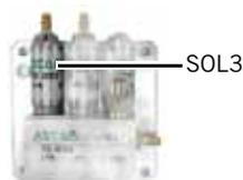
The exhalation pressure transducer solenoid periodically vents the exhalation pressure transducer to atmosphere and measures zero (atmospheric) pressure. Periodically autozeroing the transducer allows it to correct the slight zero voltage drift that can occur over time, and improves overall pressure measurement accuracy.
