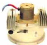
The blower draws room air through the air inlet filter and outputs the air that is delivered to the patient, and provides the pilot pressure that can actuate the safety valve. The blower contains a DC motor and a series of stator and impeller assemblies. It can provide at least 200 LPM of flow.
