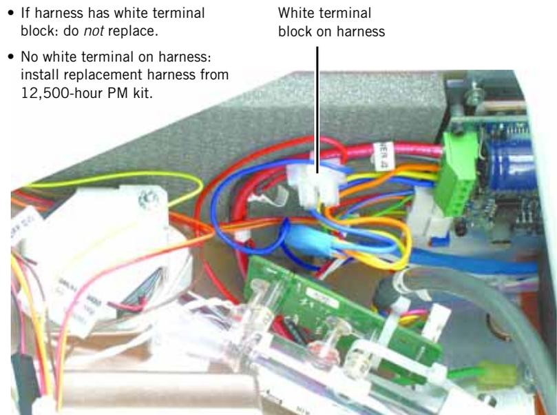
Figure 4-1: Power Supply to Blower Motor Harness Versions
