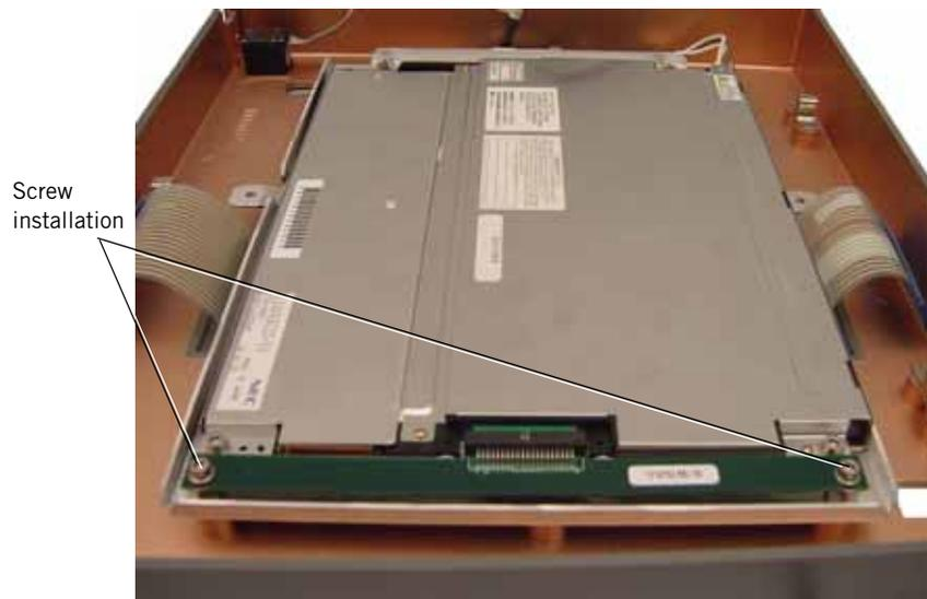
Figure 9-101: Installing the Transition PCB
