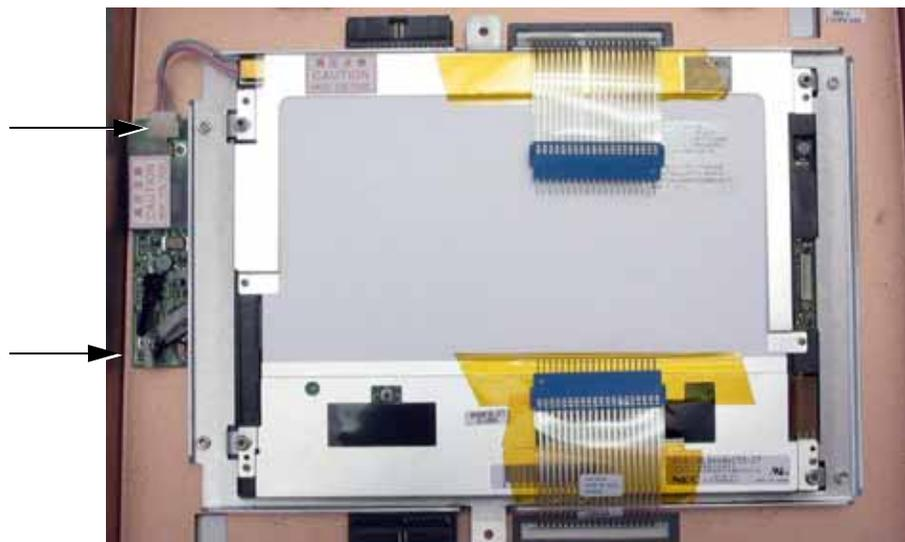
Figure 9-98: Removing the Backlight Inverter
