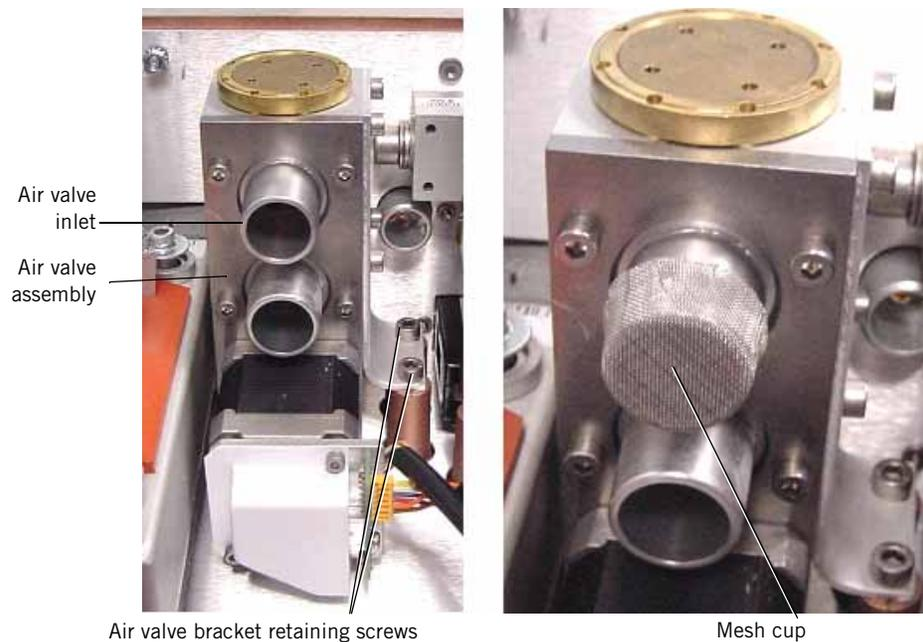
Figure 10-50: Air Valve and Mesh Cup
