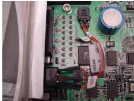
Figure 10-36: Remote Alarm Jack (Inside View)
