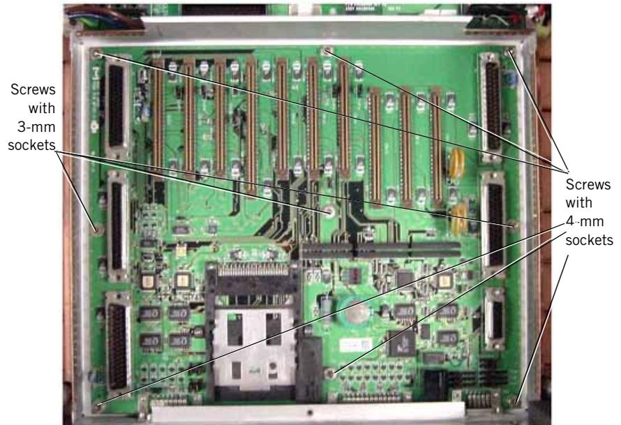
*Figure 10-34: Nine Screws That Secure Main PCB to Tray*
