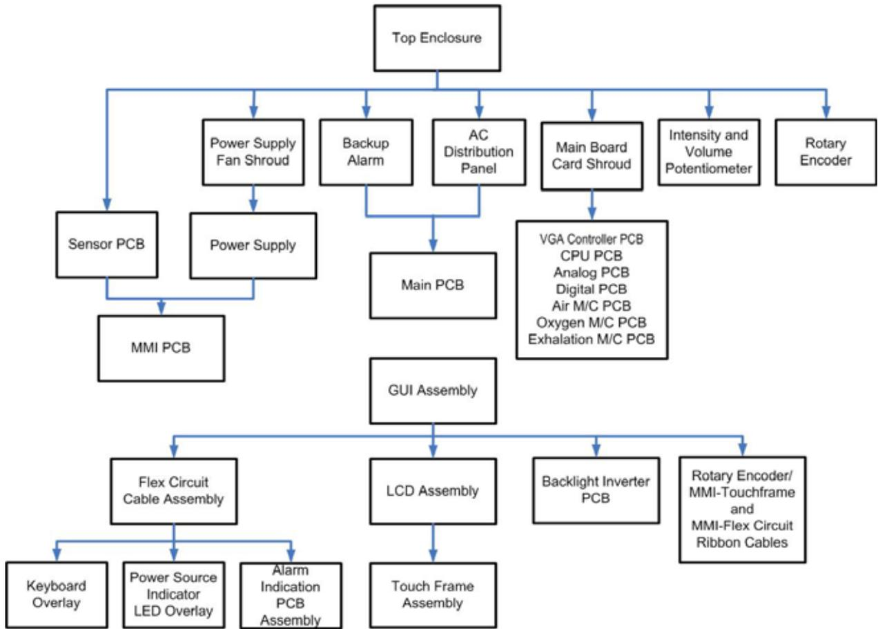
Figure 10-2: Respironics V200 Ventilator Top Enclosure Disassembly Flow Chart
