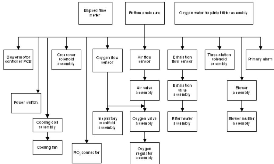
Figure 9-3: Bottom Enclosure Disassembly Flow Chart
