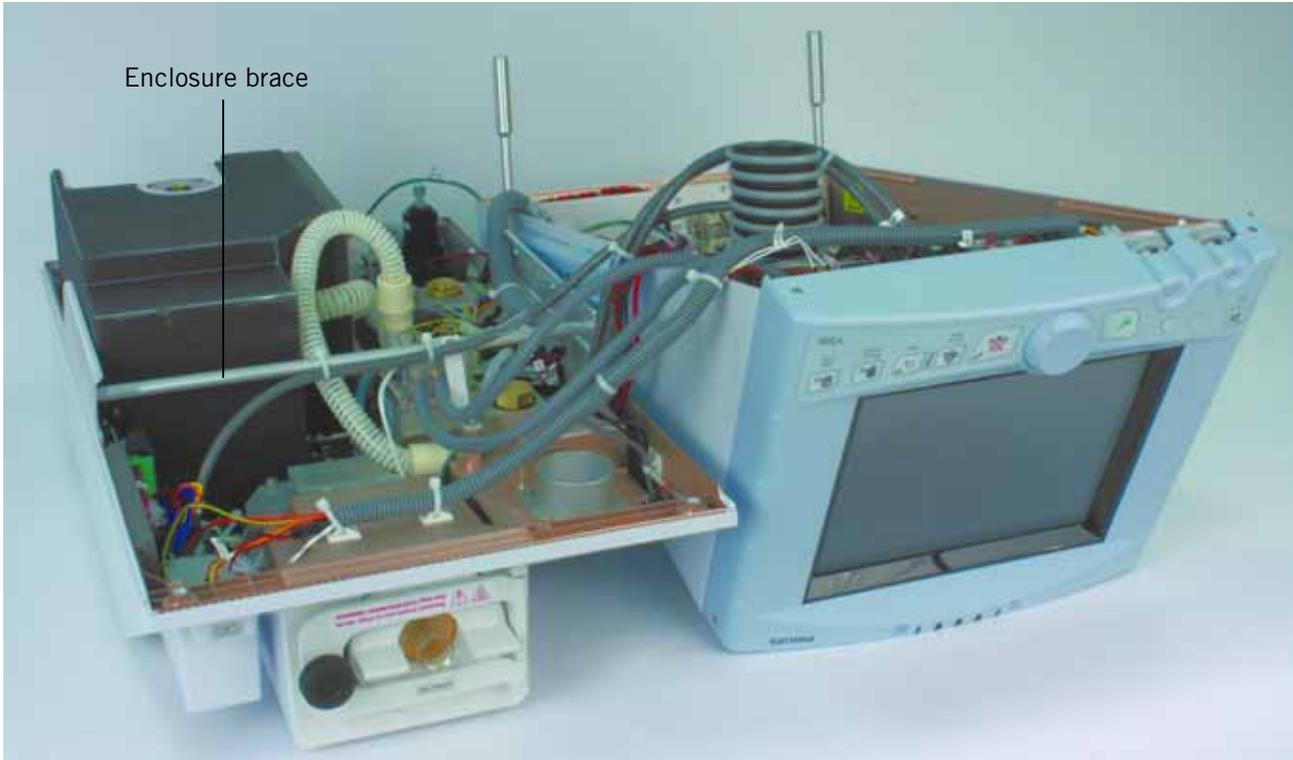
Figure 10-14: Enclosures Separated
