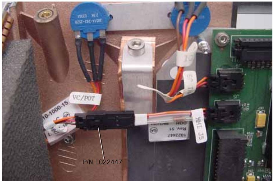
Figure 9-43: Increased Alarm Volume Harness
