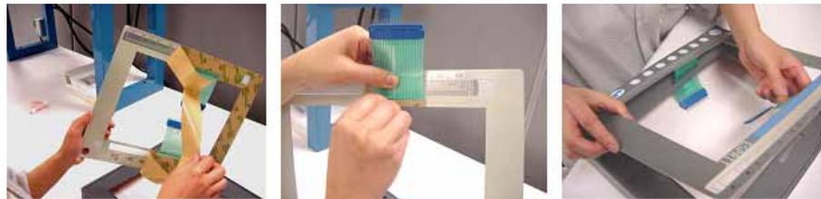
Figure 9-33: Installing GUI Front Panel Overlay (10.4-in. GUI)
