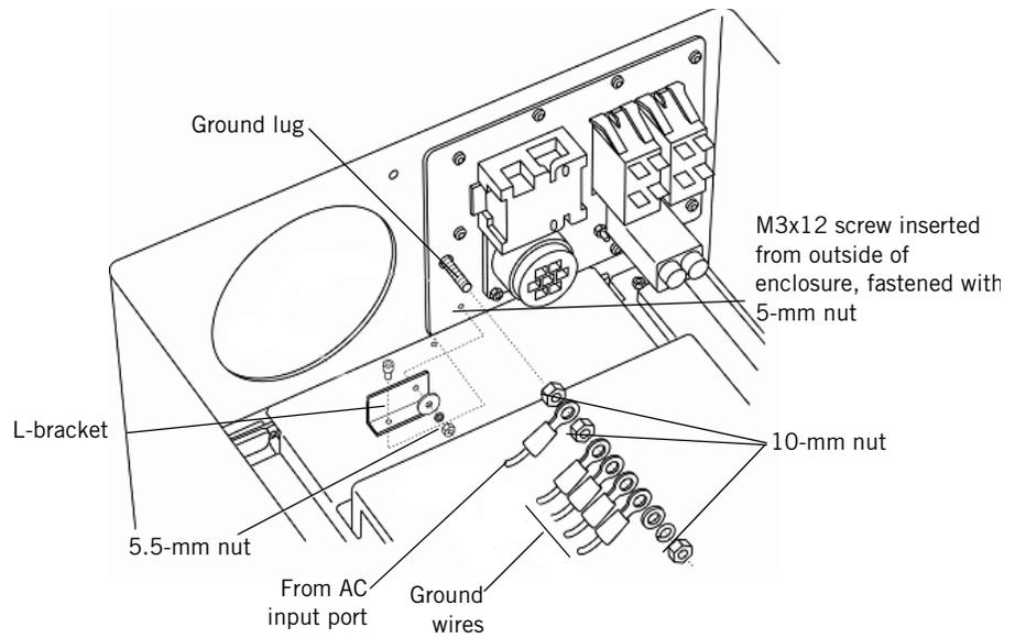
Figure 10-27: AC Distribution Panel (From Inside the Enclosure)
