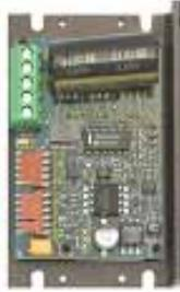
The blower motor controller PCB controls the speed of the blower motor based on analog input conditioned by the sensor PCB. It includes a lockup sensing circuit, which monitors sensors in the blower motor to detect a locked rotor condition. If the blower motor stops running, the lockup sensing circuit shuts off power to the blower.
