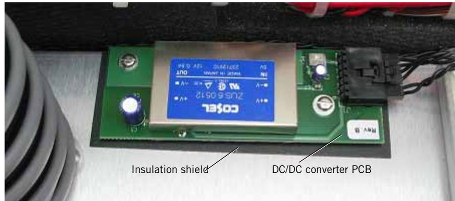
Figure 9-95: Adhesive-Backed Insulation Shield on Power Supply Shroud
