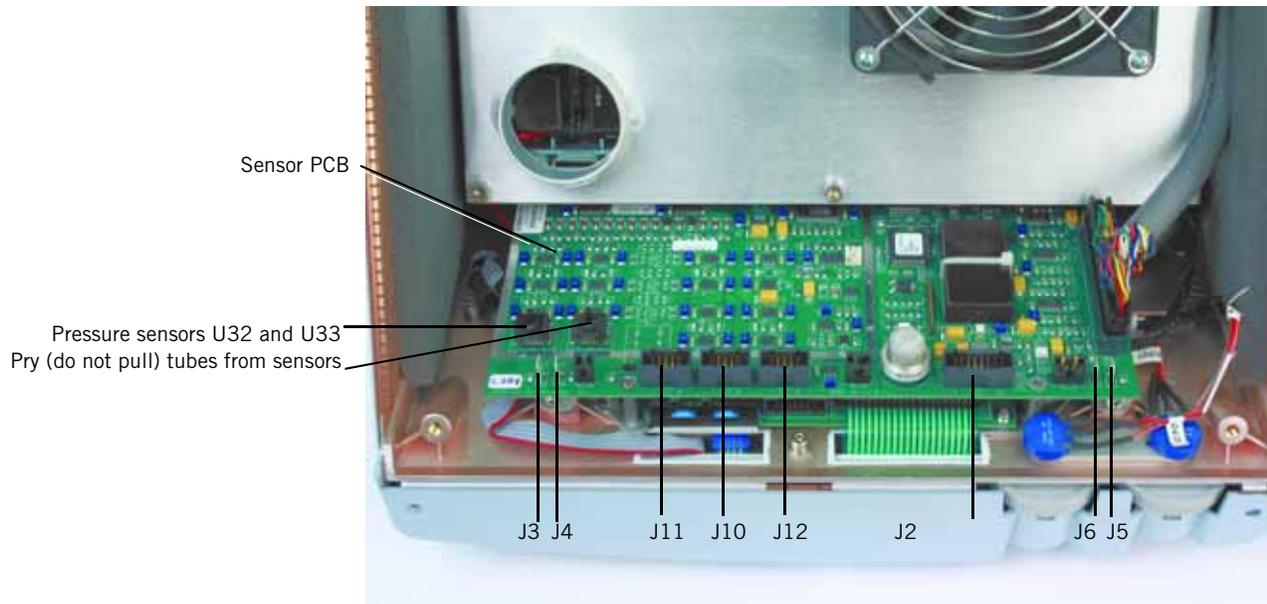
Figure 10-16: Sensor PCB
