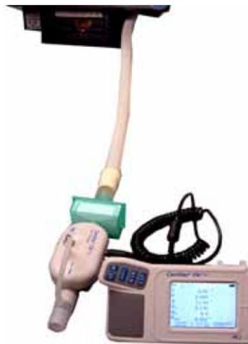
Figure 5-10: Flow Sensor Troubleshooting Setup
