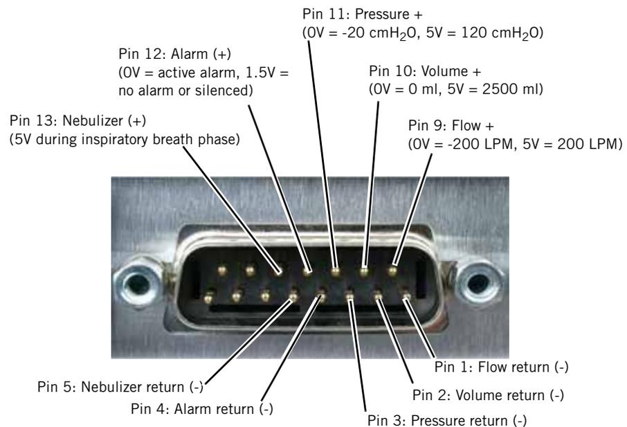
Figure 8-22: Analog Output Port Pinouts
