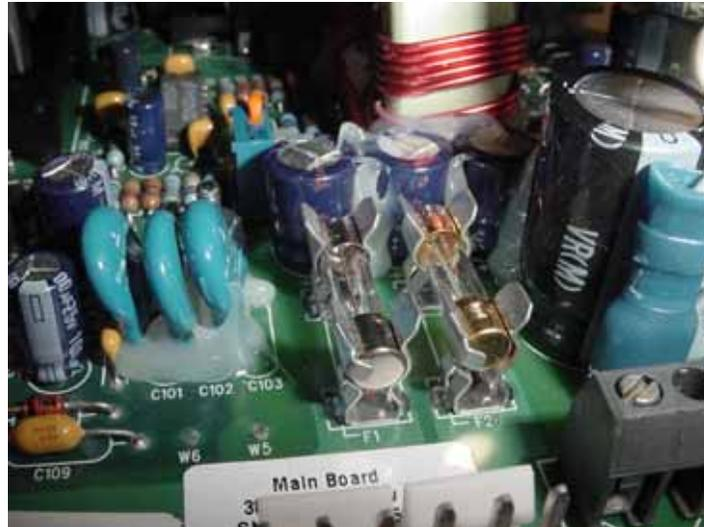
Figure 9-18: Power Supply Fuses (F2 Not Soldered)
