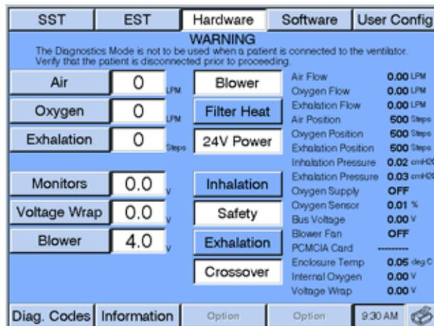
Figure 5-9: Diagnostic Mode - Hardware Screen (Safety Solenoid Energized)
