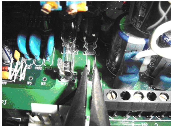
Figure 9-19: Pinch Fuse Clips Together
