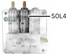
SOL4 periodically vents the inspiratory pressure transducer to atmosphere and makes a measurement at zero (atmospheric) pressure. Periodically autozeroing the transducer allows it to correct the slight zero voltage drift that can occur over time, and improves the overall accuracy of the pressure measurement.
