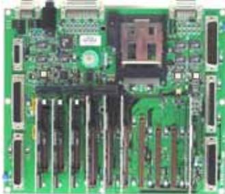
The CPU and other ventilator logic interact through the system data, address, and control buses on the main PCB. The main PCB receives input signals from various keys on the console or touch screen display and sends them to the CPU. The main PCB also contains signal inputs for non-maskable interrupt, running on AC, and running on external battery.
