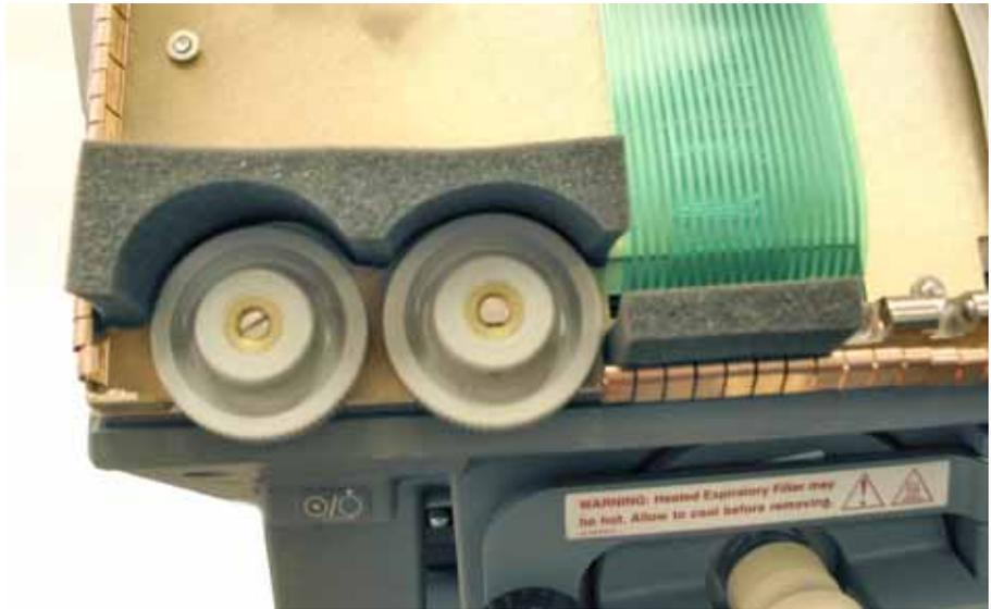
Figure 10-12: Installing the Bulkhead Foam
