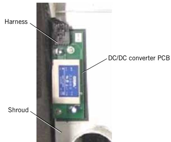
*Figure 9-13: DC/DC Converter PCB Connections (10.4-in. GUI)*
