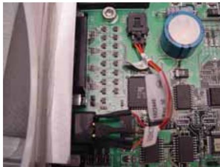
Figure 9-60: Remote Alarm Jack (Inside view)
