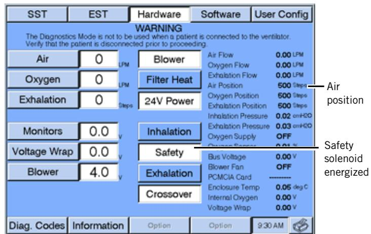
Figure 8-14: Diagnostic Mode - Hardware Screen
