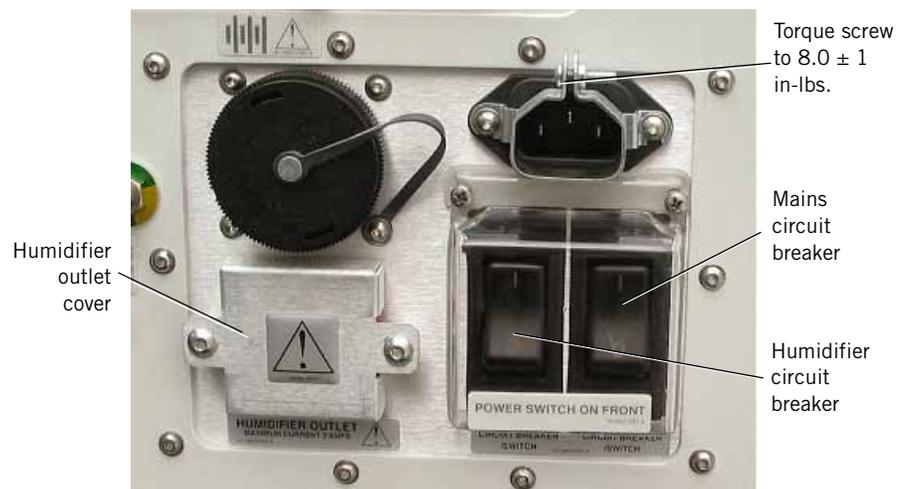
Figure 9-50: Humidifier Outlet Cover
