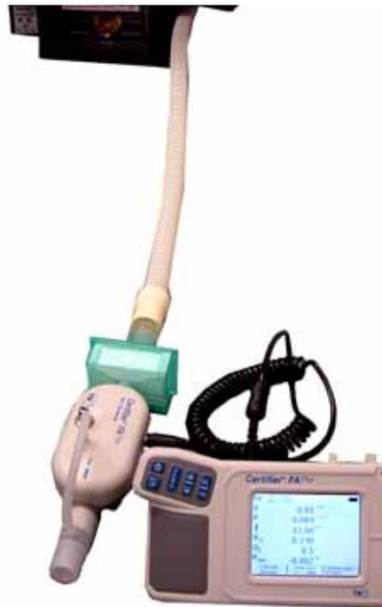
Figure 8-24: Gas Volume Accuracy Test Configuration
