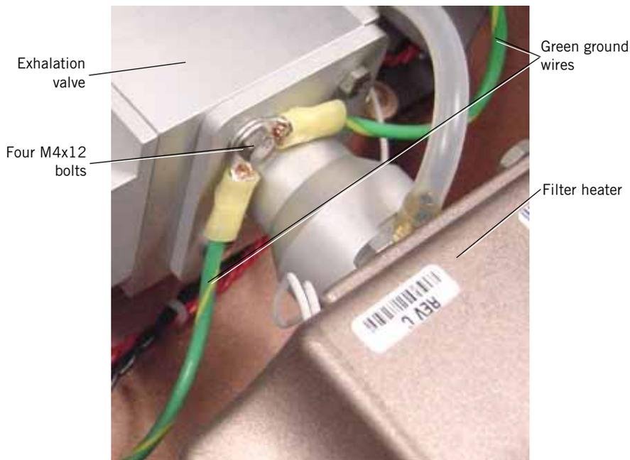
Figure 9-67: Exhalation valve to Filter Heater Connection
