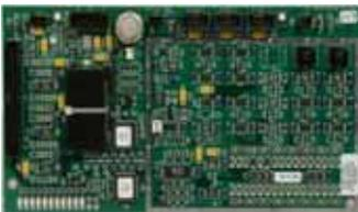
The sensor PCB contains an analog to digital converter (ADC) that converts analog signals from various pneumatic components and the power supply into digital signals for the CPU. Signals include: air flow and temperature, oxygen flow and temperature, exhalation flow and temperature, inspiratory and exhalation pressure, battery voltage, FIO<sub>2</sub>, enclosure temperature, and enclosure oxygen concentration.
