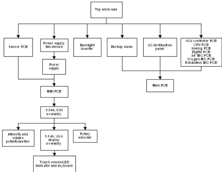
Figure 9-1: Top Enclosure (9.5-in. GUI) Disassembly Flow Chart
