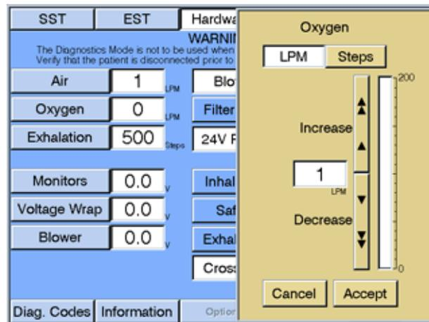
Figure 8-17: Diagnostic Mode - Setting Oxygen Flow
