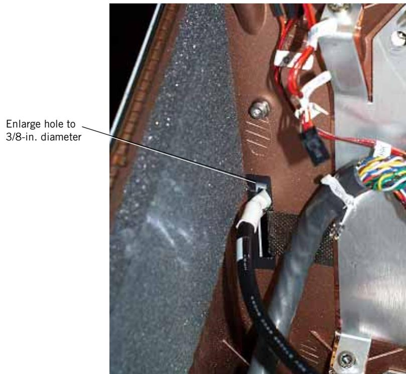
Figure 9-93: Enlarge Hole in Ventilator Enclosure for New GUI Cable
