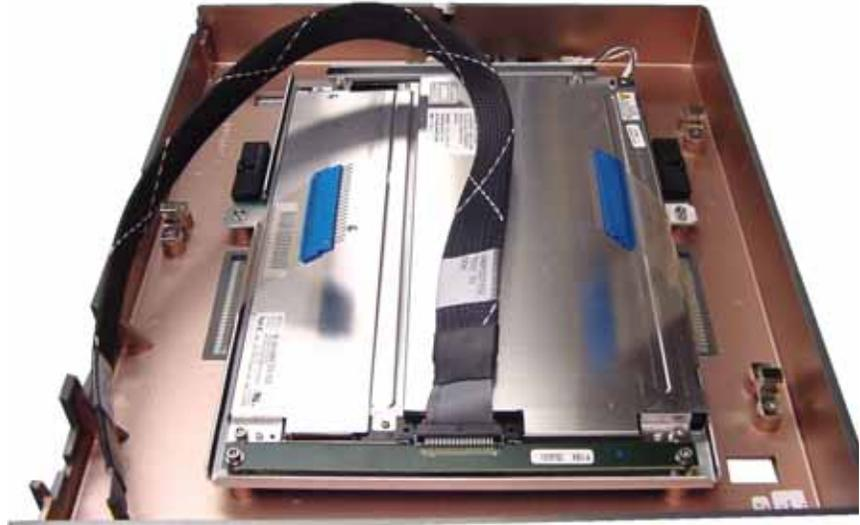
*Figure 9-102: Installing the Color Display Cable*
