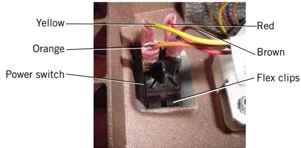
Figure 9-61: Power Switch Wire Connections
