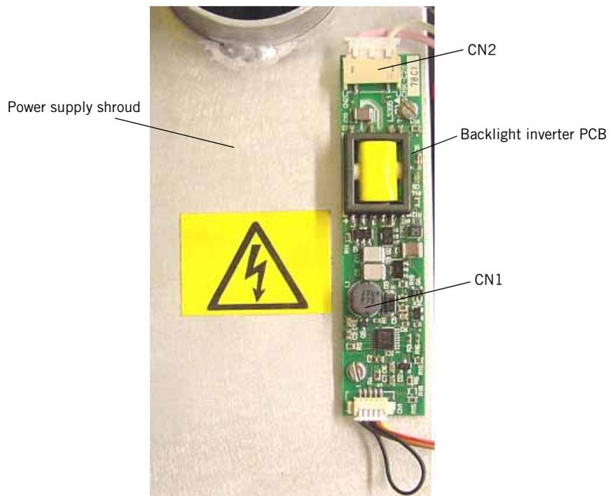
Figure 9-10: Backlight Inverter PCB Connections (9.5-in. GUI)
