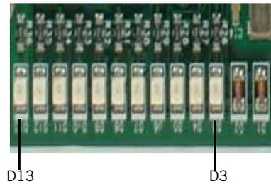
Figure 5-17: Sensor PCB LEDs
