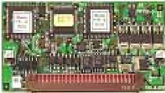
There are three motor controller PCBs for the air valve, oxygen valve, and exhalation valve. The three boards are physically the same and are differentiated by the slot they occupy on the main PCB:
