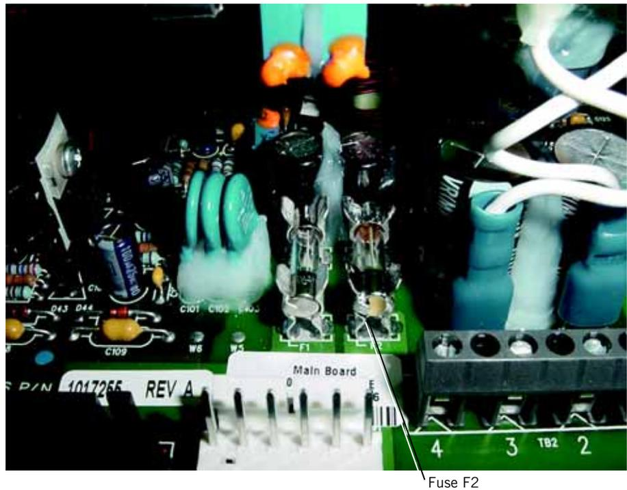
Figure 10-23: Power Supply Fuses (F2 Soldered)
