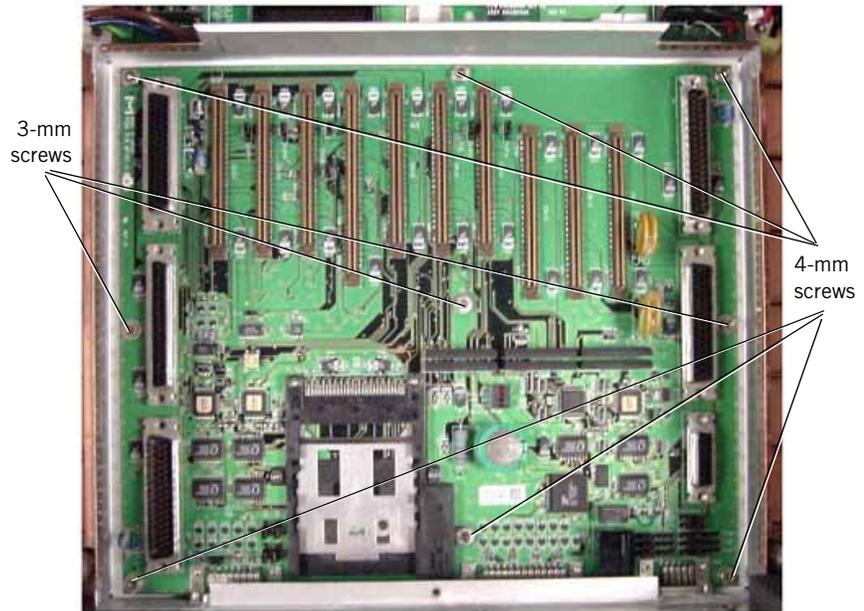
*Figure 9-58: Nine Screws Secure Main PCB to Tray*
