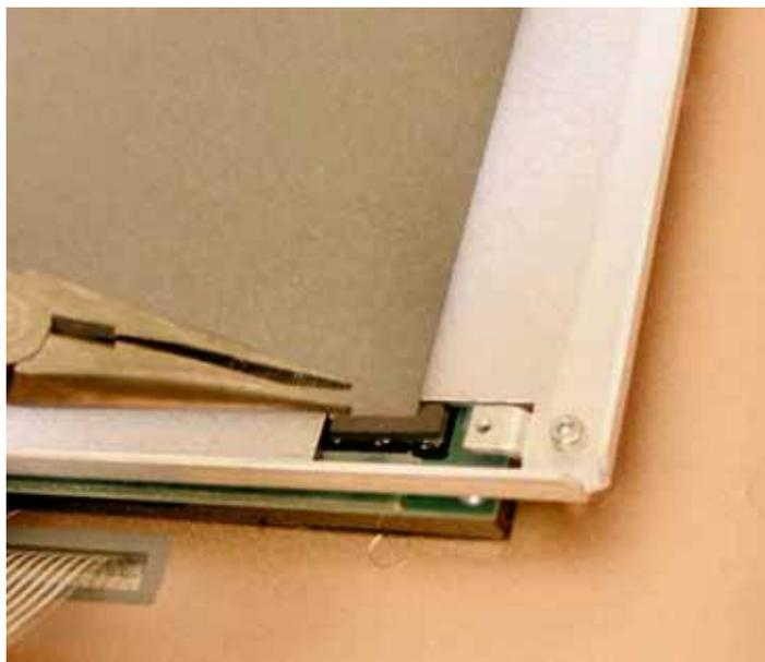
*Figure 9-41: Installing the GUI Dust Gaskets*
