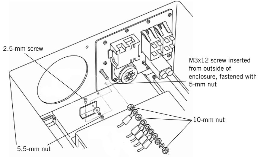
Figure 9-46: AC Distribution Panel (From Inside the Enclosure)
