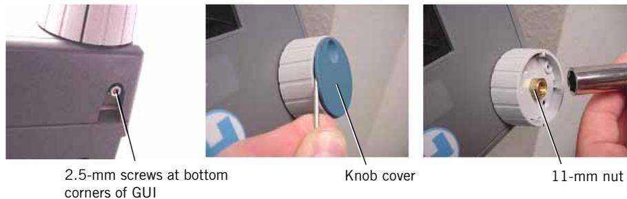
Figure 9-11: Removing/Installing the Rotary Encoder Knob
