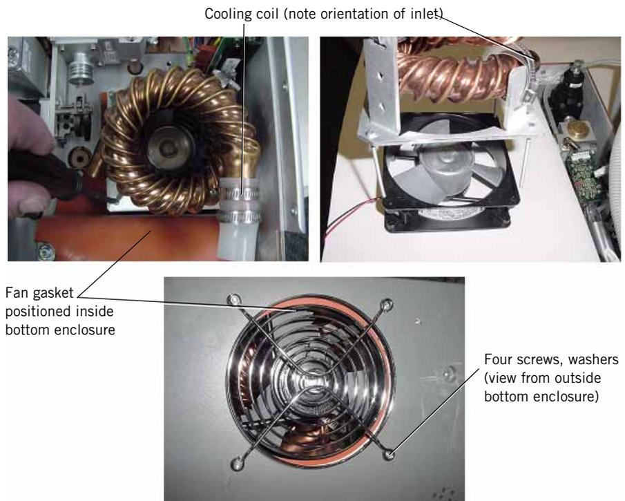
Figure 10-59: Cooling Coil and Fan
