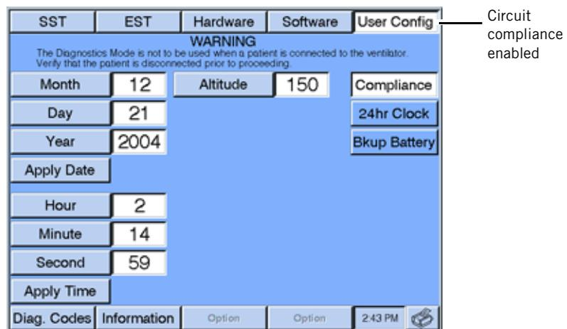
Figure 8-26: User Configuration Screen - Compliance Enabled
