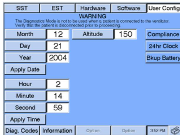
Figure 8-13: Diagnostic Mode - User Configuration Screen
