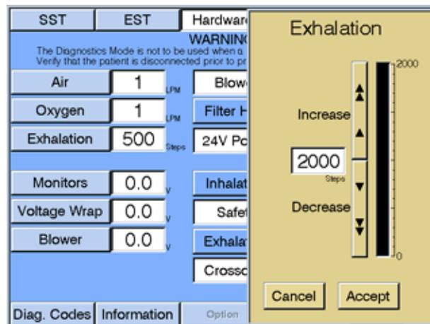
Figure 8-18: Diagnostic Mode - Selecting Exhalation Position
