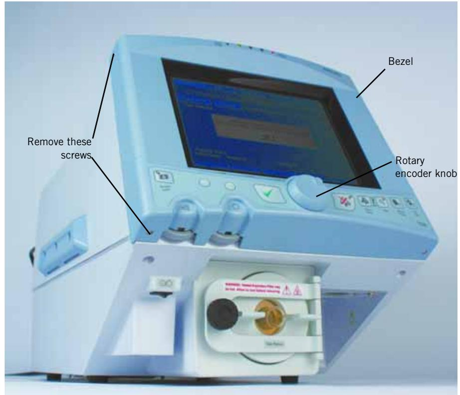
Figure 10-6: Removing GUI - Step 1
