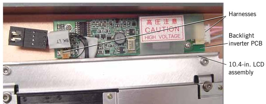
Figure 9-12: Removing/Installing the Backlight Inverter PCB (10.4-in. GUI)
