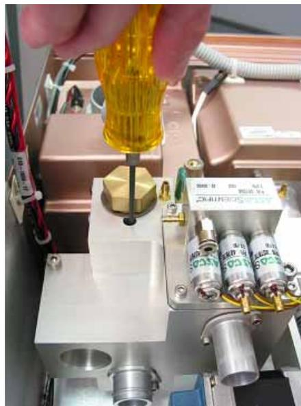
Figure 9-73: Recessed 2.5-mm Set Screw Securing Outlet Port
