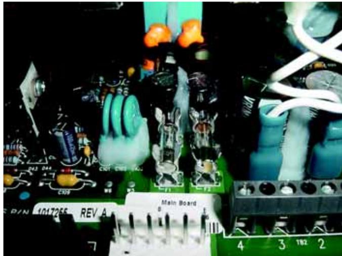
Figure 9-17: Power Supply Fuses (F2 Soldered)
