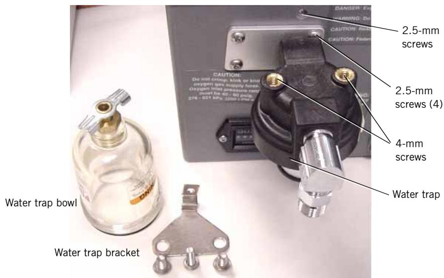
Figure 9-84: Oxygen Water Trap and Oxygen Regulator
