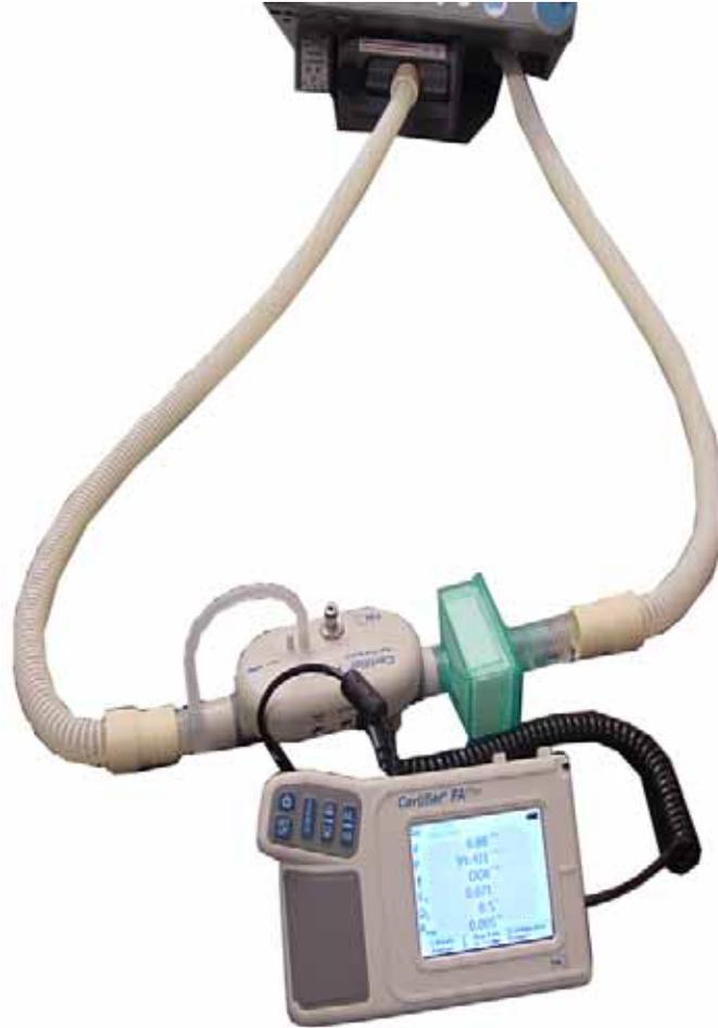
Figure 8-19: Pressure Accuracy Test Configuration
