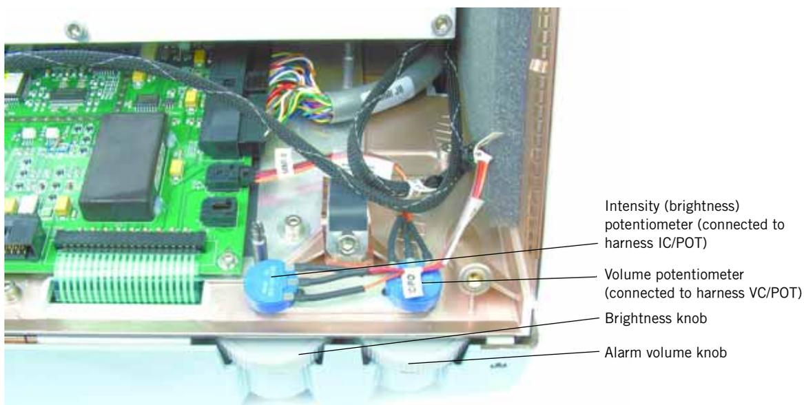
Figure 10-17: Volume and Intensity Potentiometers
