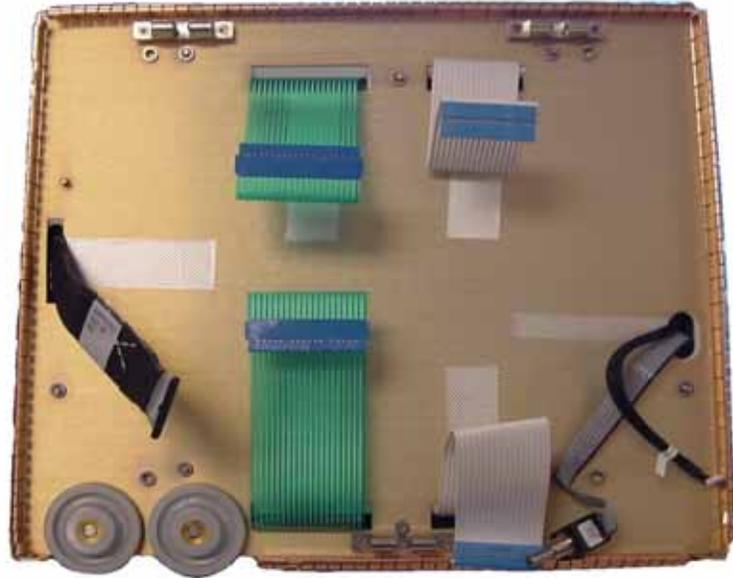
*Figure 9-28: Front of Ventilator with 10.4-in. GUI Removed*
