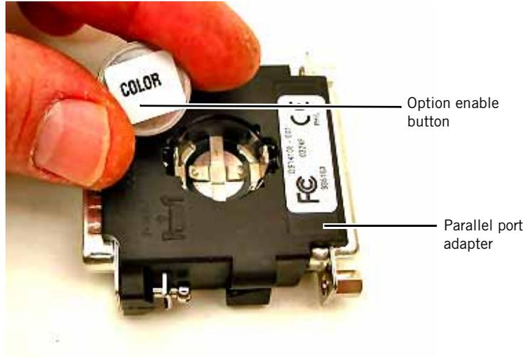
Figure 7-5: Parallel Port Adapter and Option Enable Button
