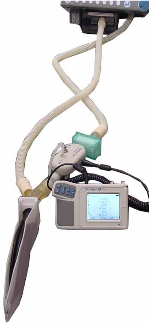
Figure 8-20: PEEP System and Breath Rate Test Setup
