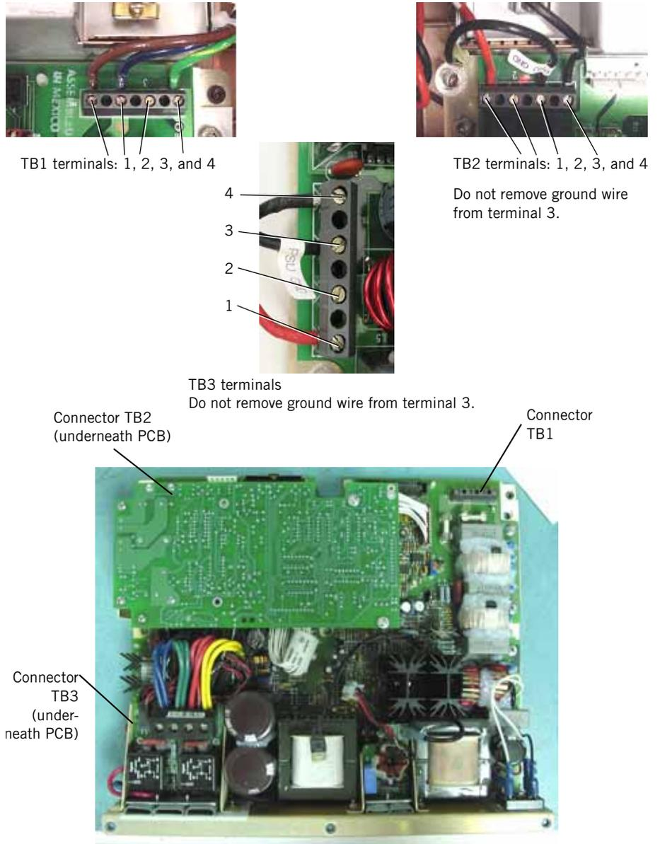
Figure 10-20: Power Supply Wire Connections
