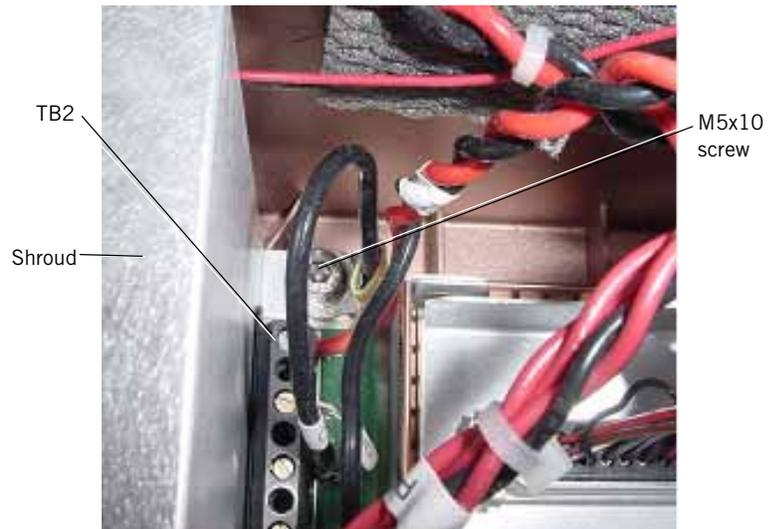
Figure 9-16: Shroud Ground Connection
