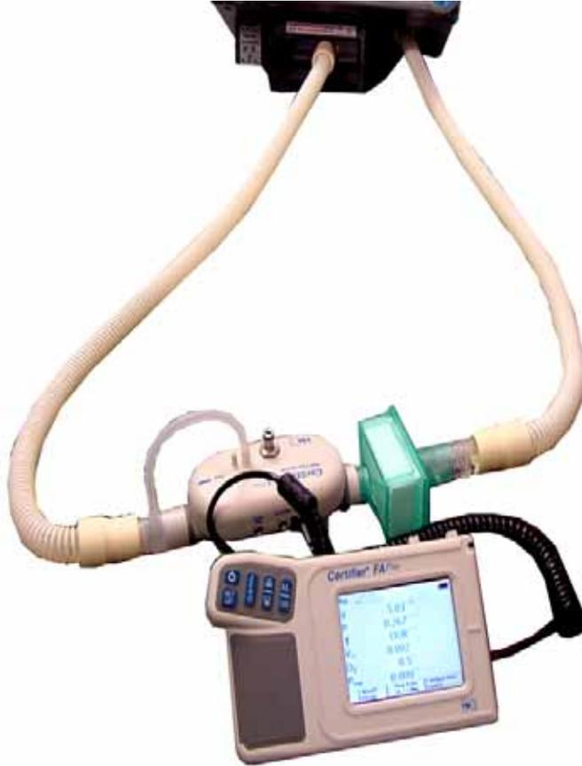
Figure 8-16: Flow Accuracy Test Configuration
