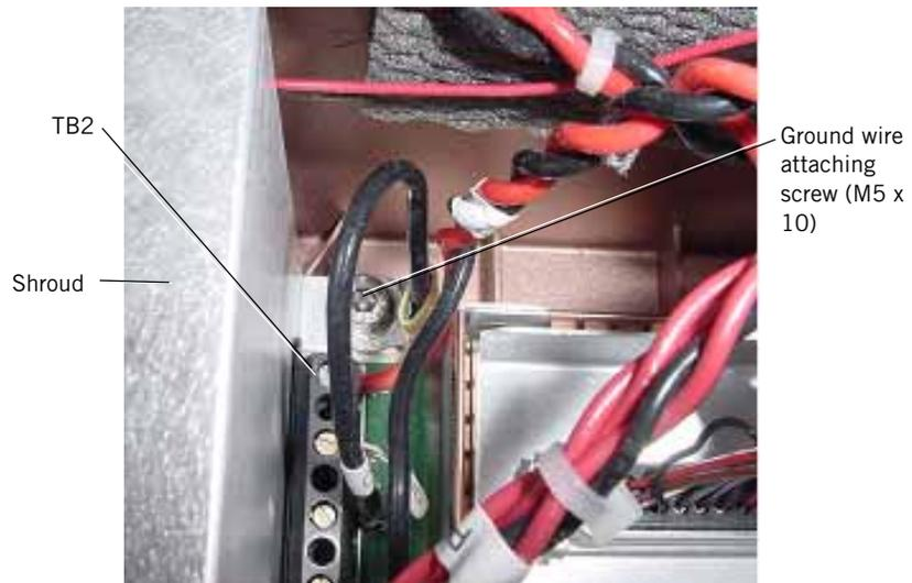
Figure 10-22: Shroud Ground Connection
