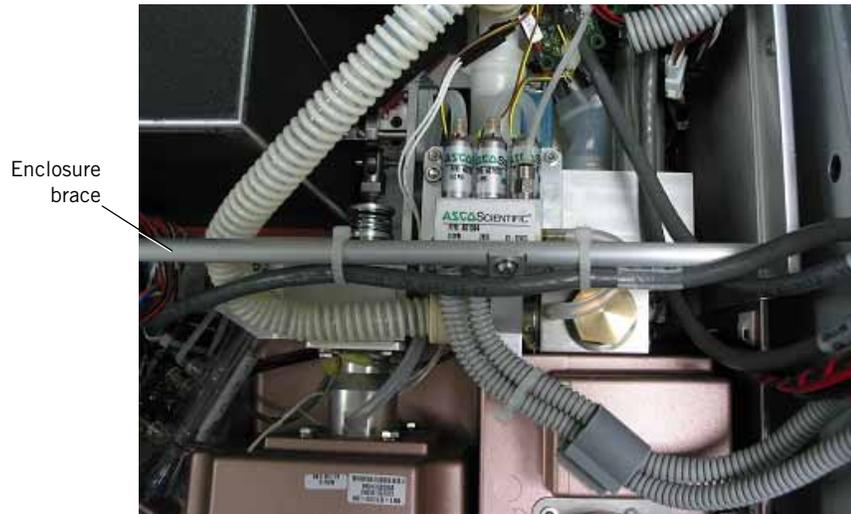
Figure 10-15: Enclosure Brace
