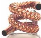
The cooling coil is a copper tube connected to the outlet of the blower dissipate heat from gas leaving the blower before it reaches the air valve.
