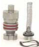
The pressure relief valve provides a backup to the operator adjustable high-pressure alarm and prevents excessive pressures in the patient circuit. The pressure relief valve is spring-loaded to limit the maximum circuit pressure to 130 to 140 cmH<sub>2</sub>O.
