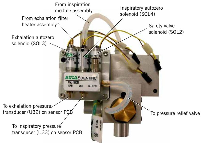
Figure 9-78: Three-Station Solenoid Assembly
