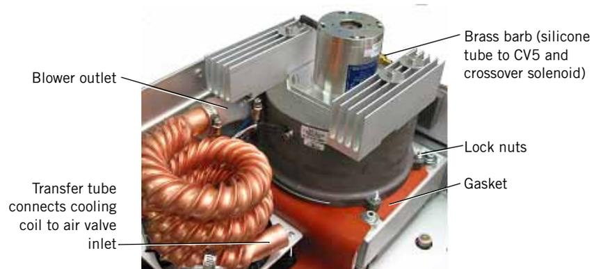
Figure 9-89: Blower Assembly Position on Gasket
