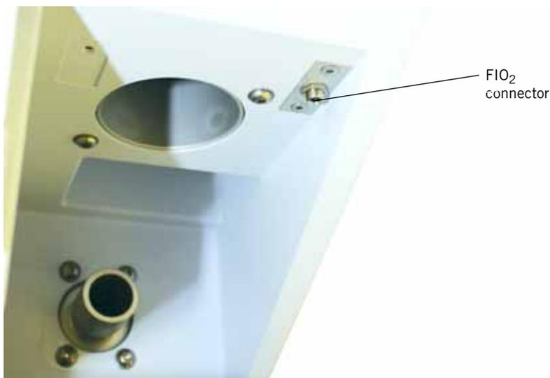
Figure 10-38: FIO<sub>2</sub> Connector
