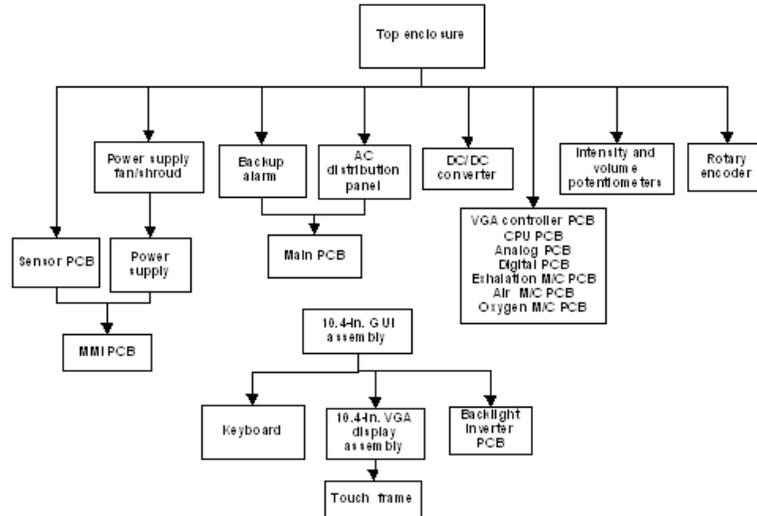
Figure 9-2: Top Enclosure (10.4-in. GUI) Disassembly Flow Chart
