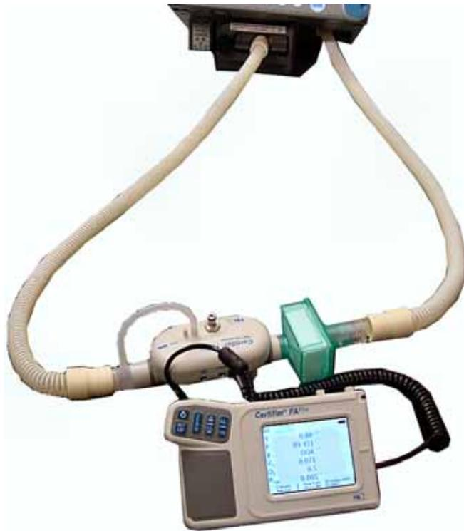
Figure 5-16: Inhalation and Exhalation Pressure Transducer Troubleshooting Setup
