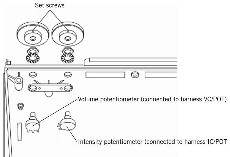
Figure 9-29: Volume and Intensity Potentiometers (9.5-in. GUI)
