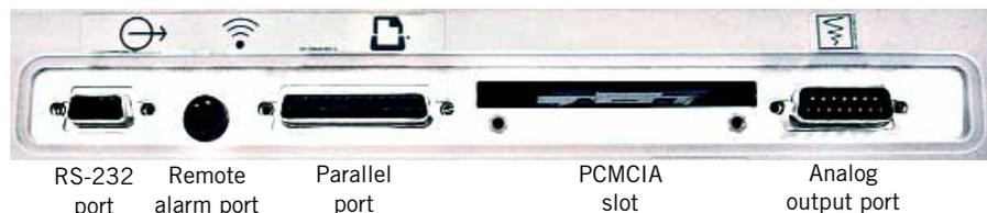
Figure 9-56: External Connectors with Port Covers and Jackscrews Removed
