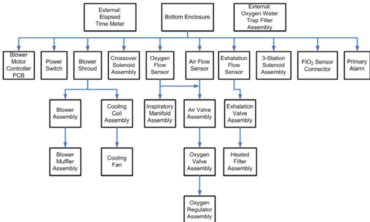
Figure 10-1: Bottom Enclosure Disassembly Flow Chart
