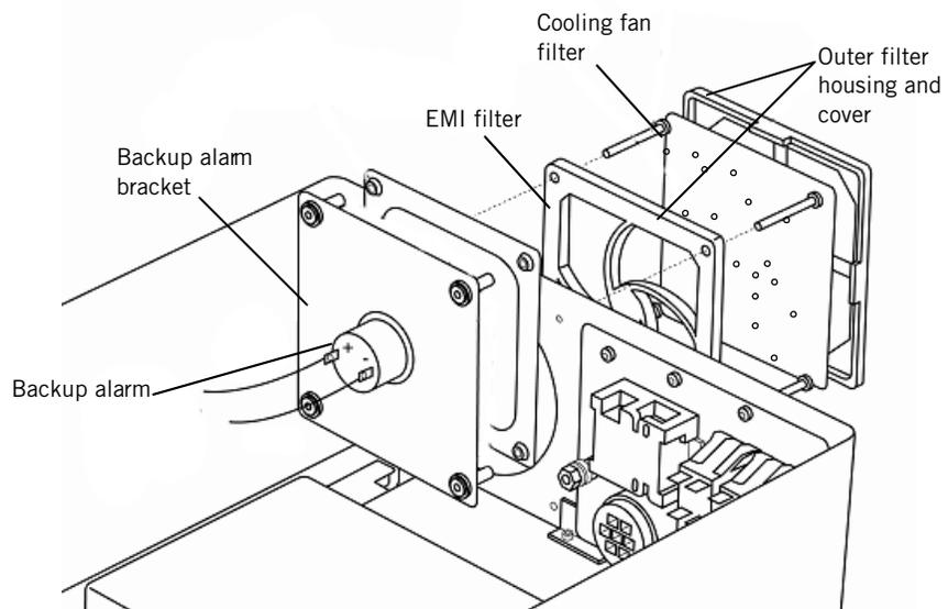
Figure 10-25: Removing the Backup Alarm
