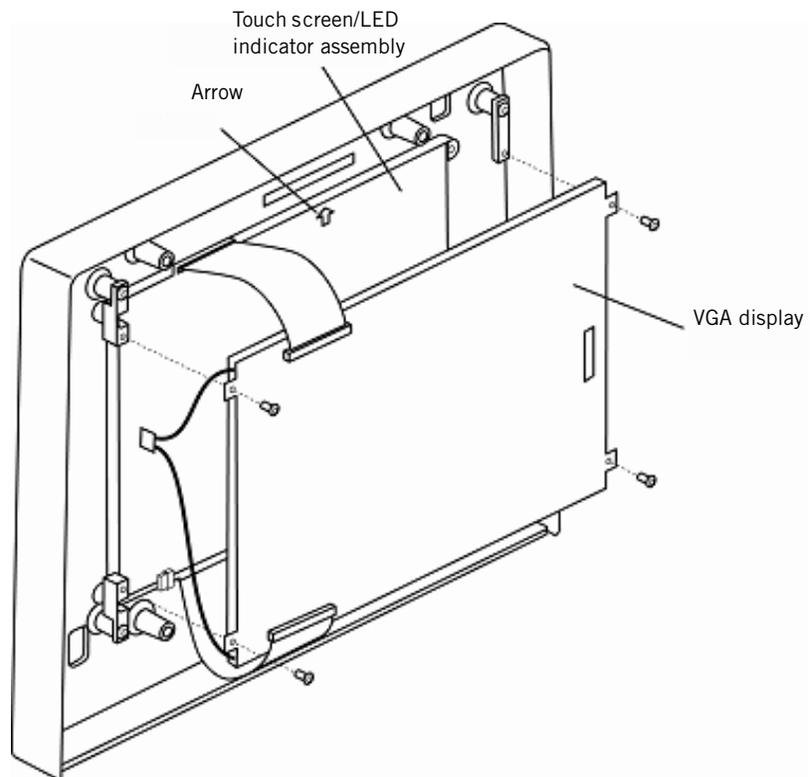
Figure 9-35: VGA Display and Touch Screen Assembly
