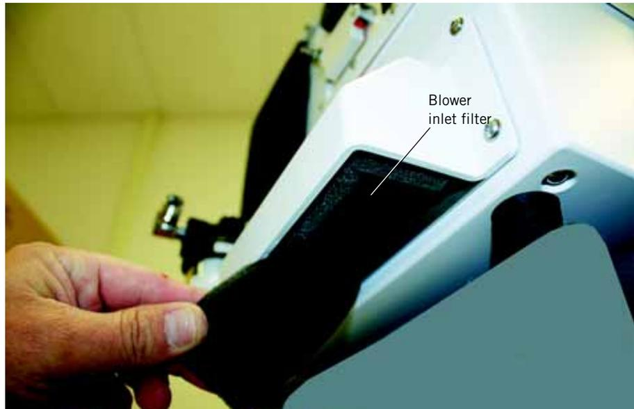
*Figure 10-4: Removing Blower Inlet Filter*
