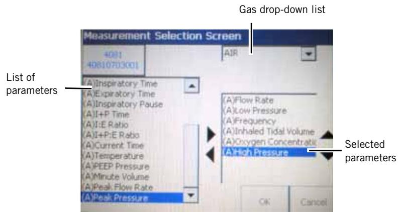
Figure 8-4: Measurement Selection Screen
