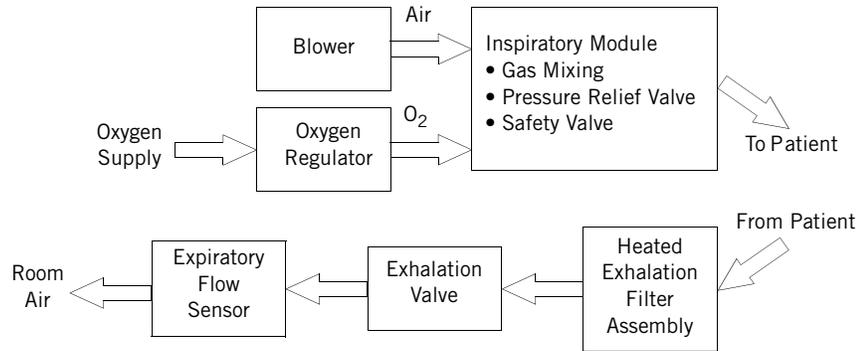
Figure 3-1: Pneumatic System Block Diagram
