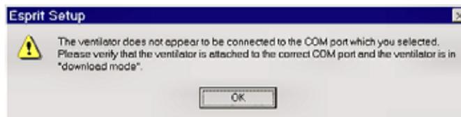
Figure 7-4: Software Download Communication Error
