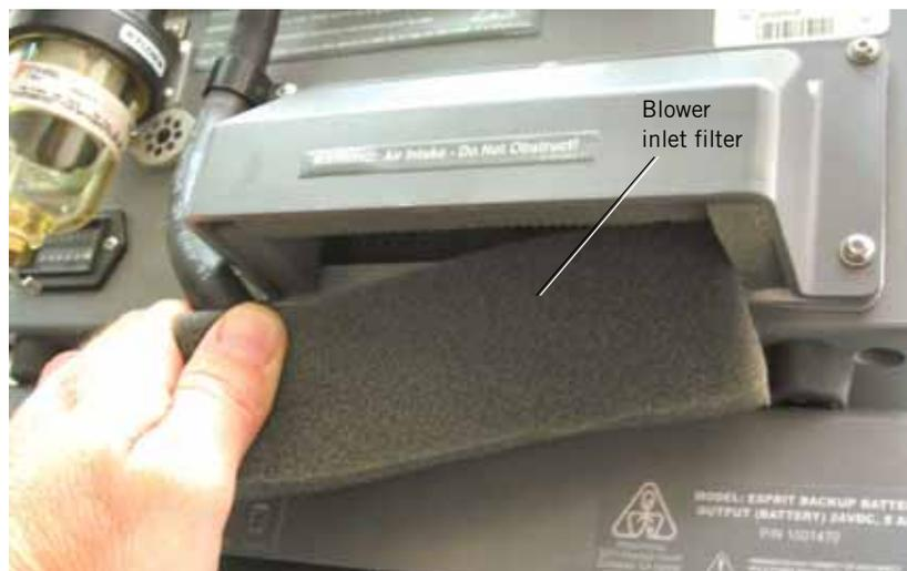
Figure 9-5: Blower Inlet Filter
