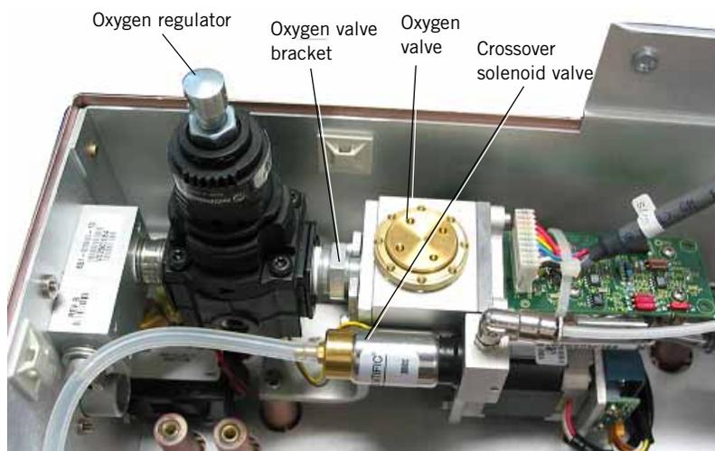
Figure 10-51: Oxygen Valve and Oxygen Regulator
