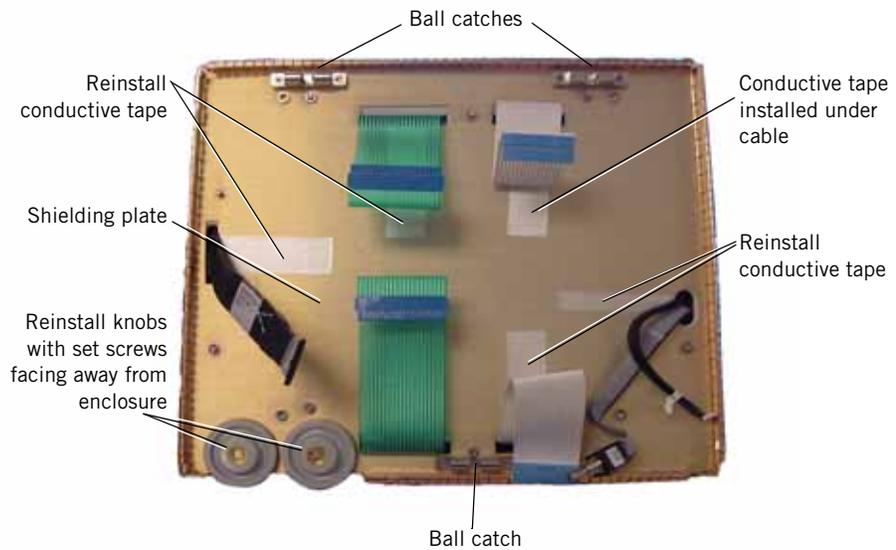
Figure 9-96: Front of Ventilator Before Installing 10.4-in. GUI
