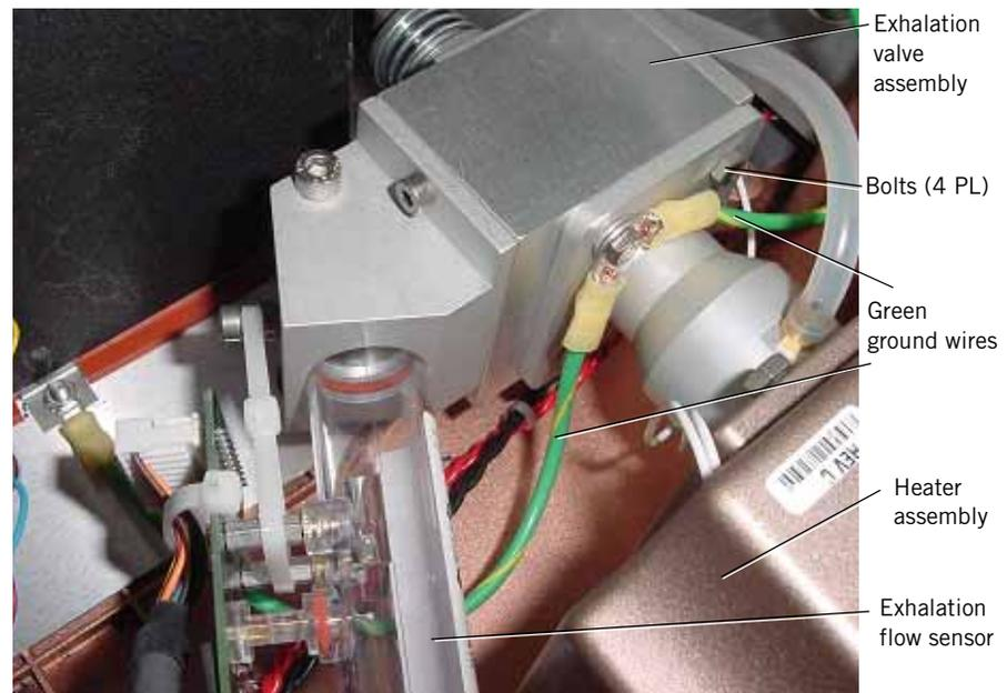
Figure 9-66: Exhalation Valve and Filter Heater Assembly
