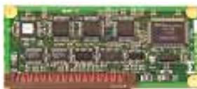
The digital PCB conditions serial port signals coming from and going to the CPU PCB. It also contains control circuitry for the power fail alarm, primary alarm, backup alarm, RS-232 port, and rotary encoder.
