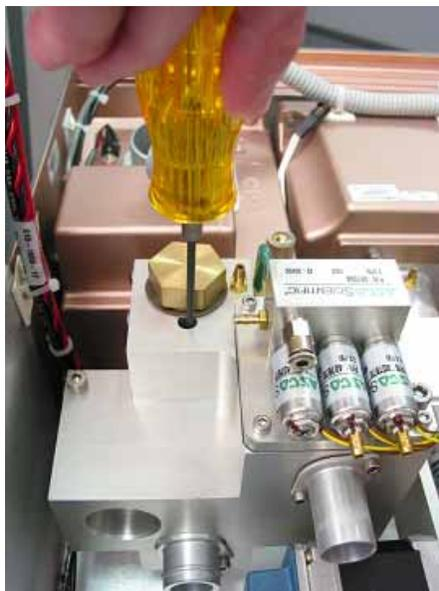
Figure 10-47: Recessed 2.5-mm Setscrew Securing Outlet Port
