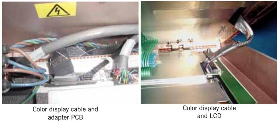
Figure 9-27: 2nd Generation 10.4-in. GUI Assembly
