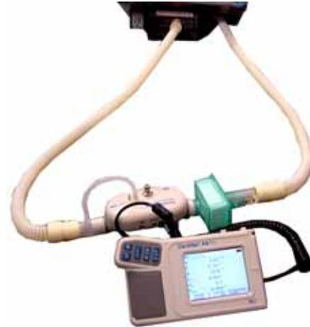
Figure 5-14: Exhalation Flow Sensor Troubleshooting Setup
