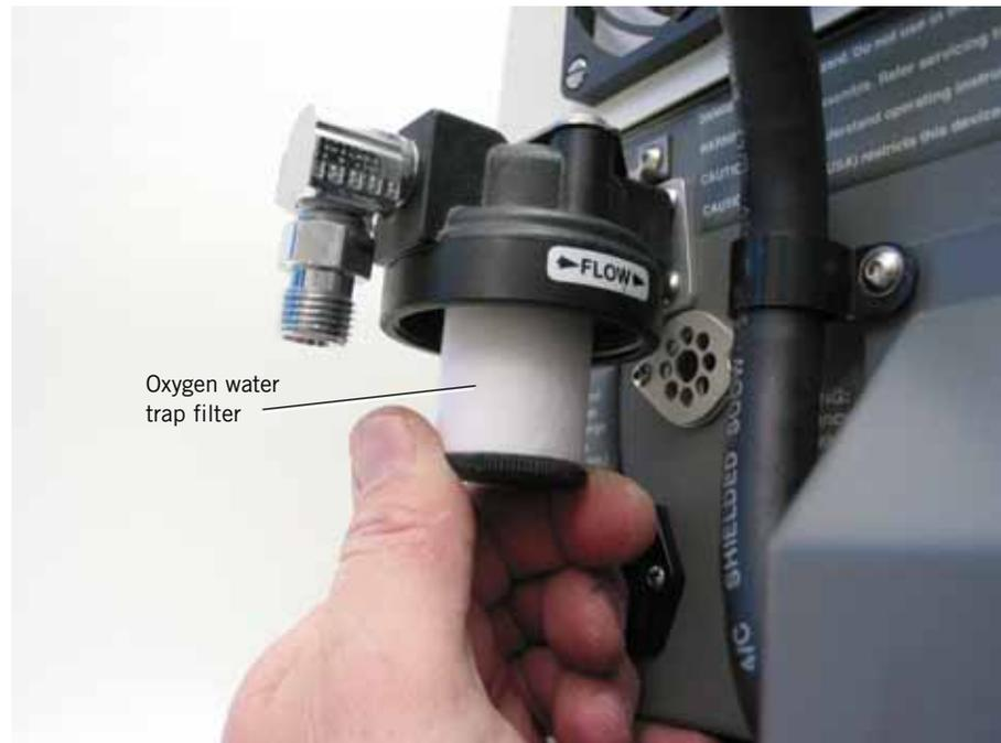
*Figure 9-6: Oxygen Water Trap Filter*
