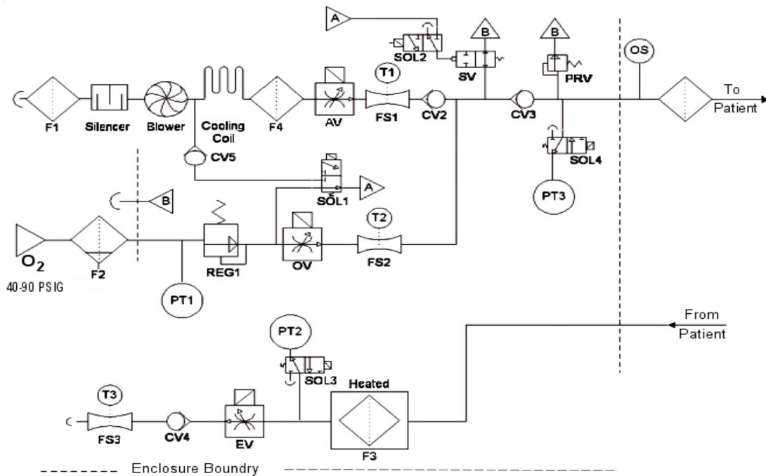
Figure 3-2: Pneumatic Schematic
