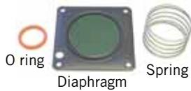
The safety valve contains a spring-loaded diaphragm that is controlled by safety valve pilot solenoid (SOL2). Under normal conditions the safety valve is closed, allowing delivered flow to reach the patient. In the event of a safety valve open (SVO) condition, pilot pressure is vented to atmosphere, which opens the safety valve and allows the patient to breathe room air through the safety port at the back of the ventilator.
