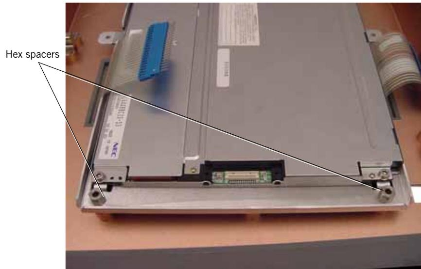
Figure 9-100: Installing the LCD
