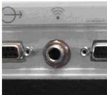
Figure 9-59: Remote Alarm Jack (Outside view)
