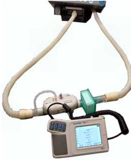
Figure 5-12: Pressure Relief Valve Troubleshooting Setup
