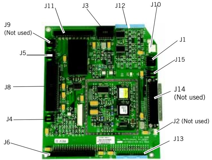
Figure 10-24: MMI PCB Connectors
