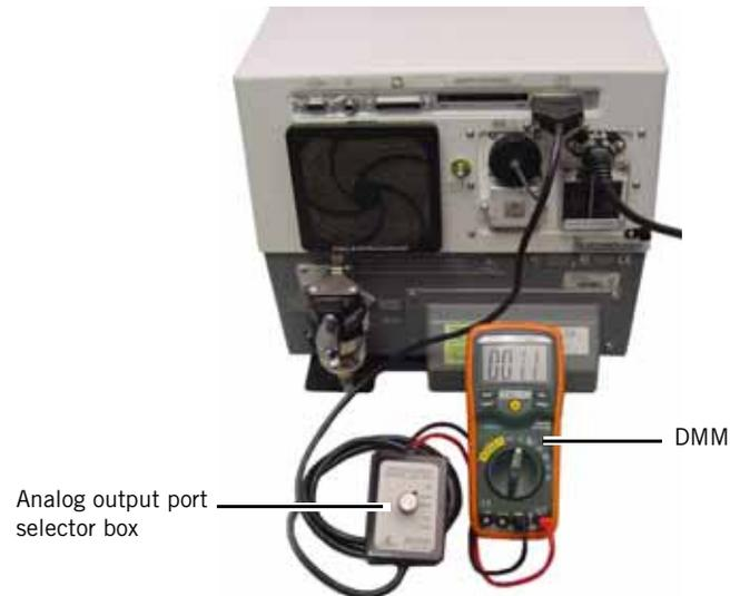
Figure 8-23: Analog Output Port Selector Box Setup
