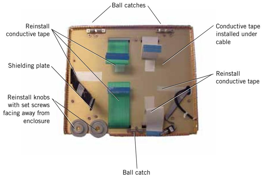
Figure 9-94: Front of Ventilator Before Installing 10.4-in. GUI
