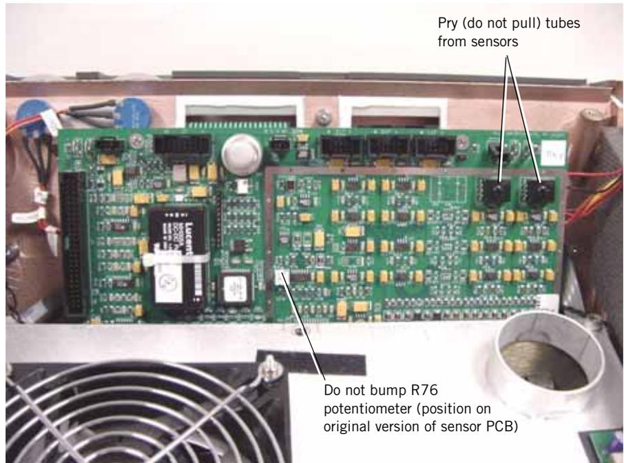
Figure 9-8: Sensor PCB
