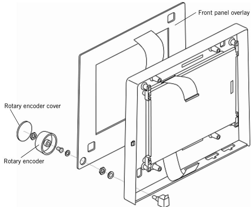
Figure 9-31: Rotary Encoder (9.5-in. GUI)
