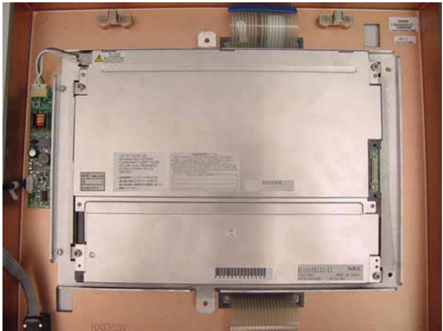
Figure 9-99: Installing the LCD
