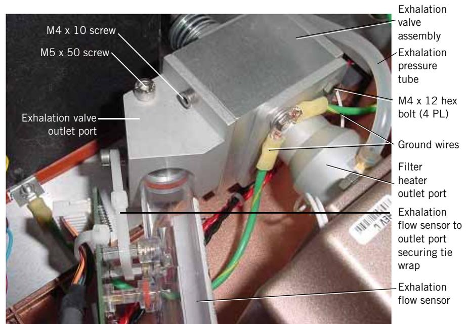
Figure 10-41: Exhalation Valve and Filter Heater Assembly
