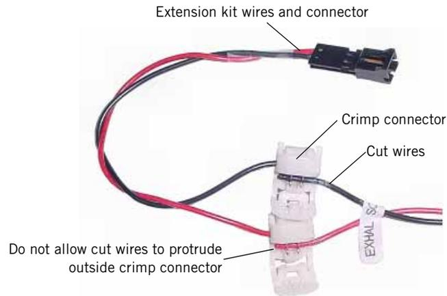
Figure 9-76: Installing Cut Wires into Crimp Connector
