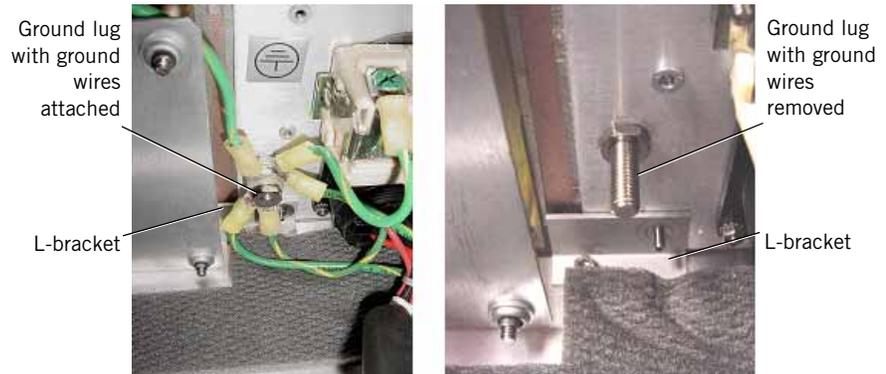
Figure 9-47: Ground Lug and L-Bracket
