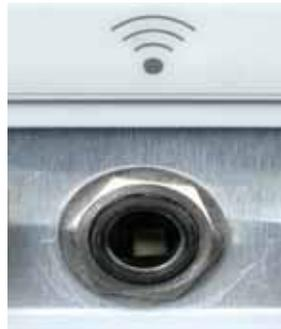
Figure 10-35: Remote Alarm Jack (Outside View)
