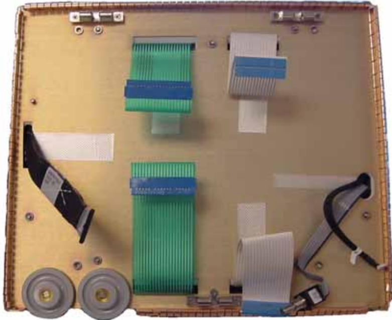
Figure 9-26: Front of Ventilator with 10.4-in. GUI Removed
