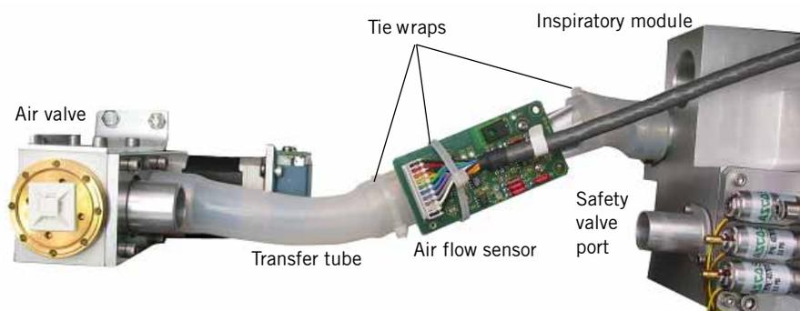
Figure 10-45: Air Flow Sensor
