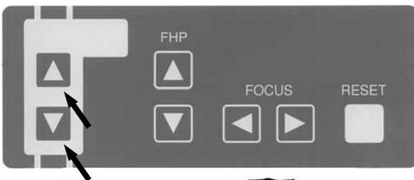
Depress either **U P** **D O W N** key on the Beam Control Panel or the one on the Sliding Unit to move position of Ear Rod(TMJ Frontal). Align ear rods to patient's external auditory foramen.
