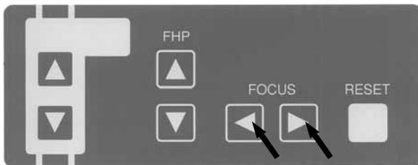
Depress either **Forward Movement** or **Backward Movement** key of FOCUS switch on the Beam Operation Panel to turn Patient Positioning Beams on.
