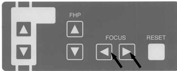
Depress either **Forward Movement** or **Backward Movement** key of FOCUS Beam switch on the Beam Operation Panel, and align Focus Beam Line with roots of upper and lower anterior teeth.
