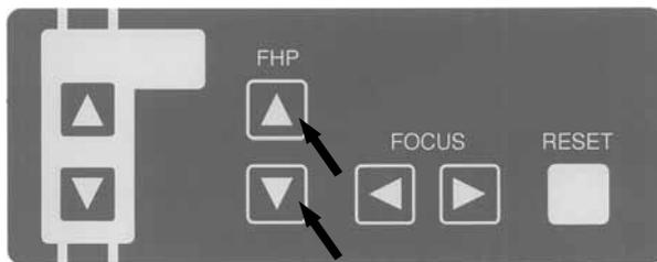
Depress either **UP** · **DOWN** key of Frankfort Beam on Beam Operation Panel and align Frankfort Beam Line with Frankfort Plane of a patient.
