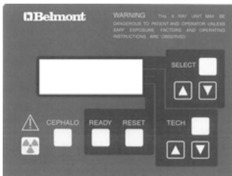
\* Set the Exposure Mode, KvP and mA by using this control panel.
