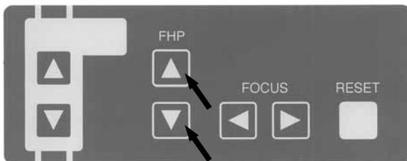
Depress either **UP** or **DOWN** key of Frankfort Beam on Beam Operation Panel and align Frankfort Beam Line with Frankfort Plane of a patient.
