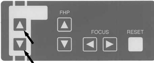
Depress either **U P** **D O W N** key on the Beam Control Panel or the one on the Sliding Unit to move position of Ear Rods (TMJ Lateral). Bring ear rods close to patient's external auditory foramen.
