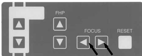
Depress either **Forward Movement** · or **Backward Movement** key of FOCUS Beam switch on Beam Operation Panel, and align Focus Beam Line with roots of upper and lower anterior teeth.
