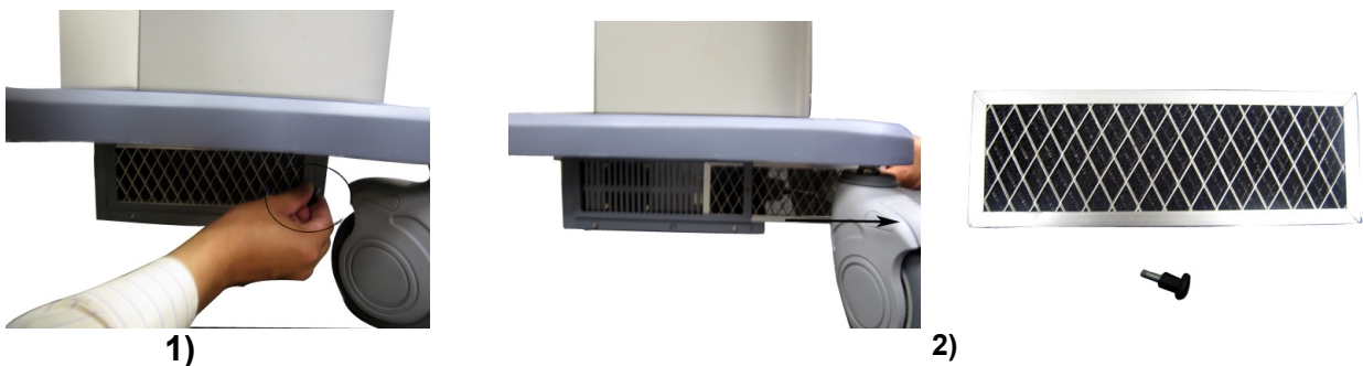
Figure 8-1 Air filter and Knob Screw Disassembly
