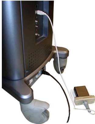
Figure 3-11 Connect Foot Switch to the system
