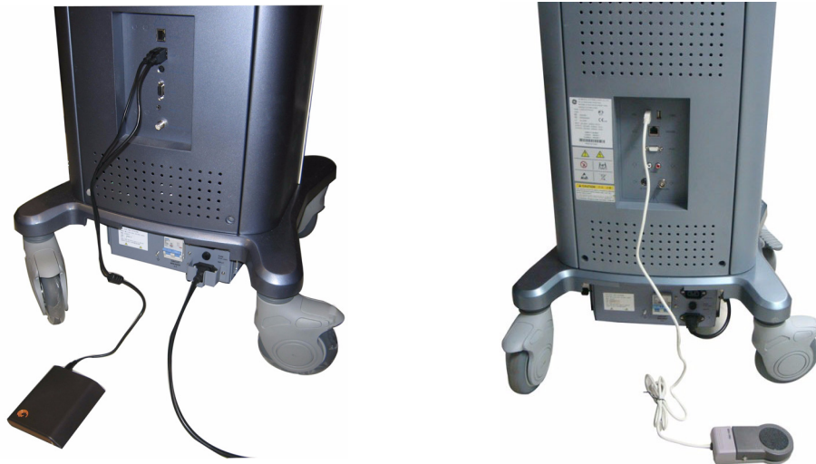
Figure 3-14 USB Hard Disk Connection
