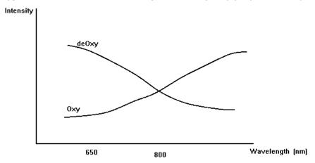
Careful analysis of the light from two wavelengths allows the pulse oximeter to determine the percentage of hemoglobin saturated with oxygen.
