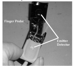
The most common probe for a pulse oximeter is the finger probe. Broken wires, springs and plastic cases are common problems that can be fixed in the field.
