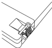
Hook the lock lever on the projection from the body and press it down until it is horizontal (flat position).
