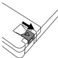
Lift the lock lever to open the battery compartment lid as shown in the left picture.
