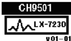
Make sure whether the channel number on the LCD matches the channel number indicated on the label of the LX-7230N and the channel number configured on the receiving monitor. This screen automatically moves onto the next waveform display screen.
