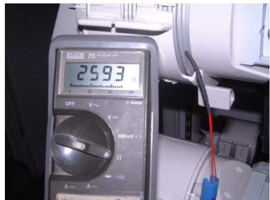
Fig. 10 Measuring control temperature and temperature overshoot
