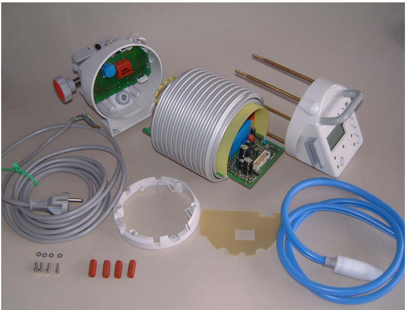
Fig. 15 ASTOTHERM PLUS and ASTOLINE dismantled into assemblies
