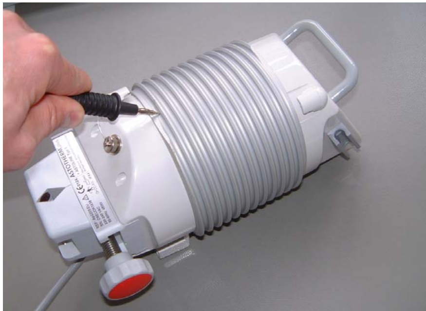
Fig. 17 Contact point for protective earth resistance test
