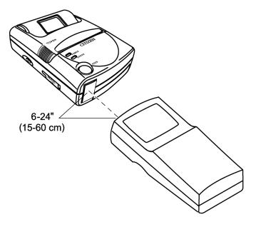
**Figure 3: Printer Alignment**
