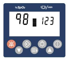
Movement of the blip bar indicates that real-time data is displayed. Continue to listen for the pulse beep tone as the monitor is used. If it does not sound with each pulse, it indicates one of the following:
