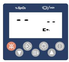
The monitor displays [--/--] (two dashes and two dashes) and the **Pulse Search** indicator does not display when the monitor fails to detect an *OXIMAX* sensor or an invalid sensor.
