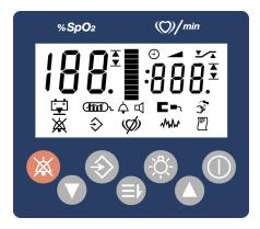
**%SpO2** Displays the measured percent of oxygen saturation.
