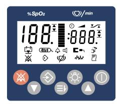
Decimal points after the %SpO2 or pulse rate indicate that the respective limits have been changed from the power-on default values.
