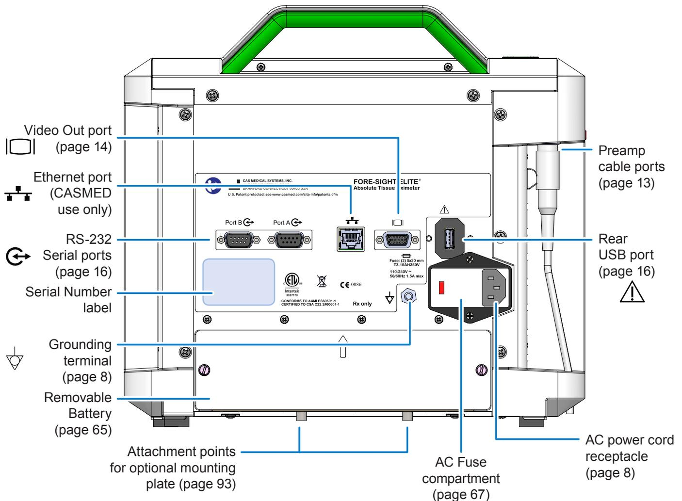
Figure 3: Oximeter — Rear View
