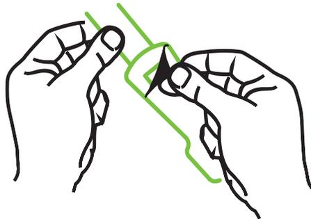
**Figure 15:** Removing Protective Liner from Sensor
