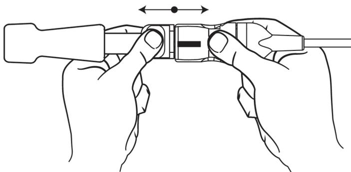
**Figure 26:** Disconnecting a Sensor from the Preamp Cable
