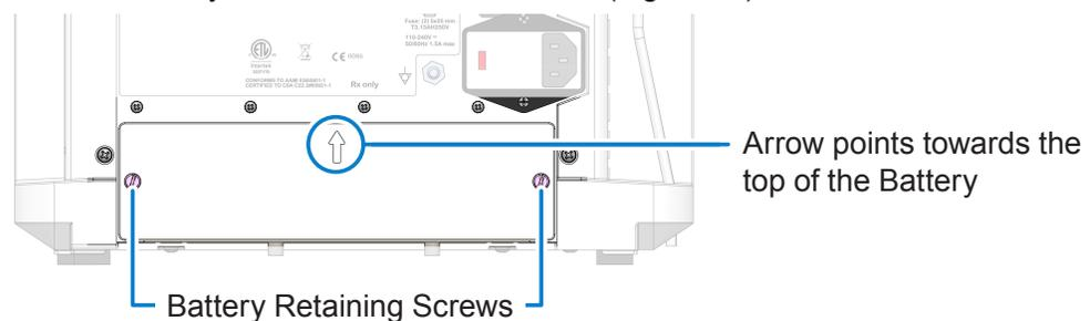
**Figure 32:** Battery Compartment
