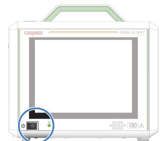
**Figure 8:** Power Switch and AC Charge Indicator
