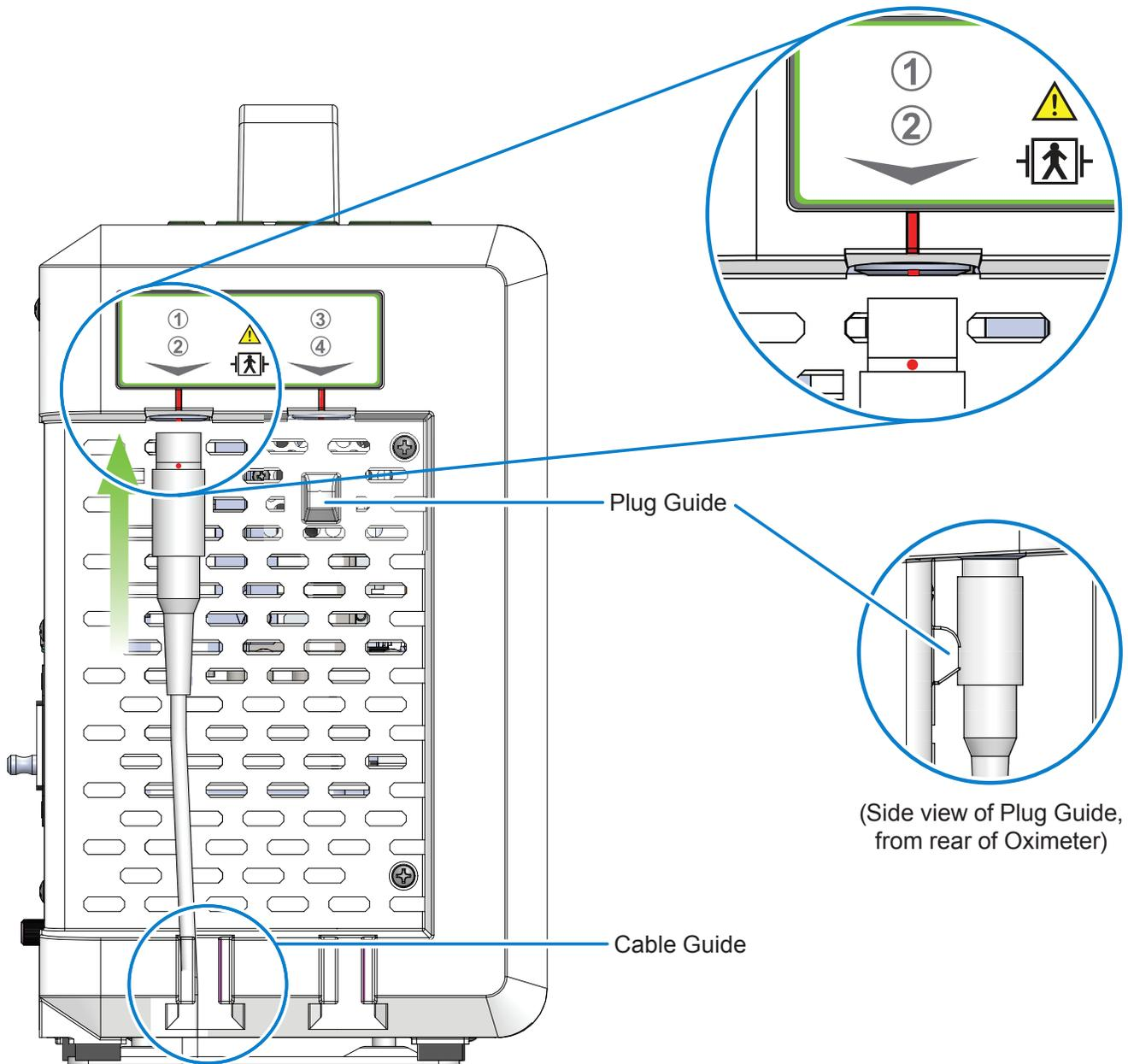
Figure 10: Attaching the Preamp Cable
