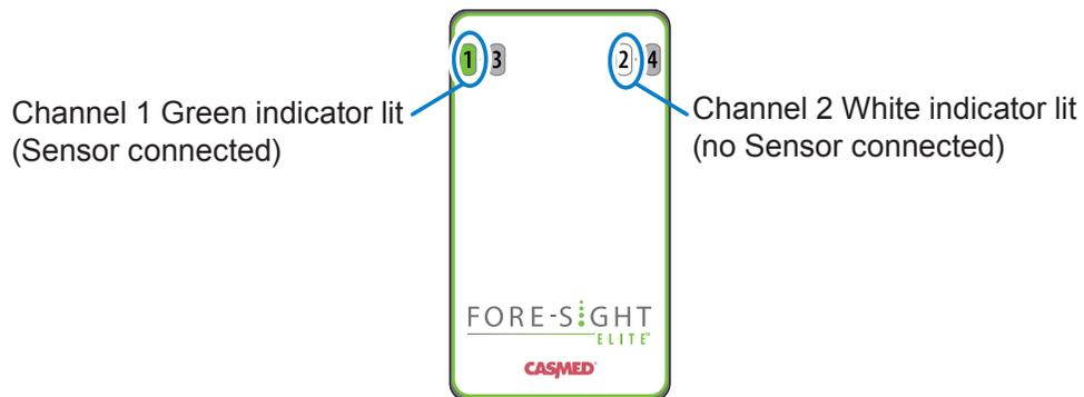
**Figure 19:** Sensor connected to Channel 1
