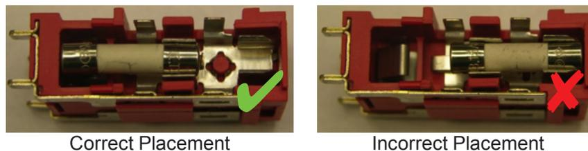
**Figure 34:** AC Fuse Placement
