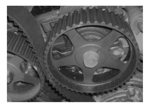
Above is an example of a loose belt that is no longer in contact with the corresponding gear.
