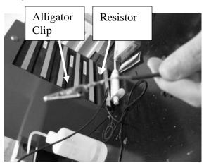
2. Slide the heat shrink over the resistor connections and heat with hot air gun (or lighter if you do not have a hot air gun). Then fit the alligator clip wrap over the clip.
