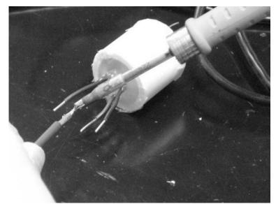
Tape the wires together with electrical tape.
