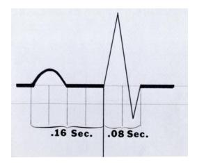
An "inverted signal" means that one of the main peaks of the signal is inverted. An inverted signal generally looks like this:
