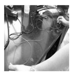
2. These wires will become the main cables of each lead. Strip both ends of each wire, and fit a piece of heat shrink tubing onto the wire.
