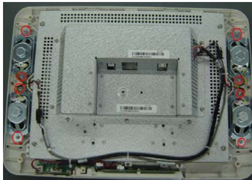
Fig 7-95 Disassemble the speaker on the display (2)
