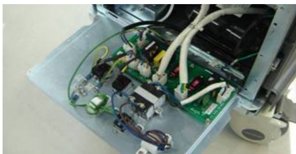
Fig 7-64 Disassemble the power supply connecting board
