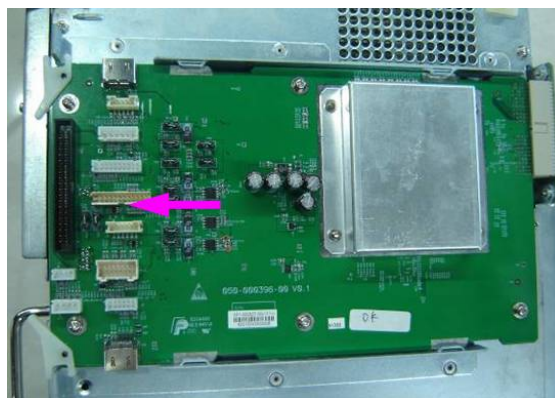
Fig 7-32 Disassemble the IO port board (1)
