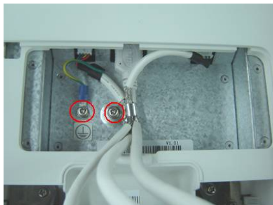
Fig 7-10 Disassemble the monitor assembly (2)
