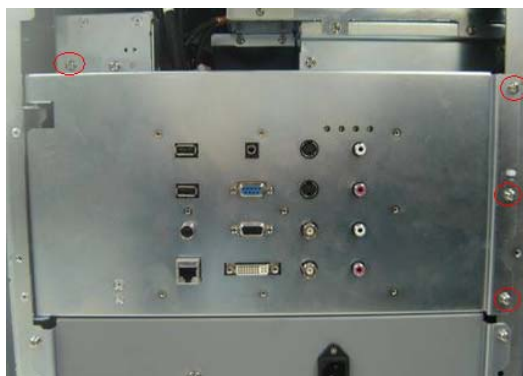
Fig 7-16 Disassemble the IO assembly (1)
