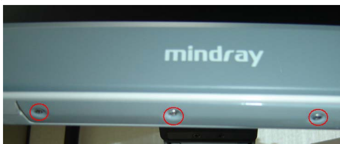
Fig 7-93 Disassemble the Display bottom light
