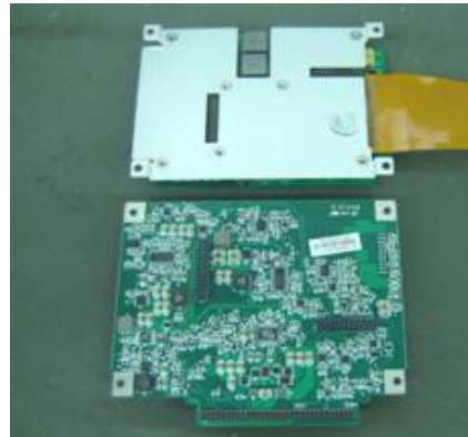
Fig 7-43 Disassemble the power supply main board, auxiliary board (3)
