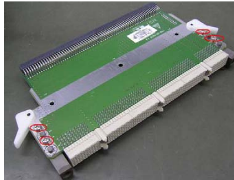
Fig 7-38 Disassemble the probe connecting board (3)
