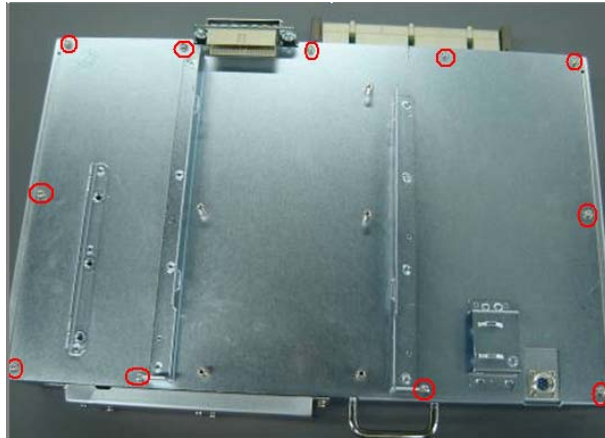
Fig 7-39 Disassemble the main unit box cover
