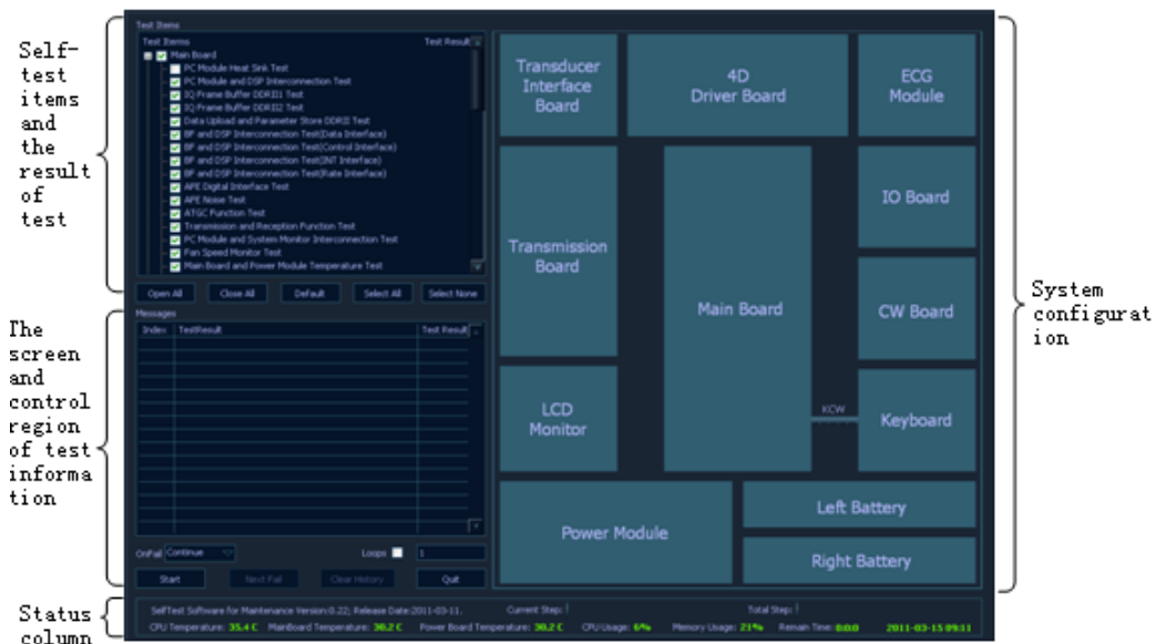
Fig 9-2 The interface of maintenance and self-test
