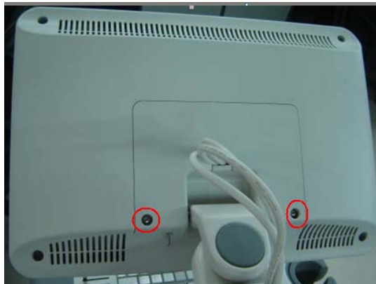
Fig 7-9 Disassemble the monitor assembly (1)
