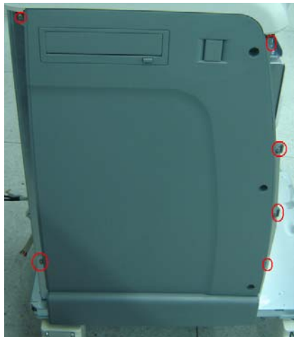
Fig 7-7 Disassemble the Main Unit Left Cover
