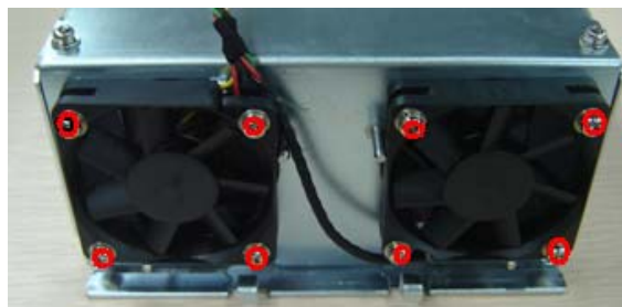
Fig 7-81 Disassemble the battery fan
