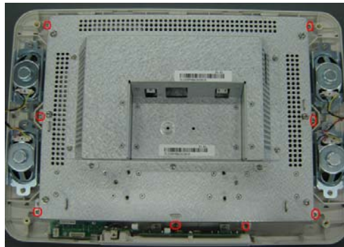
Fig 7-96 Disassemble the display assembly
