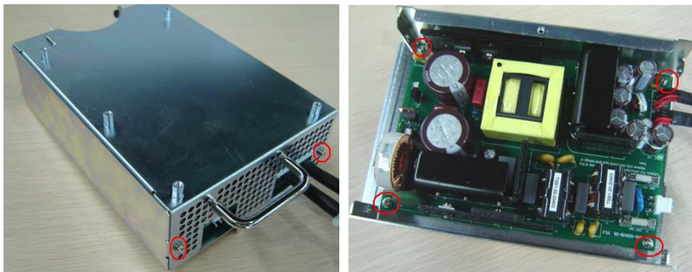
Fig 7-76 Disassemble the AC-DC board
