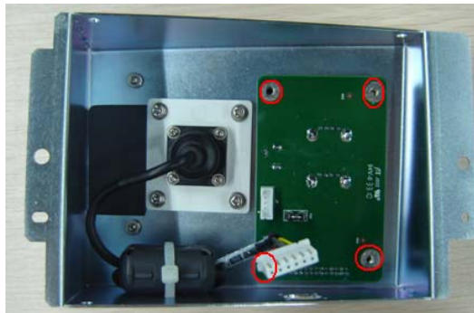
Fig 7-72 Disassemble the I/O front board and ECG board (2)
