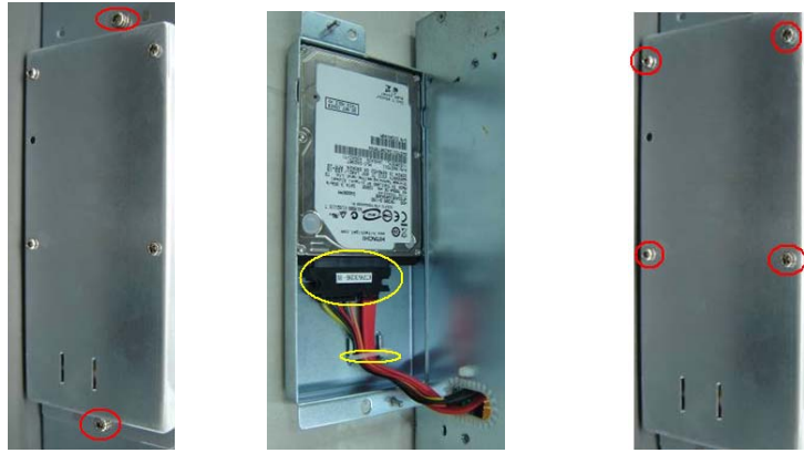
Fig 7-83 Disassemble the hard disk
