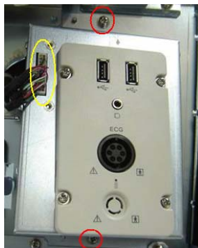
Fig 7-70 Disassemble the ECG
