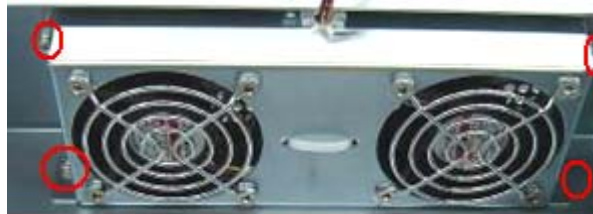
Fig 7-78 Disassemble the system air inlet fan
