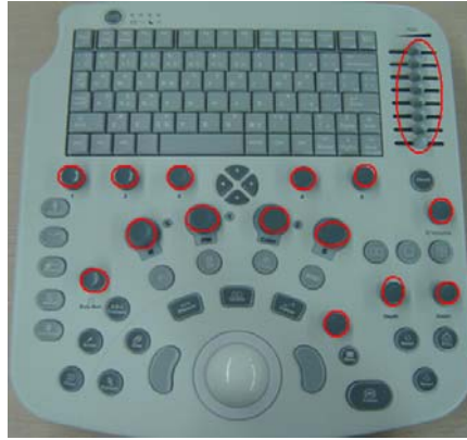
Fig 7-59 Disassemble the control panel (1)
