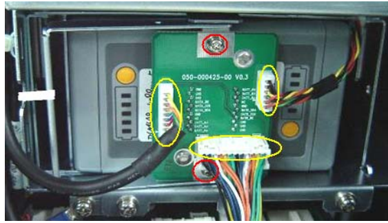
Fig 7-77 Disassemble the battery connecting board
