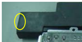
Fig 7-46 Disassemble the transmitting board heat-conducting pad and FPGA heat-conducting pad
