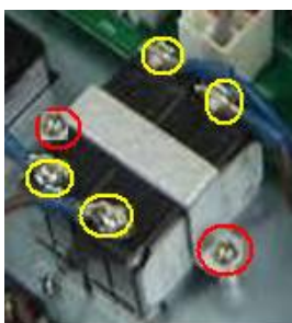
Fig 7-66 Disassemble the circuit breaker
