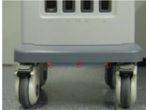
Fig 7-4 Disassemble the main unit front cover (1)
