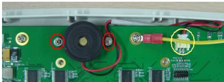
Fig 7-58 Disassemble the buzzer
