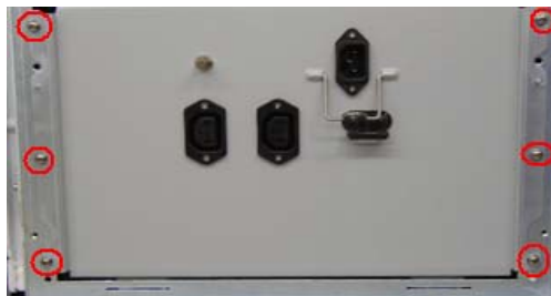
Fig 7-63 Disassemble the power supply connecting board
