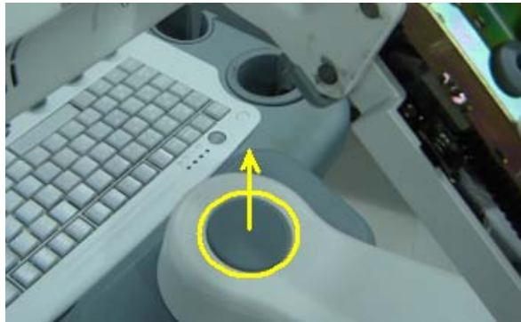
Fig 7-15 Disassemble the support arm (2)
