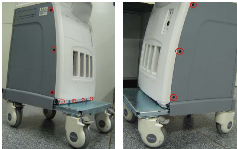
Fig 7-5 Disassemble the main unit front cover (2)
