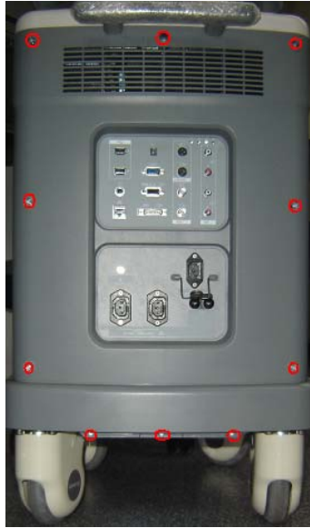
Fig 7-6 Disassemble the rear cover
