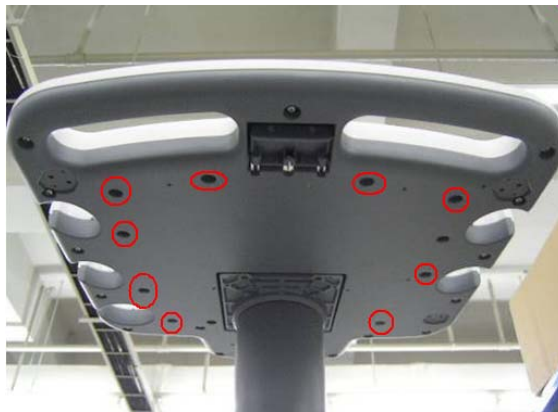
Fig 7-20 Disassemble the control panel (1)
