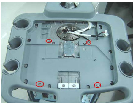
Fig 7-91 Disassemble the cover of cast aluminium base (1)
