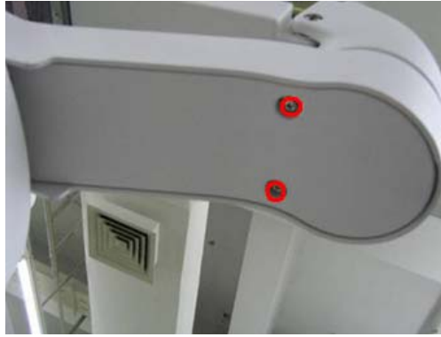
Fig 7-14 Disassemble the support arm (1)
