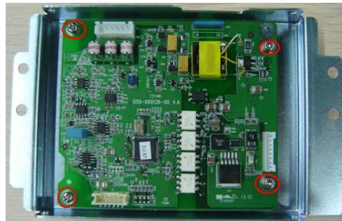
Fig 7-73 Disassemble the I/O front board and ECG board (3)
