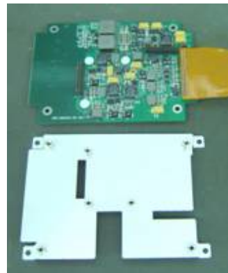
Fig 7-44 Disassemble the power supply main board, auxiliary board (4)
