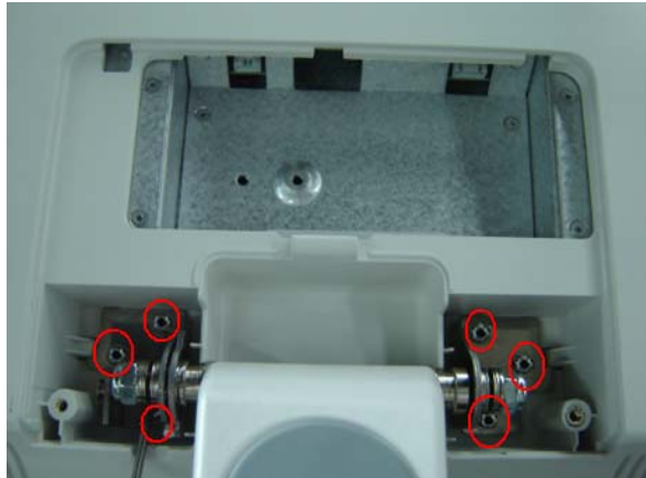
Fig 7-11 Disassemble the monitor assembly (3)
