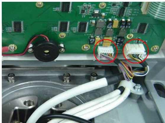
Fig 7-21 Disassemble the control panel (2)
