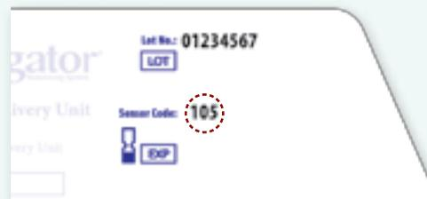
**Important:** Once the code has been entered and you have hit the Set button as instructed below, you will not be able to change the sensor code number. If you have entered the code incorrectly, you will have to replace the sensor and enter the right sensor code. If you choose the wrong sensor code, you may get erroneous results from the sensor.
