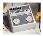
4.6. Joule Test Using Built-In energy circuit.
