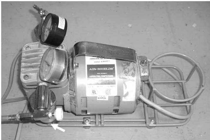
This is a typical simple suction machine. The collection jar and seal are missing. The float valve and trap are shown near the bottom left (arrow).
