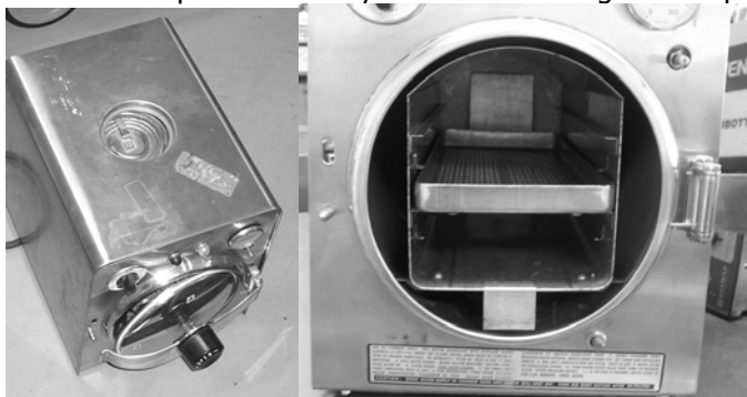
Inside and outside of a small, electric autoclave.
