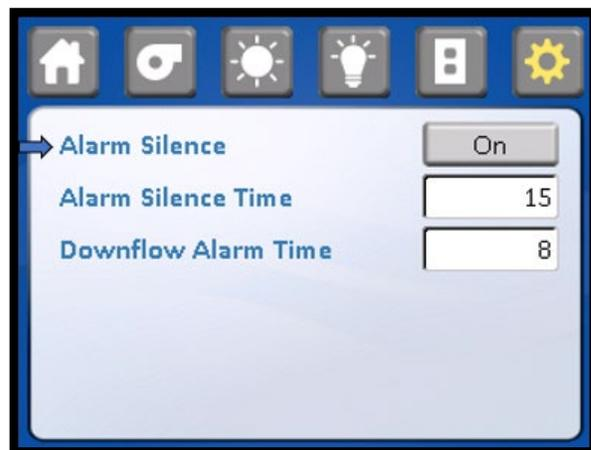
**Alarm Silence Time:** This parameter allows for the selection of time to determine how long the audible alarm shall be silenced. The time is displayed in minutes with a programmable range of 1 to 60.
