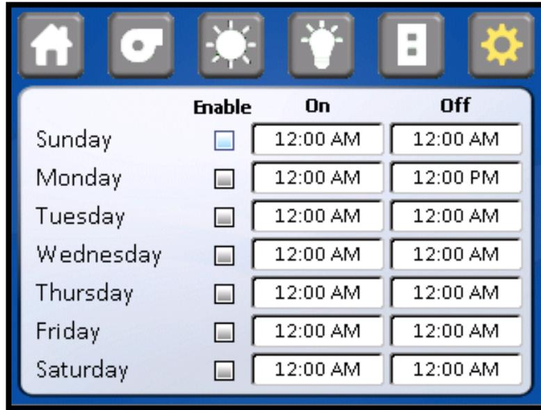
Once into the selected day, press on window to enter the on/off times. Use the keypad to enter hours or minutes. Press menu icon SAVE after each time entry. Repeat auto timer function for each day as desired
