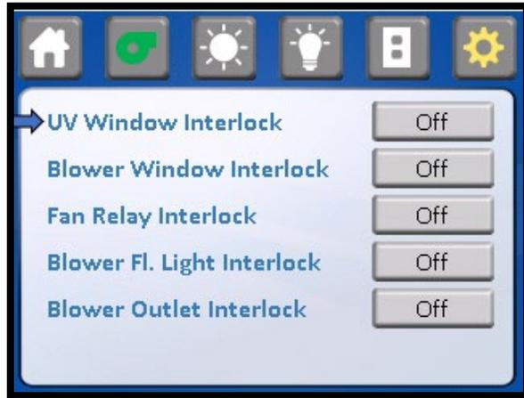
👉 **Note:** In addition to the **TOUCHLINK** system UV window interlock there is a double redundant UV window interlock relay. To override the UV window interlock for service purposes only, both interlocks must be changed through the **TOUCHLINK** system and shorting the relay connection (See electrical schematic for reference).
