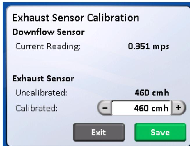
Press +/- to change exhaust volume to the value just calculated using the inflow volume.
