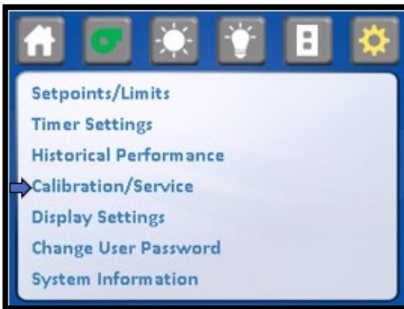
Entry into the Calibration/Service functions requires a service password for entry. After pressing the Calibration/Service menu item, a password screen will appear. The default password is "9876". Once the service password is entered; the Calibration/Service menu will appear.
