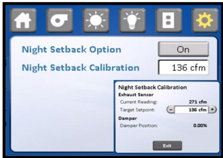
At this point, the night setback is active and the butterfly valve will begin to close. Now measure the inflow volume using a Direct Reading Instrument of inflow velocity measurement method. The goal is to reduce the inflow volume to a lower level that maintains a negative inflow velocity to save energy. This can be set at any other values within the damper operational range of 30% to 80%.
