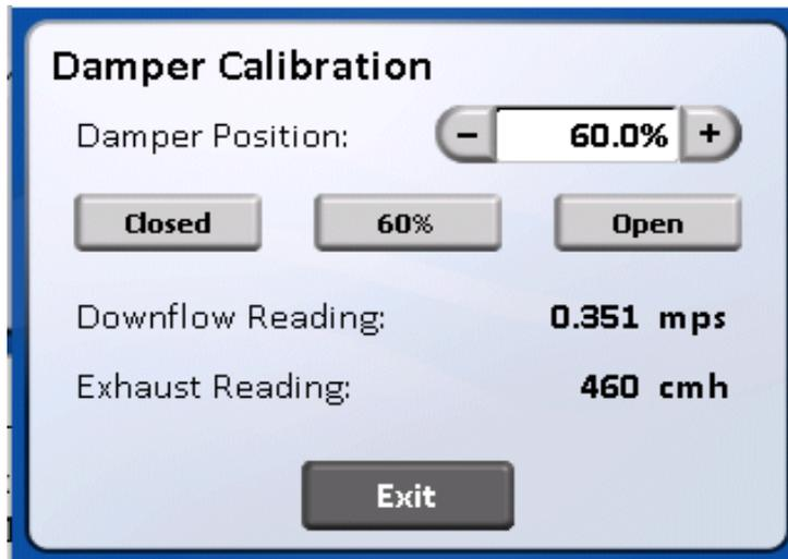
Step 4: Now, measure inflow velocity using the recommended procedure found in Table 7.0. If necessary, adjust the exhaust system and/or damper to achieve the correct inflow velocity.
