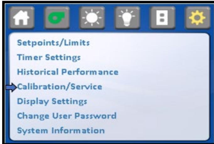
Entry into the Calibration/Service functions requires a service password for entry. After pressing the Calibration/Service menu item, a password screen will appear. The default password is "9876". Once the service password is entered, the Calibration/Service menu will appear. To exit, either press the menu or home icon.
