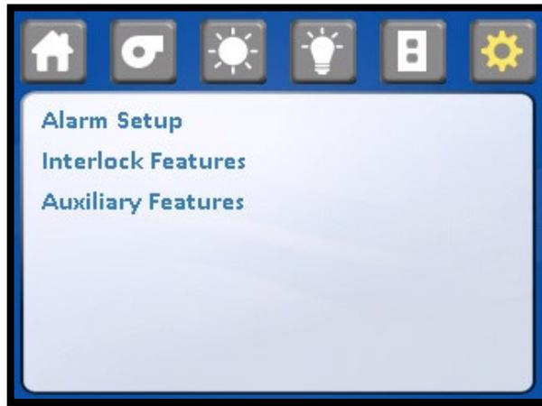
**Alarm Silence** : This parameter allows for the selection of the alarm silence key function. When the alarm silence function is on, all current and future alarms will be silenced for the designated alarm silence time (i.e. default time is 15 minutes). When the alarm silence function is off, all current alarms will be silenced for the designated alarm silence time. If a new alarm is present, the audible alarm will again be turned on.
