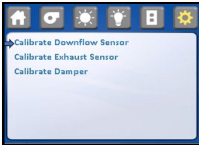
Step 2: Press CALIBRATE DOWNFLOW SENSOR to access individual calibration screen.
