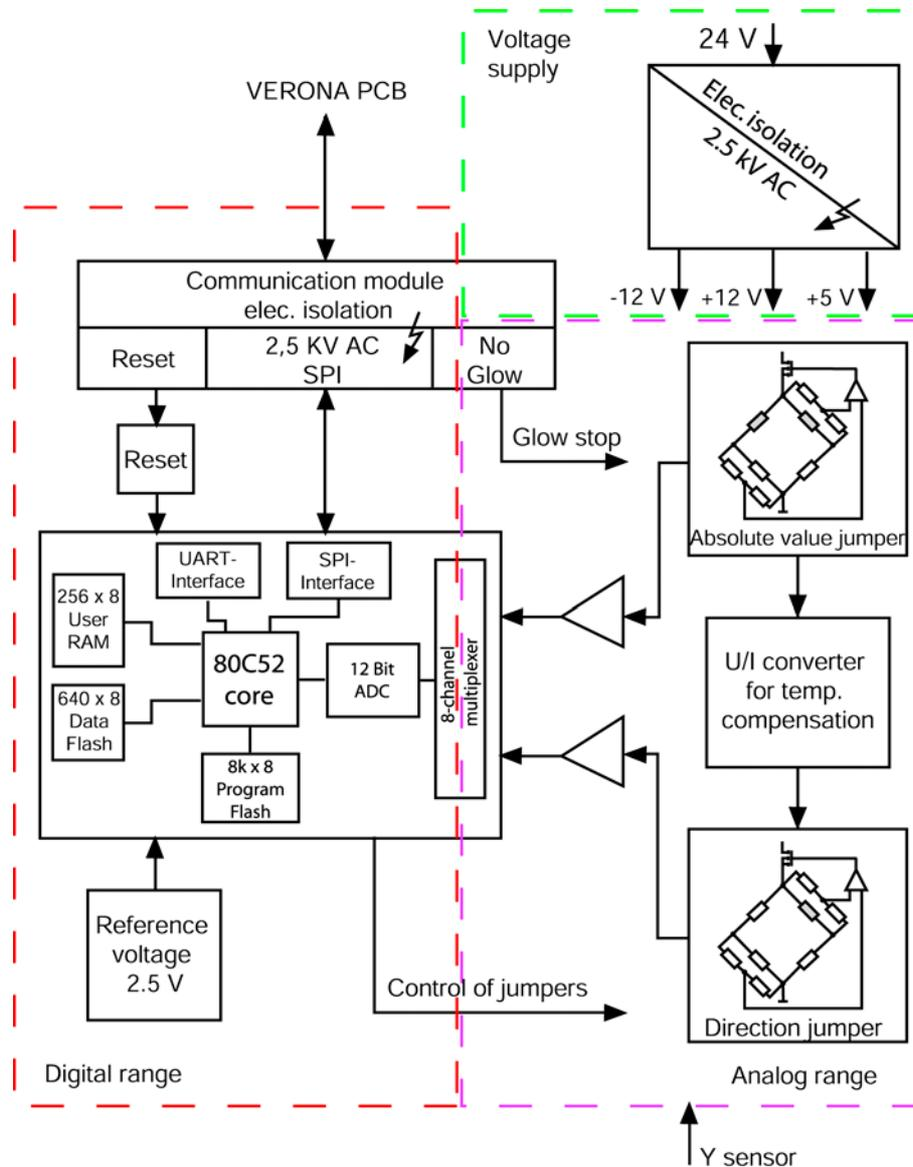
Figure 6 External Flow PCB block diagram
