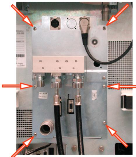
**Figure 18** CS module fixing screws
