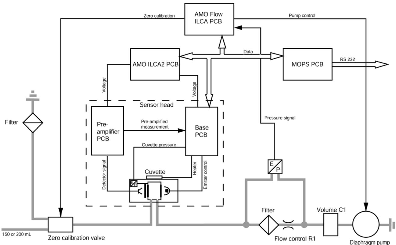
**Figure 32** Block diagram of the ILCA
