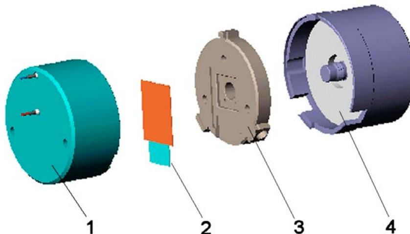
Figure 26 PATO sensor head configuration
