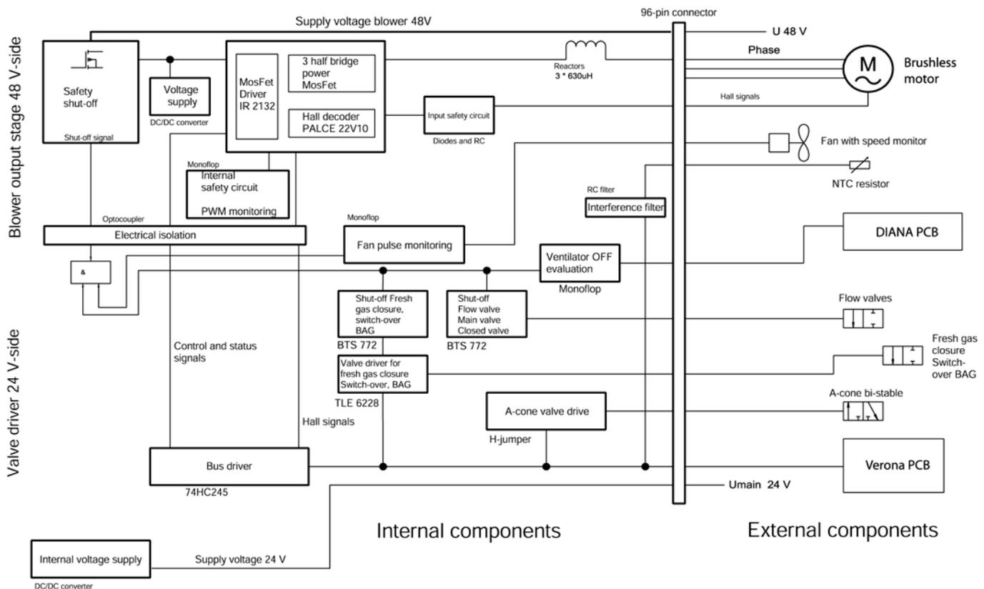
Figure 5 Vent Power PCB block diagram
