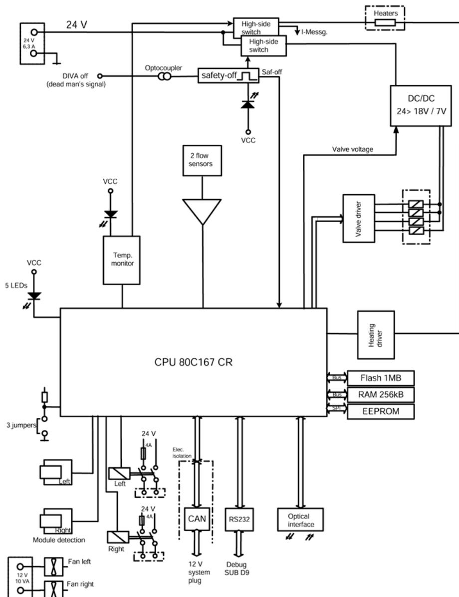
Figure 16 Block diagram of the Supply Module PCB
