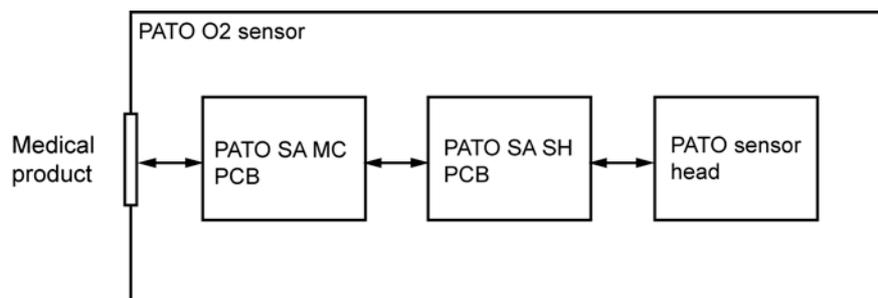
Figure 25 PATO O2 sensor configuration
