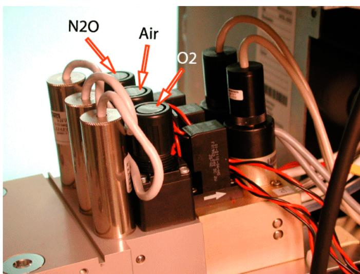
Figure 22 Assignment of pressure regulators
