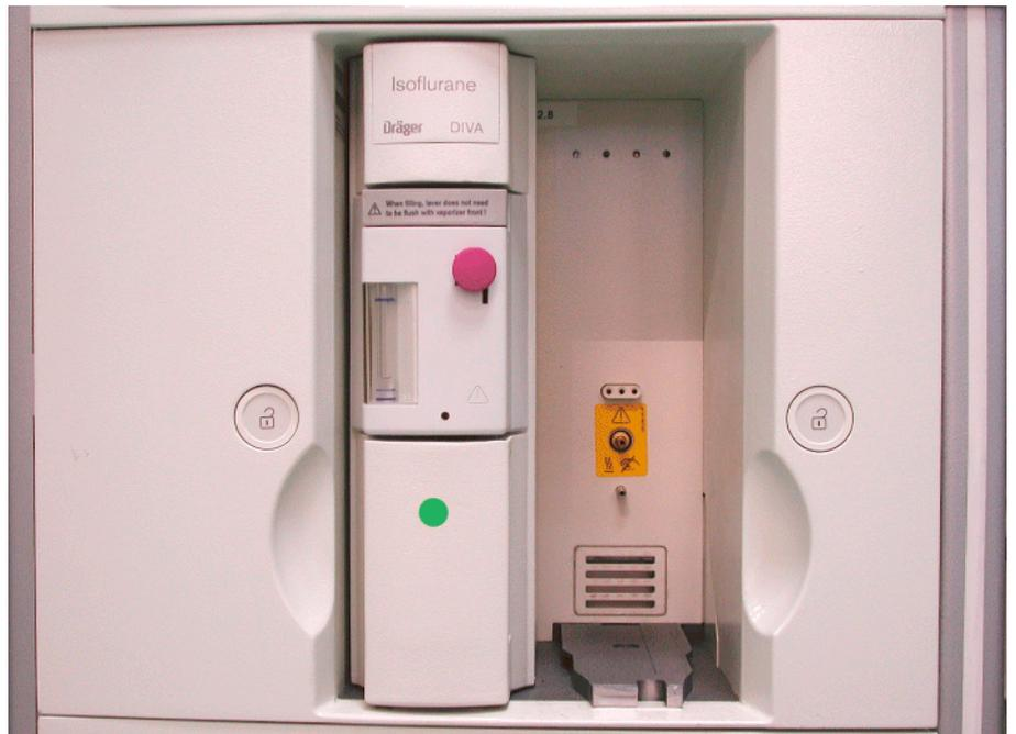
Figure 13 Supply module with 1 connected metering module
