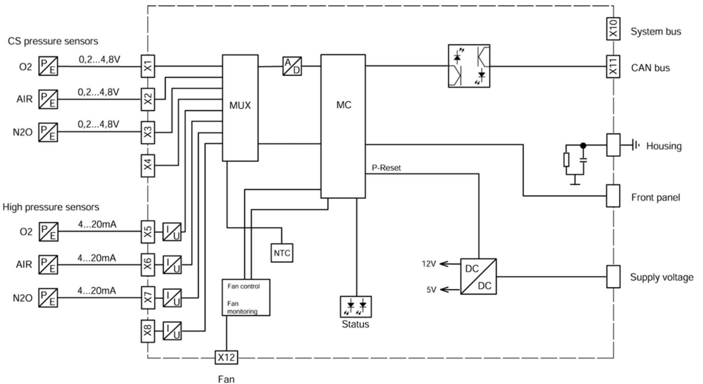
**Figure 10** Block diagram of CS Pressure PCB
