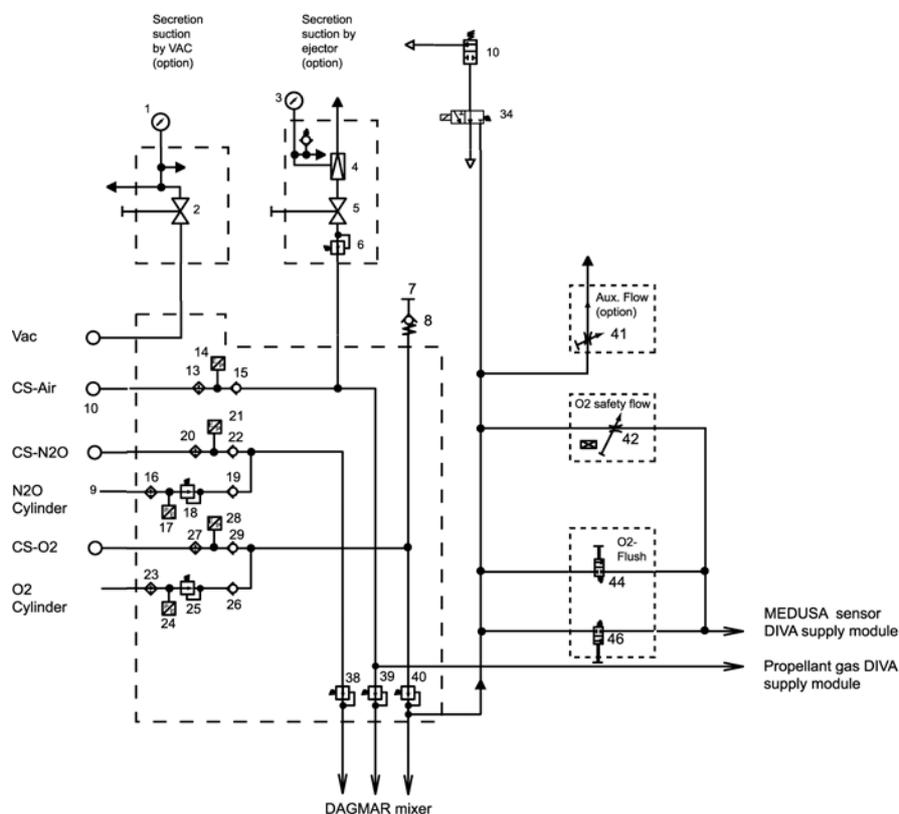
**Figure 9** Extract, gas flow diagram, gas inlet block
