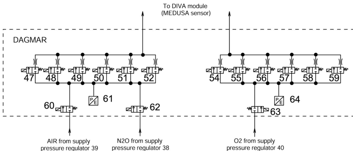
**Figure 11** Extract from Zeus gas flow diagram, Dagmar valve block
