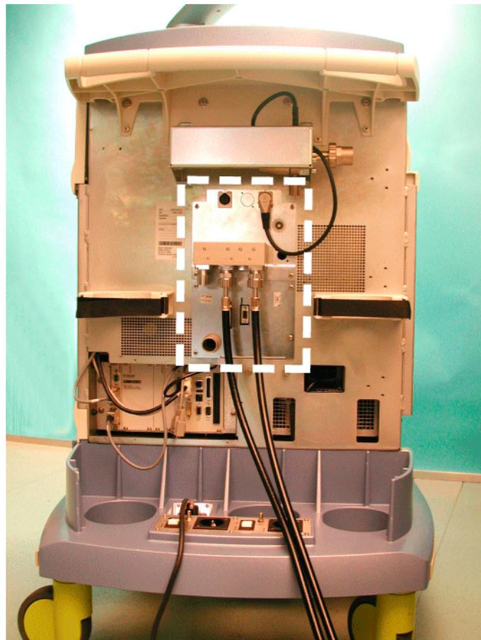
**Figure 17** CS module fitting location
