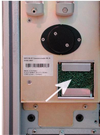
**Figure 7** Filter mat (arrow) in the GMZ
