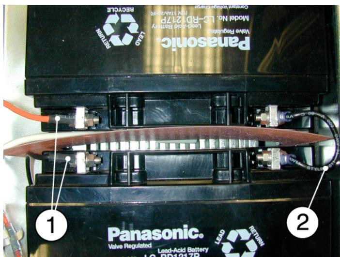
**Figure 25** Connecting the rechargeable batteries
