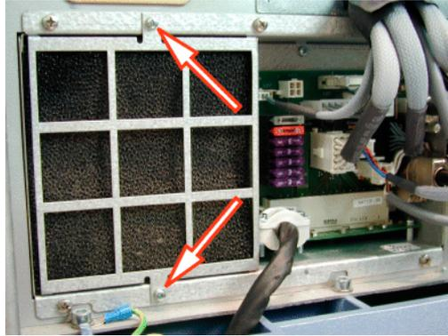
**Figure 5** Frame fixing screws
