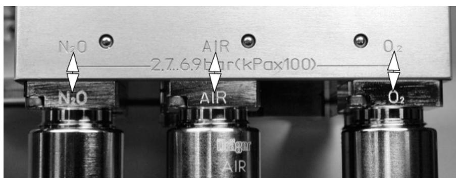
**Figure 16** NIST and cylinder connection markings
