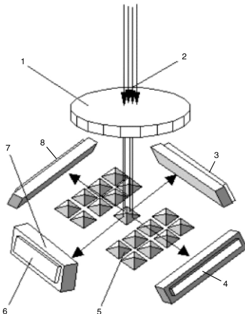
**Figure 31** Principle of multi-channel detector with IR filters
