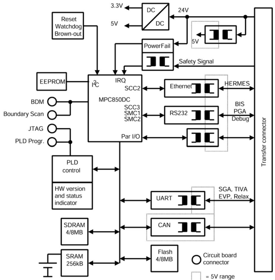
Figure 3 Block diagram of the DIANA PCB
