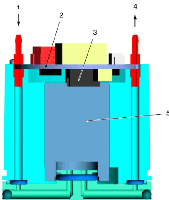
Figure 33 Layout of the OxyTrace oxygen measuring module
