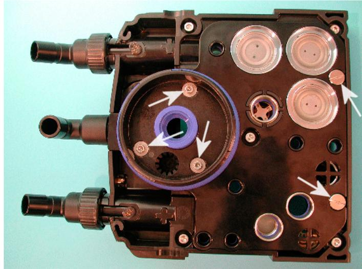
**Figure 8** Plate fixing screws
