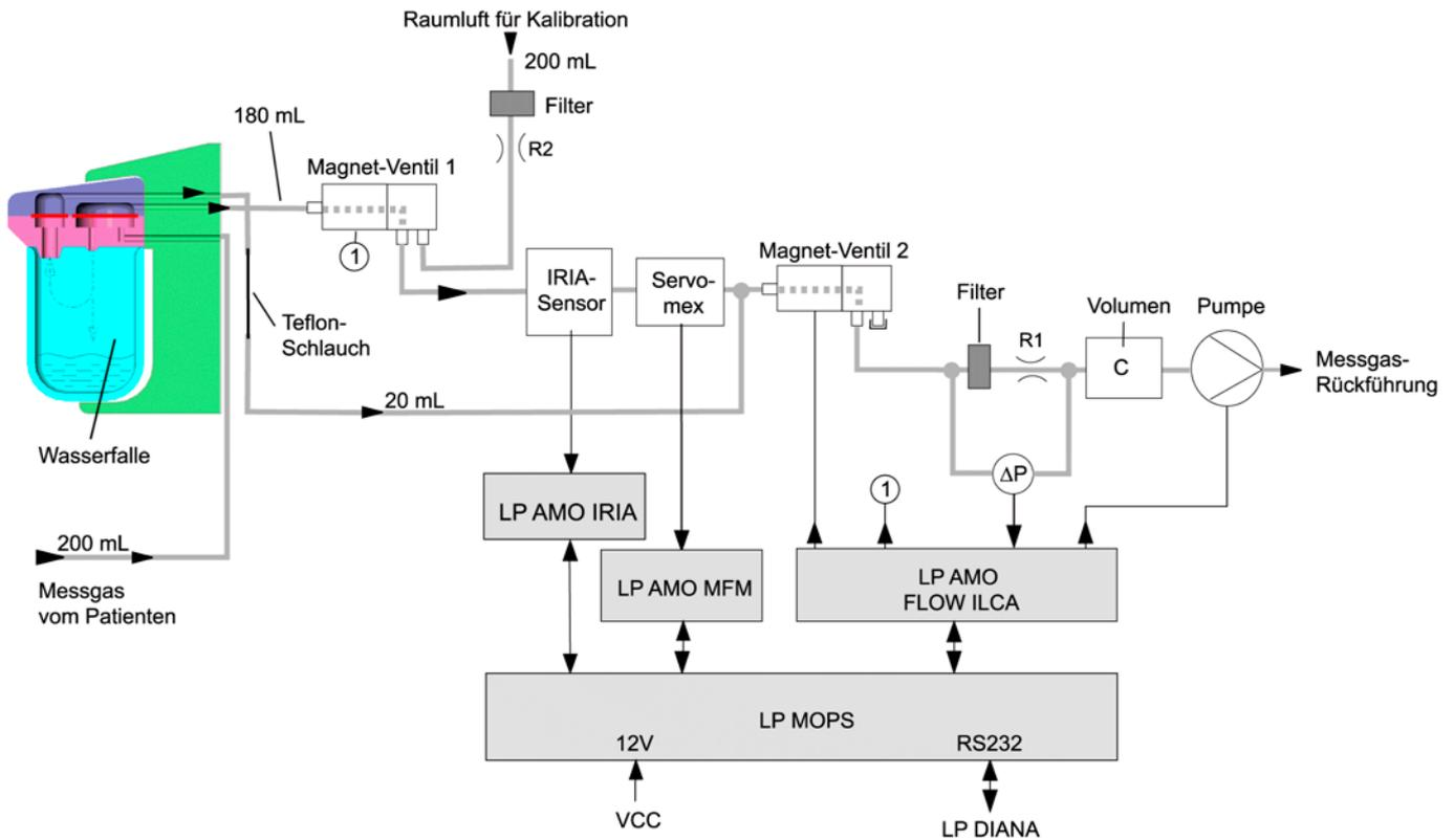
Figure 20 PGA block diagram (example GMZ)
