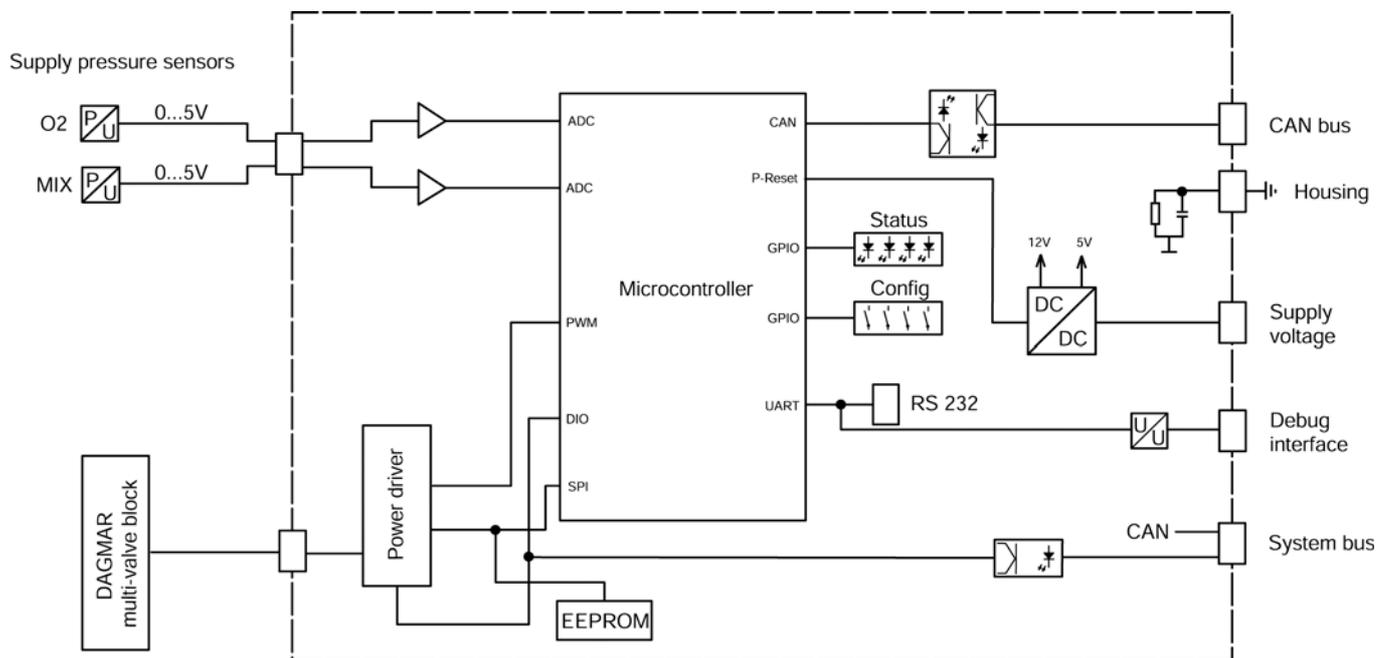
Figure 12 Block diagram of the DAGMAR PCB
