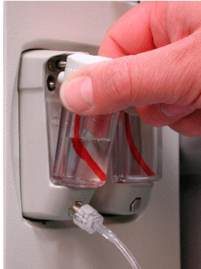
**Figure 1** Removing the water trap
