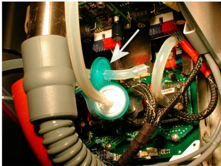
**Figure 13** Sampling-gas return-line filter
