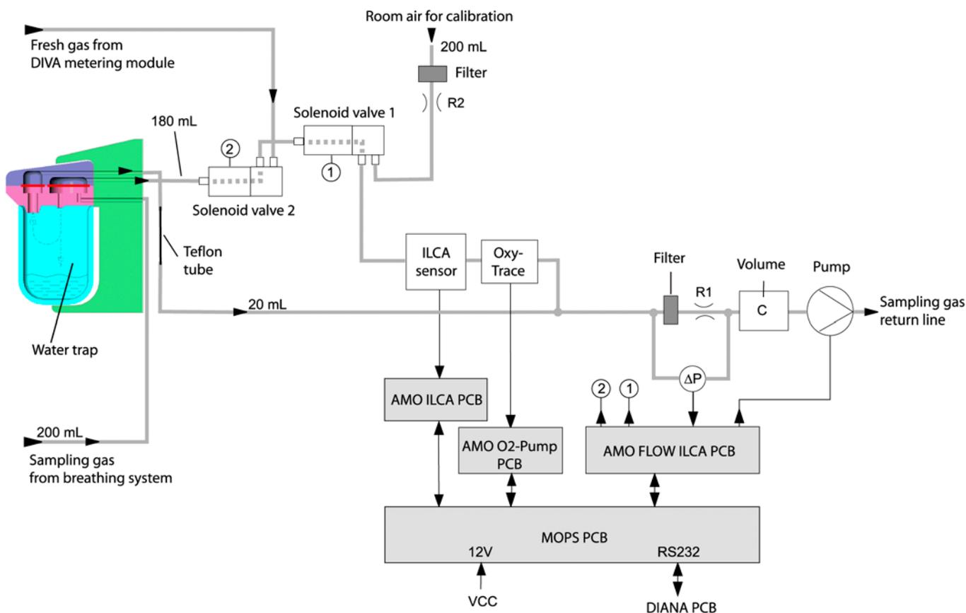
**Figure 29** Connection diagram
