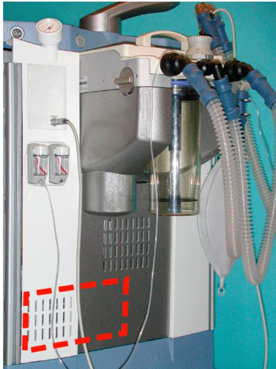
**Figure 4** Fitting location of the power supply unit in the Zeus
