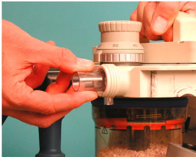
**Figure 12** Removing the flow sensor
