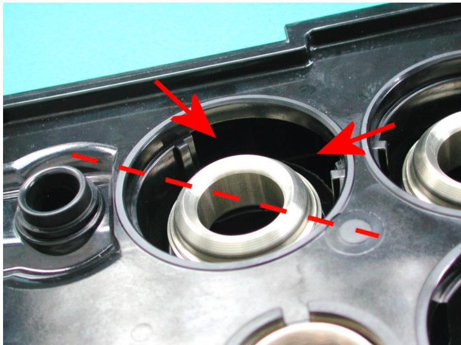
**Figure 10** Diaphragm mount location hole
