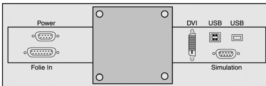
Figure 43 Monitor connections
