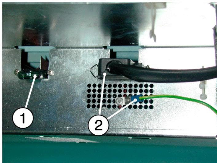
Figure 24 Fuse (1) and connector (2) on drawer unit
