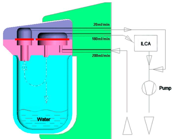
**Figure 35** Principle of operation of the Dräger water trap
