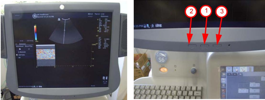
**Figure 6-89 17 inch IPS-Pro Type LCD Monitor Adjustment buttons**
