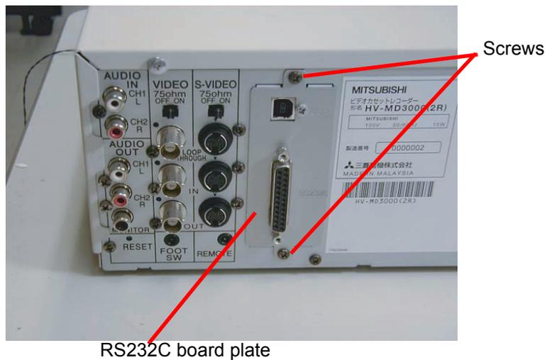
Figure 6-109 Opening Board Plate
