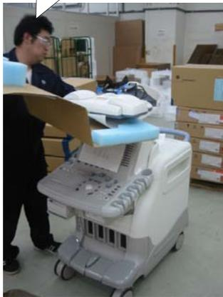
Turn over the LCD monitor, and place the sleeve to the location above. Make sure LCD arm is locked.
