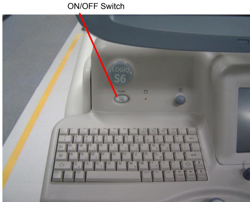
**Figure 4-12 Power On/Off Standby Switch Location**
