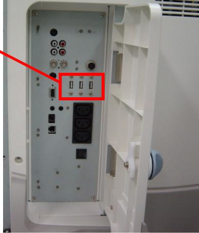
**Figure 6-80** Inserting the Service Dongle
