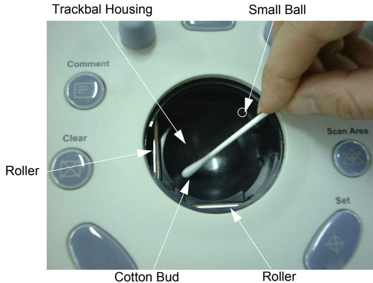
**Figure 6-99 Cleaning TrackBall and Housing**
